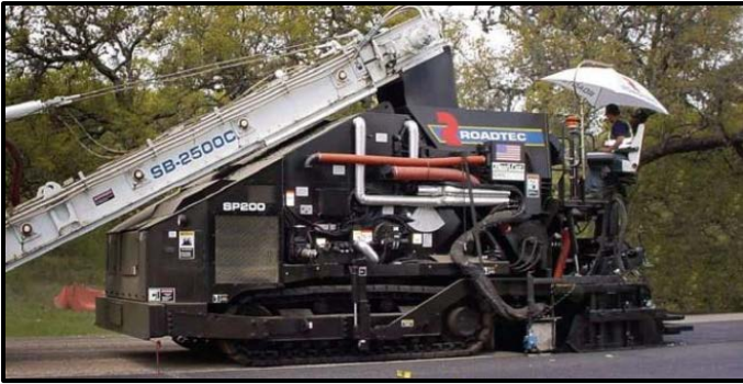
Figure 6. Spray paver used in asphalt overlay construction (Al-Qadi et al. 2012).
