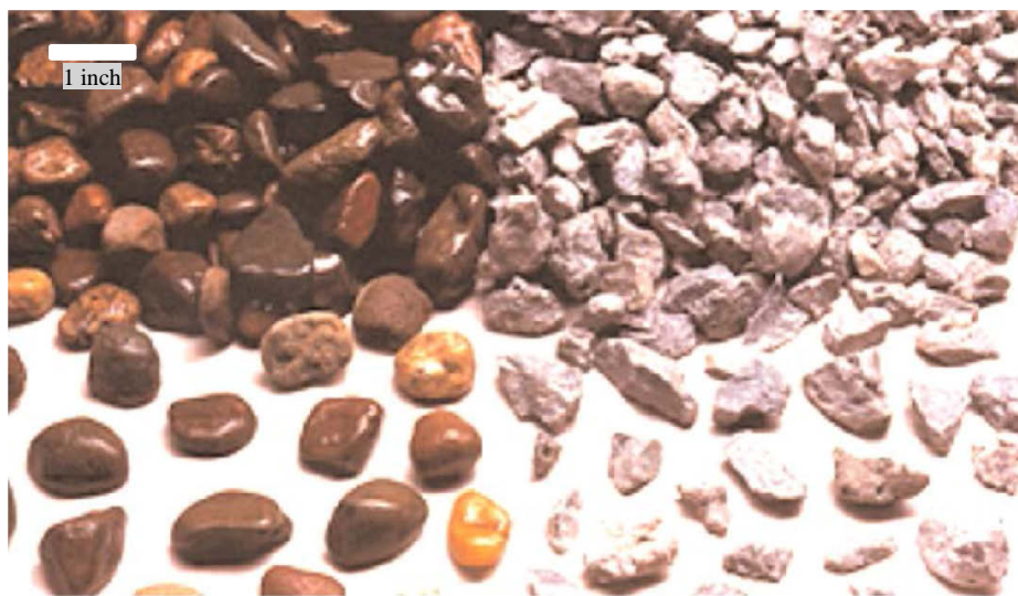
Figure 3-2. Coarse aggregates: rounded gravel (left) and crushed stone (right) (Kosmatka and Wilson 2011).
