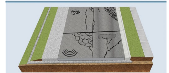
Poor - Frequent surface distresses such as potholes, block cracking, or thermal cracking plus alligator cracking, rutting, shoving, slippage, stripping, and raveling.
