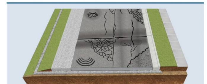
Deteriorated - Significant surface and structural distresses, including potholes, block cracking, or thermal cracking plus alligator cracking, rutting, shoving, slippage, stripping, and raveling.
