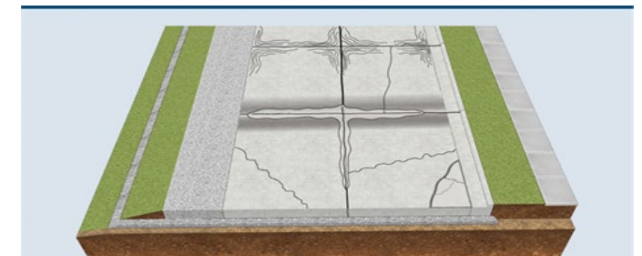
Deteriorated – Significant surface deterioration and structural distresses, including joint deterioration from freeze-thaw damage or material-related distress at 50% or more of the joints.
