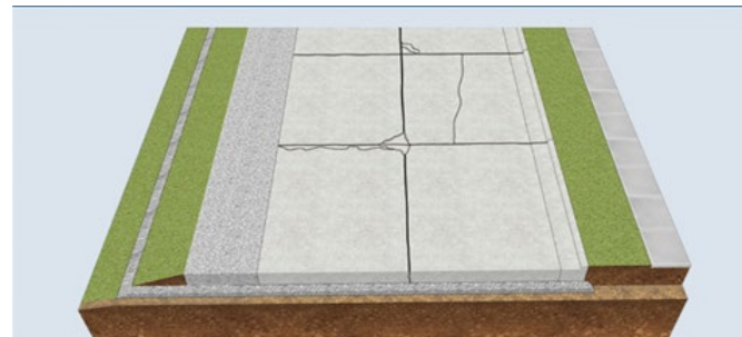
Fair – Structurally sound with minor surface distresses such as random cracking, periodic partial-depth joint spalling, and shadowing.
