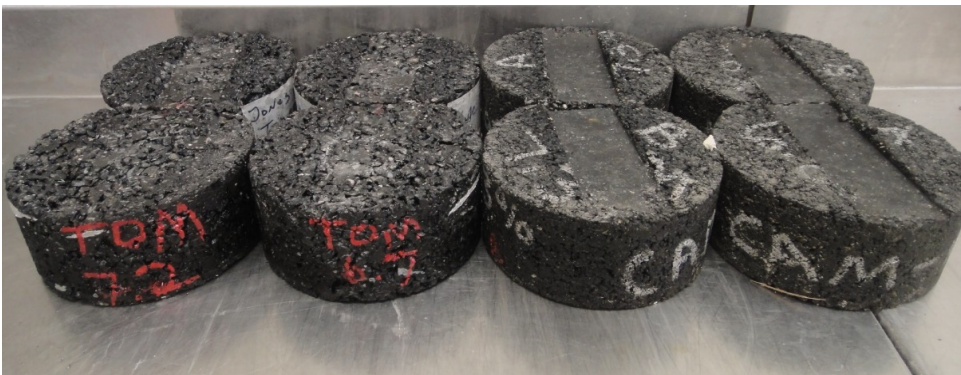
Figure 9. TOM and CAM samples after HWTT. Source: Tom Scullion, TTI
