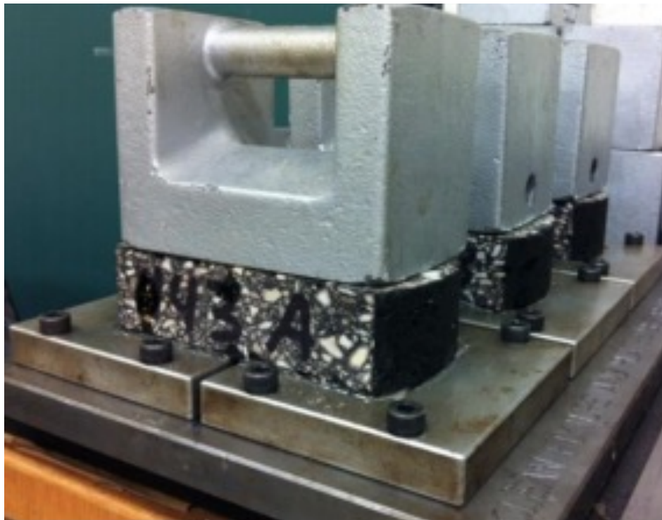
Figure 12. Weighted specimens after being epoxied to blocks. Source: TxDOT 2017
