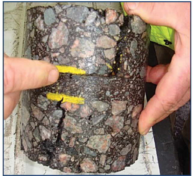
Figure 13. Crack jumping over a crack attenuating layer with a stiff surface mix. (Source: Bennert 2021)
