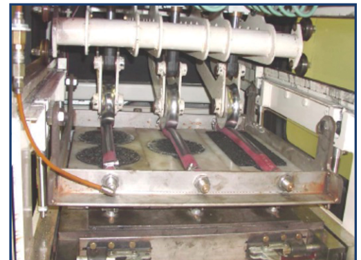
Figure 17. Asphalt Pavement Analyzer. (Source: Dr. Tom Bennert)
