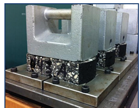
Figure 20. Weighted specimens after being epoxied to blocks. (Source: TxDOT 2017)
