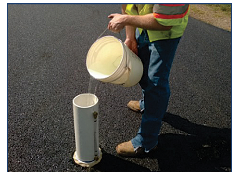
Figure 26. Water flow test. (Source: TxDOT 2015)
