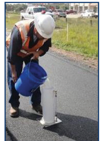
Figure 16. Texas water flow test. (Source: TxDOT)
