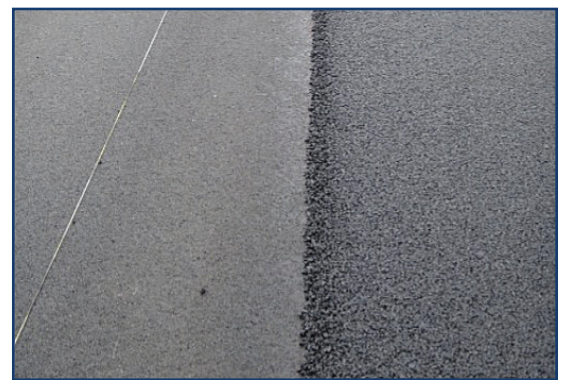
Figure 2. Surface texture of TOM-F (left) and TOM-C (right). (Source: Texas A&M Transportation Institute)
