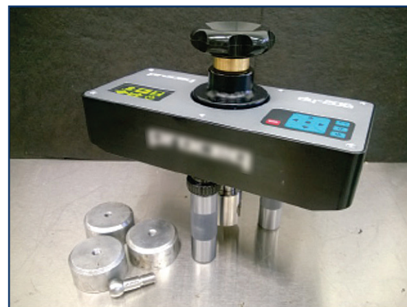
Figure 12. Pull-off bond strength tester. (Source: TxDOT)
