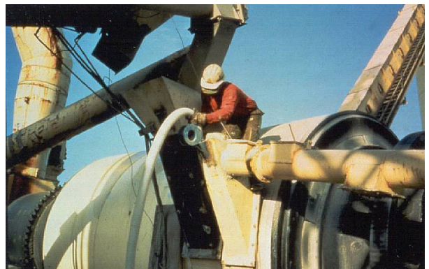
Figure 7: Fiber injection point in a double-barrel asphalt plant. (Source: Krendl Machine Co.)
