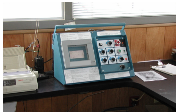
Figure 6: Rate controller for accurately proportioning fiber. (Source: Krendl Machine Co.)
