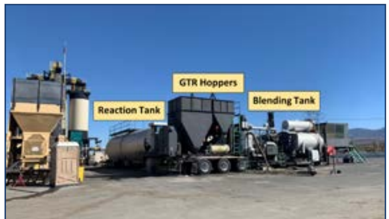
Figure 5. Asphalt rubber blending unit.
