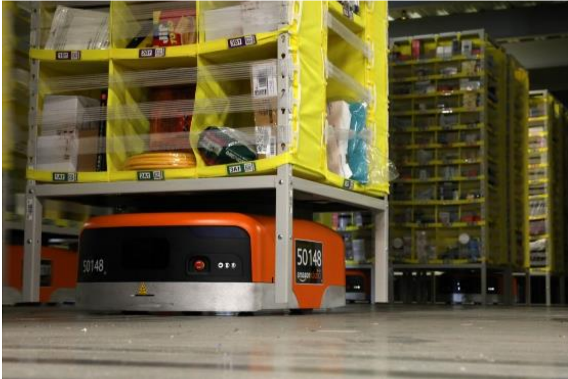
Figure 7. Robot Lifting a Pod in the MSP 1 Amazon Fulfillment Center
