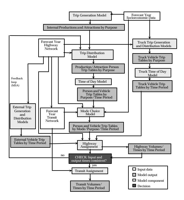
Fig. 1: Structure of the SEMCOG Model
