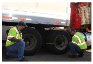
Figure 2 – Measuring Test Truck Axle Spacing
