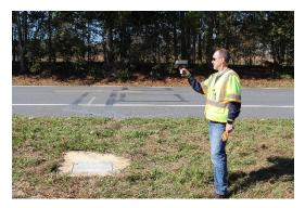
Figure 12 – Collecting Test Truck Speed
