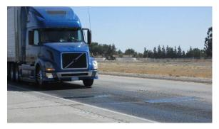
Figure 1 – Calibration Test Truck Approaching WIM Scale
