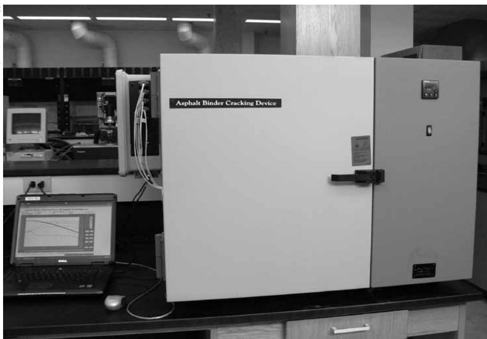
Innovations funded by FHWA's Technology Partnerships Program include the Asphalt Binder Cracking Device, which simulates pavement cracking to help agencies predict and prevent asphalt failure caused by cracking at low temperatures.
