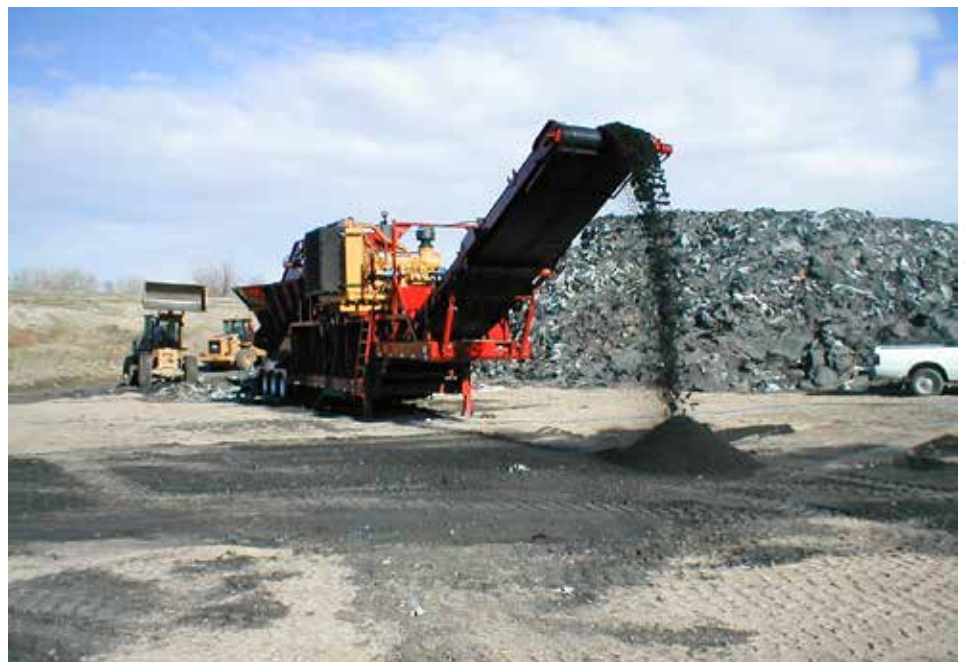
Recycled shingles can be used in hot-mix asphalt.
