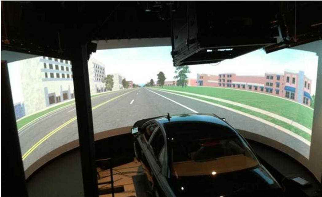
**Figure 4-2: Photograph. Driving simulator used for the study.**
