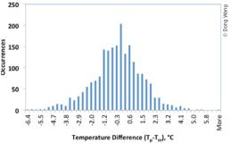
Histogram of asphalt pavement subsurface temperature difference
