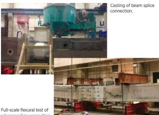
Full-scale flexural test of a beam splice connection made of UHPC. *IMPACT:* This research allows for the development and implementation of a quality control test method for UHPC in a production environment. Broader use of UHPC could lead to more durable and longer lasting highway structures, reducing the cost and risks associated with reconstruction.
