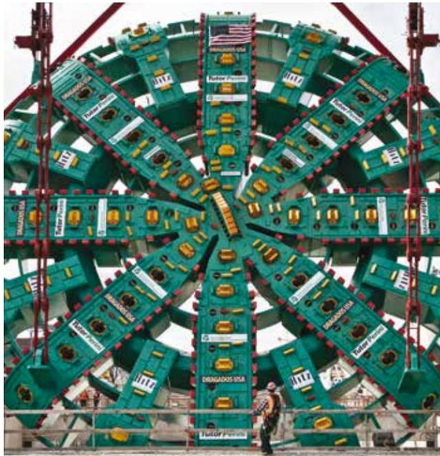
Figure 2. Photo. Tunnel boring machine nicknamed “Bertha” being lowered into position to begin 2-mile-long tunnel project in Seattle, WA, July 2013. ©Washington State Department of Transportation.
