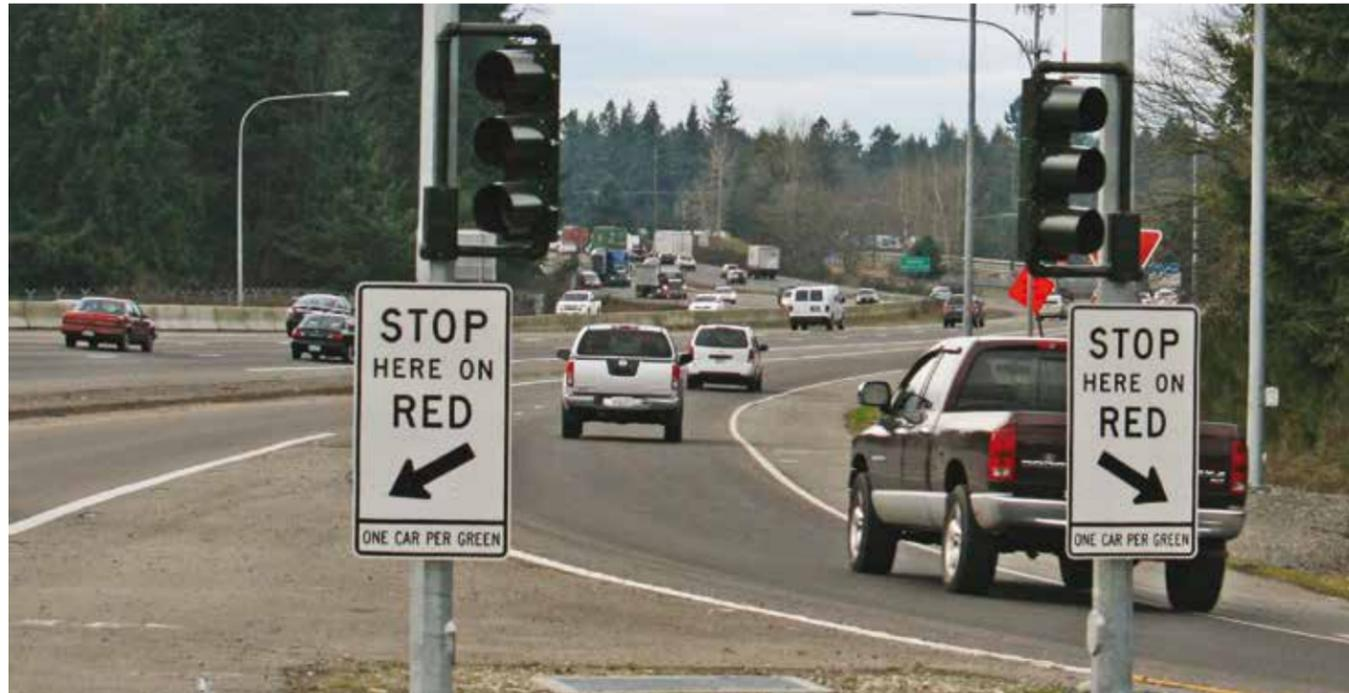
**Figure 1. Photo. Ramp metering system uses traffic signals to regulate the flow of vehicles entering a freeway from on-ramps. ©Washington State Department of Transportation.**
