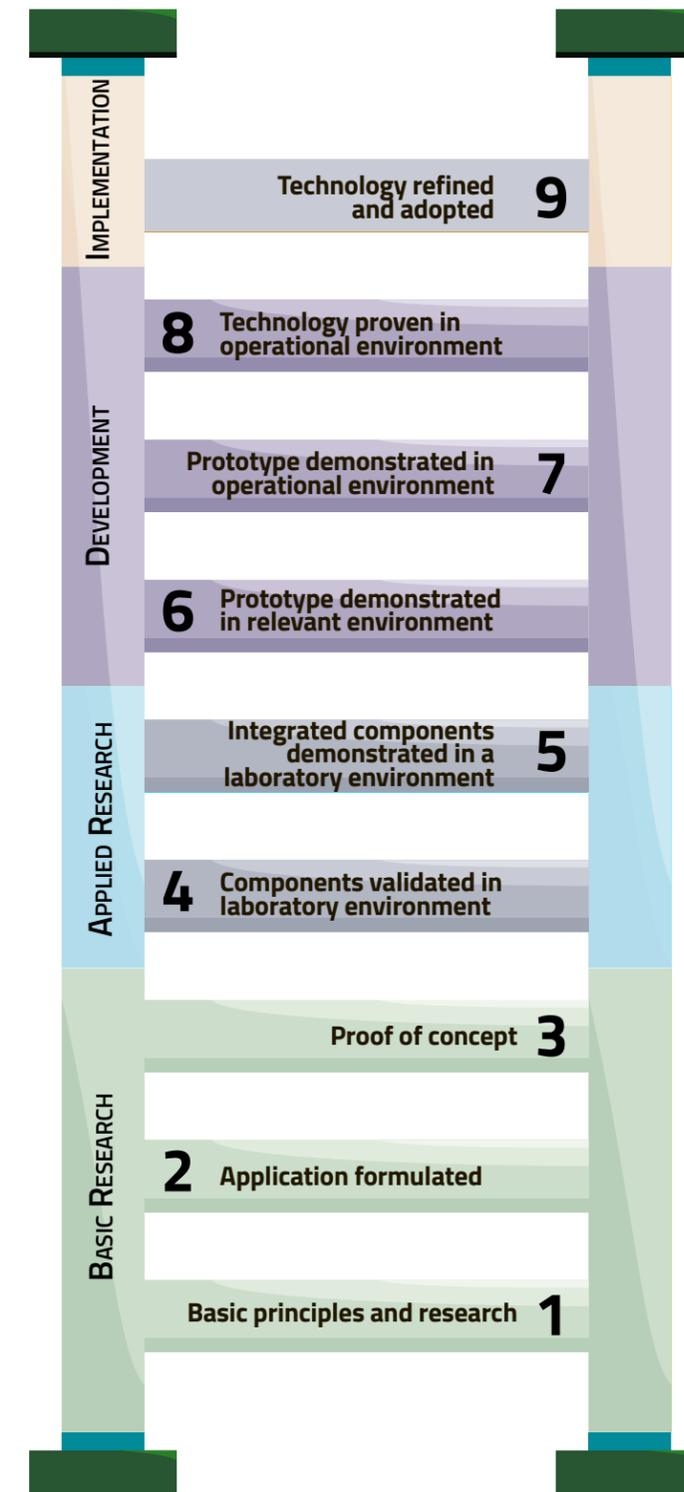
Figure 8. Chart. TRL Scale Levels Ladder Graphic.
