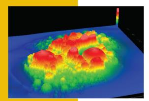
Photo credit: © Henry Samueli School of Engineering and Applied Science, University of California, Los Angeles. A three-dimensional image acquired using vertical scanning interferometry that shows a cluster of fly ash particles. The color gradient from blue to red indicates the height relative to the adjacent surface (low to high).
