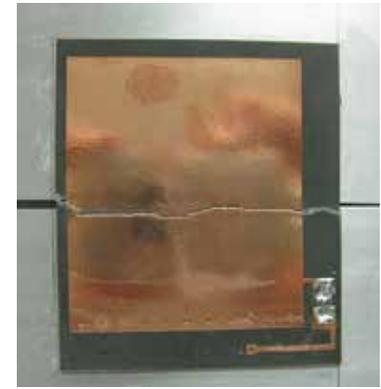
Antenna sensor tracking crack propagation.
