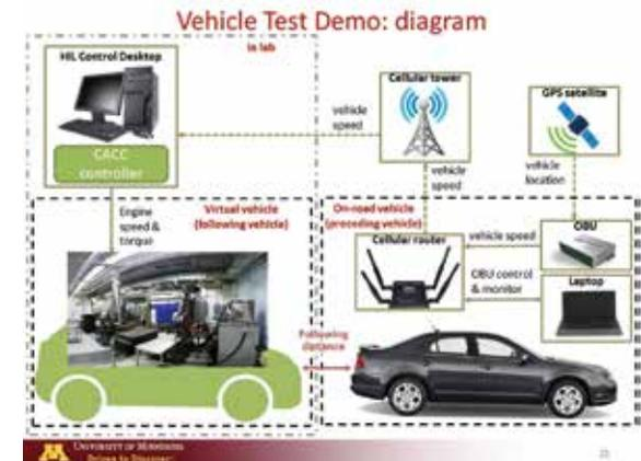
The in-lab testbed ensures that the engine has the same load as the engine running in the field-test CAV with an onboard unit (OBU) under various operation scenarios. The engine’s emission and fuel consumption are precisely measured by the lab’s powerful devices. Source: FHWA.
