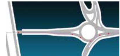
Actual road data (red points) used in response comparisons for a roundabout scenario. Source: FHWA.
