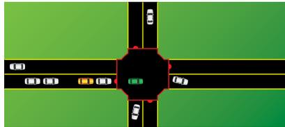
An AIM simulation, which shows virtual and real vehicles at an intersection. White vehicles have a reservation to enter the intersection; yellow vehicles do not. The green vehicle is a proxy, representing the real-world location of the autonomous vehicle. Source: FHWA.
