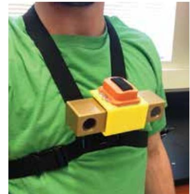
A chest-mounted stereo camera and inertial measurement unit form part of Auburn University's pedestrian navigation system. © Auburn University.
