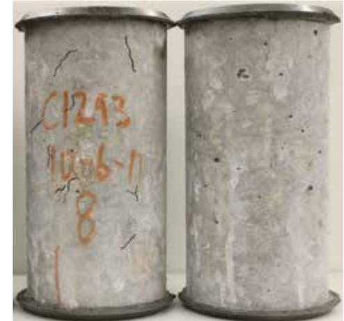
Two concrete samples using equivalently reactive aggregate. Left, ASR-damaged concrete with cracks marked; right, crack-resistant HyFRC for concrete strength and stiffness retention. © 2013 Claudia Ostertag.
