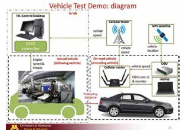
The in-lab testbed ensures that the engine has the same load as the engine running in the field-test CAV with an onboard unit (OBU) under various operation scenarios. The engine’s emission and fuel consumption are precisely measured by the lab’s powerful devices. Source: FHWA.
