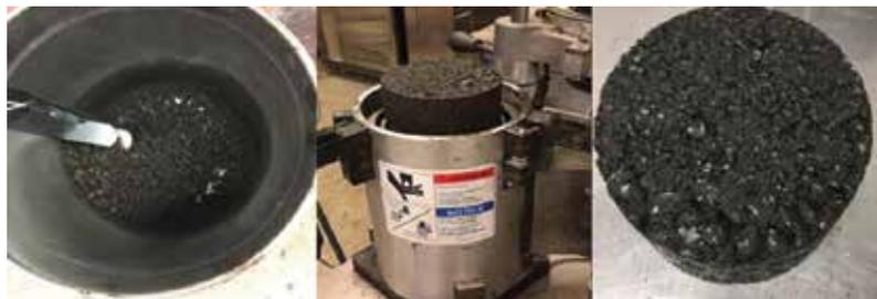
Researchers created a rotary reactor to simulate the production of the hot-mix bio-binder through mixing aggregates with bioasphalt. © 2017 Department of Civil and Environmental Engineering, Washington State University.
