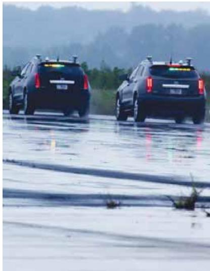
FHWA test vehicles simulate a "platoon" of vehicles using cooperative adaptive cruise control.
