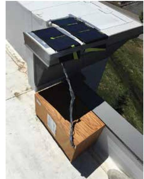
The project's control system collects, processes, and transmits the real-time water quality data provided by the in situ sensors. © Qing Yang, Montana State University.
