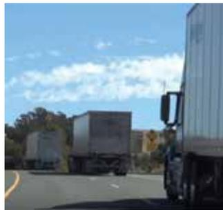
Three Class 8 trucks equipped with CACC during field test. © University of California, Berkeley.
