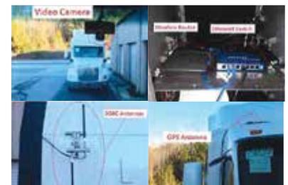
CACC incorporates video cameras, a DSRC system for inter-vehicle data exchange, and GPS. © n.d. Auburn University, College of Engineering.
