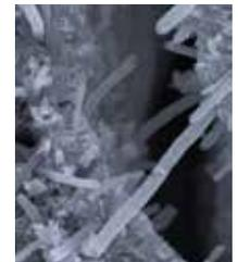
Carbon nanofibers spanning nano/micro crack in a cementitious composite. Source: FHWA.
