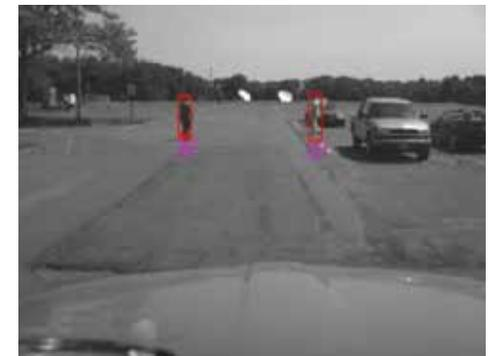
Visual output of the pedestrian-detection system as it recognizes crossing pedestrians. Source: FHWA.
