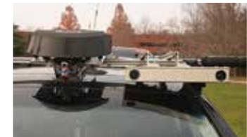
Camera and LIDAR equipment mounted on the roof of the test vehicle. Source: FHWA.
