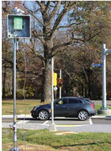
Battery-powered AVTS radar housed in weatherproof case on adjustable-height tower. Source: FHWA.
