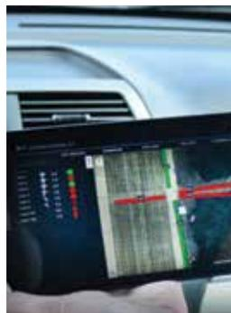
CONVAS incorporates data from actual connected vehicles and traffic signals (left) into a simulation that displays the interaction among the vehicles and infrastructure. © Texas A&M Transportation Institute.
