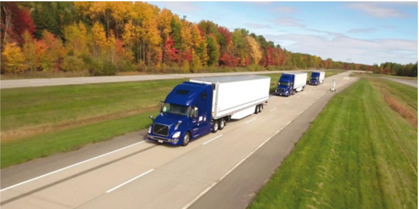
**Figure 1.** University of California-Berkeley researchers built a cooperative adaptive cruise control system into a platoon of three long-haul trucks to test the technology's potential to improve traffic flow, save fuel, and curtail emissions.
