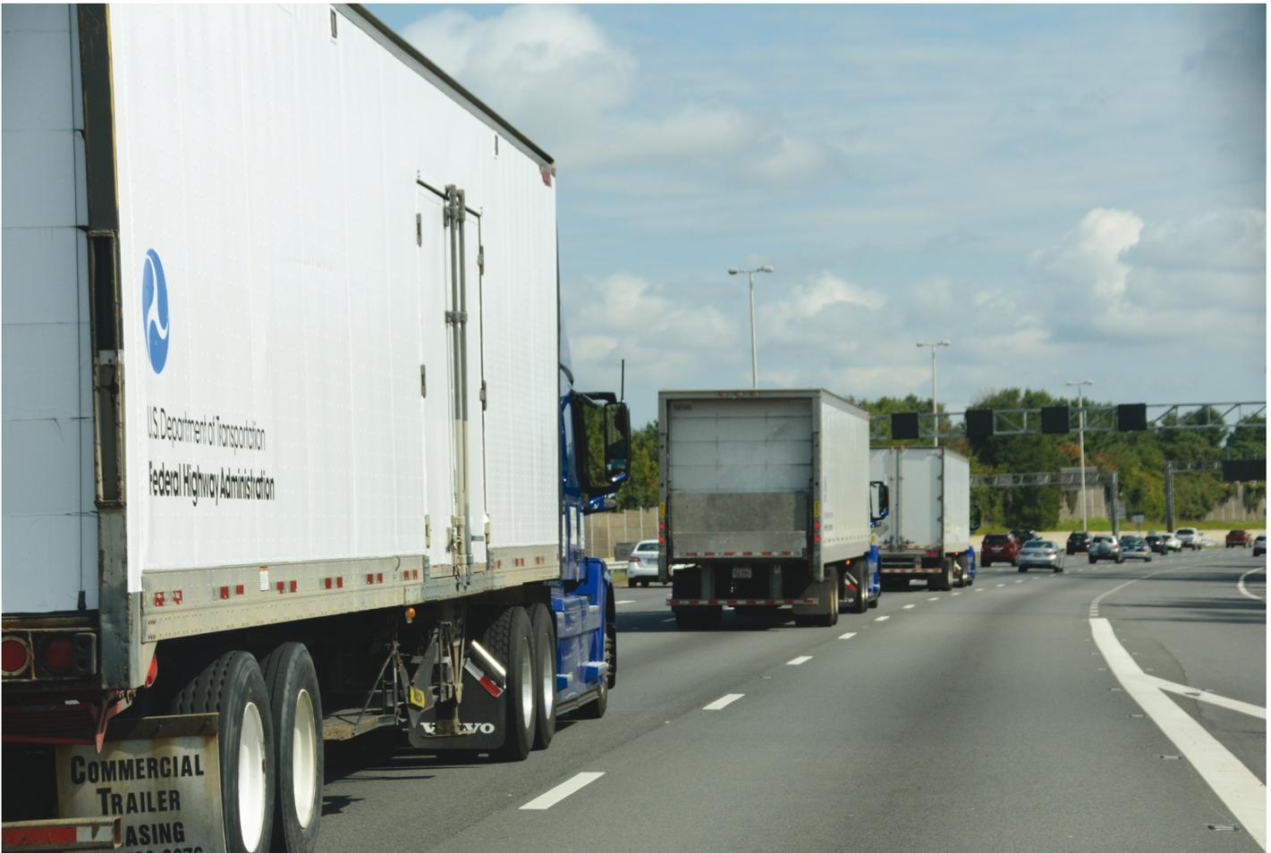
Figure 7. Researchers demonstrated the truck-platooning system on Interstate 66 in Northern Virginia. Source: FHWA.
