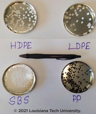
This photo shows different processed industrial waste plastic (HDPE, LDPE, SBS, and PP) used in this study.
