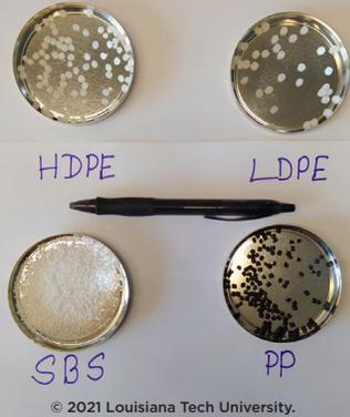
This photo shows different processed industrial waste plastic (HDPE, LDPE, SBS, and PP) used in this study.
