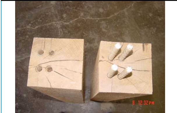
Figure 1. GFRP rebars embedded in a wood beam.
