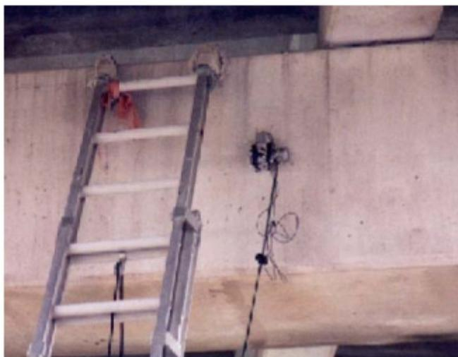
Figure 36. Photo. Biaxial accelerometer mount with vertical and horizontal accelerometers, west pier, Woodville Road Bridge.
