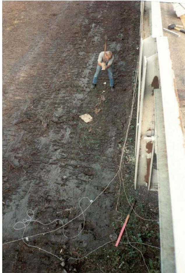
Figure 7. Photo. SASW tests at bent 12, structure 4, Trinity River Relief Bridge.
