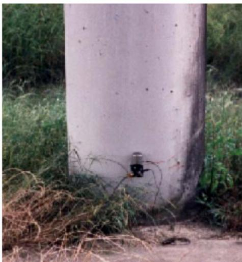
Figure 37. Photo. Vertical accelerometer at base of column of west pier, Woodville Road Bridge.
