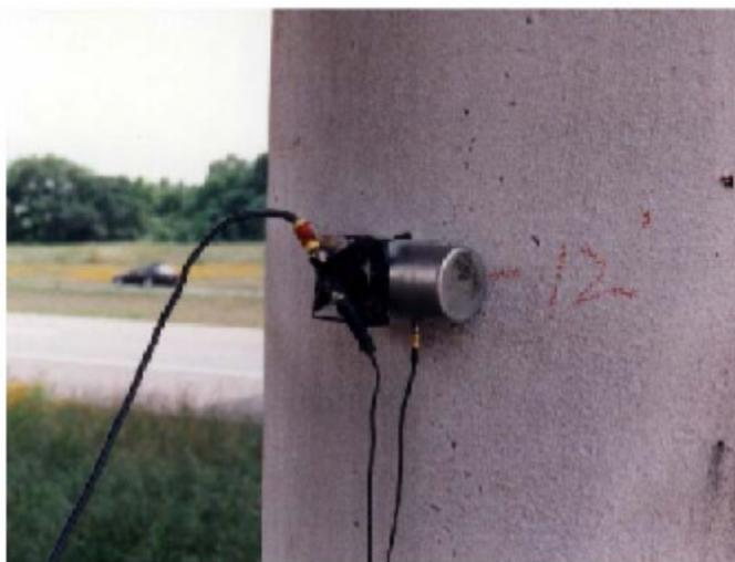
Figure 38. Photo. Horizontal accelerometer on side of column of west pier, Woodville Road Bridge.
