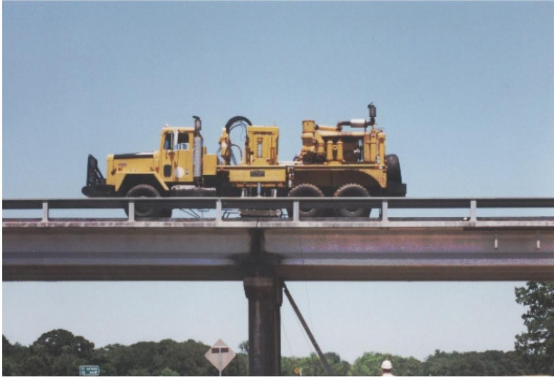
Figure 10. Photo. Vibroseis truck over Woodville Road Bridge pier.
