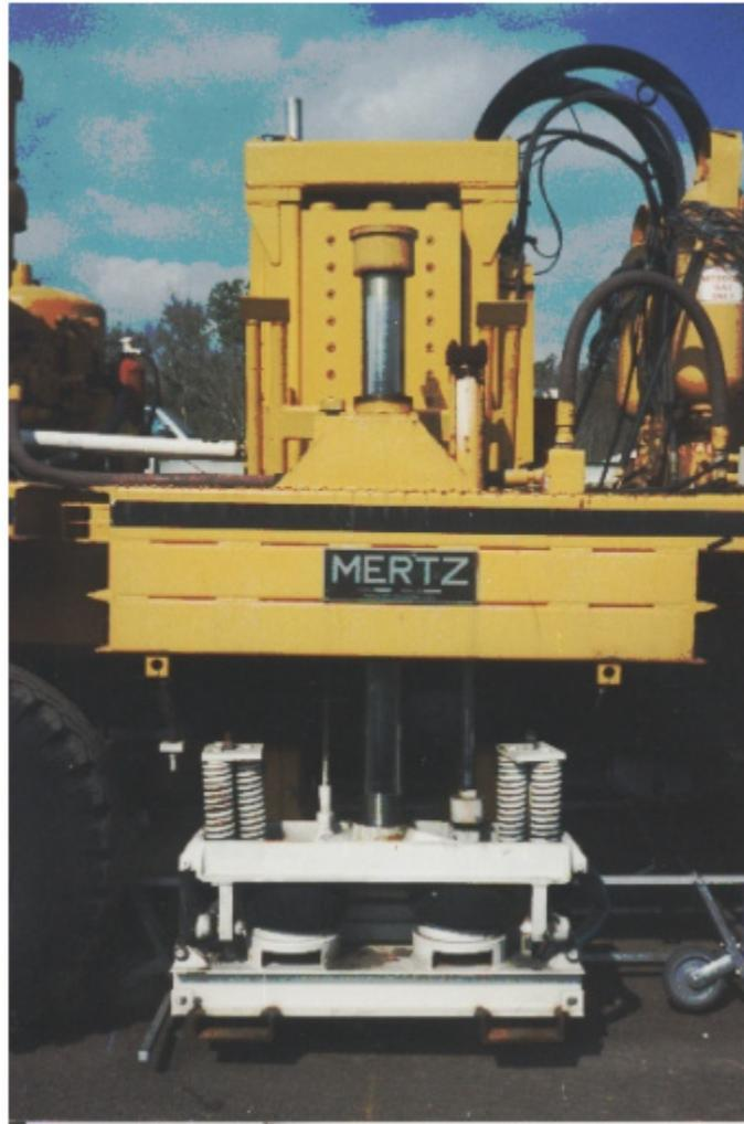
Figure 11. Photo. Vertical vibrator mechanism of Vibroseis truck.
