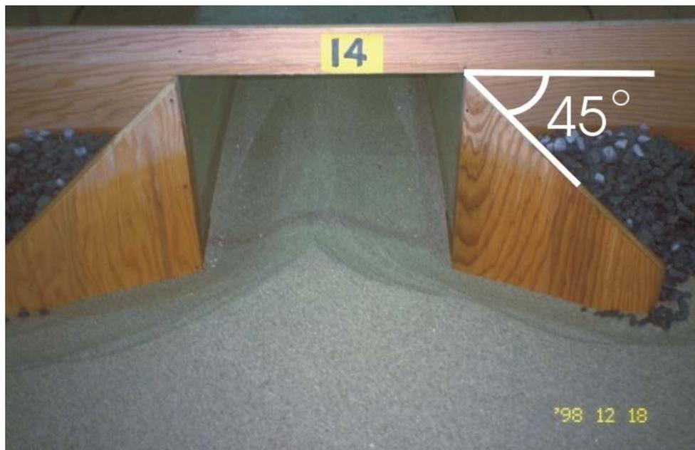
**Figure 5. Rectangular model with wingwalls.**
