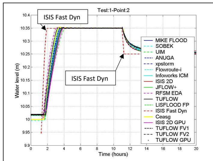
Figure 2-8 Test Point 2 – Water Level versus Time from Report SC120002 (2013)
