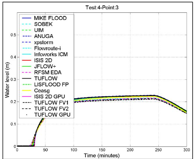
Figure 5-15 Test Point 3 – Water Level versus Time from Report SC120002 (2013)
