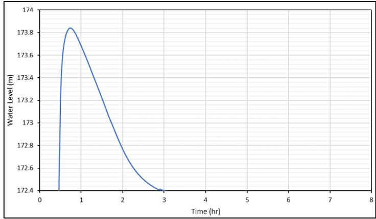
Figure 6-29 Test Point 6 – Water Level versus Time from SRH-2D
