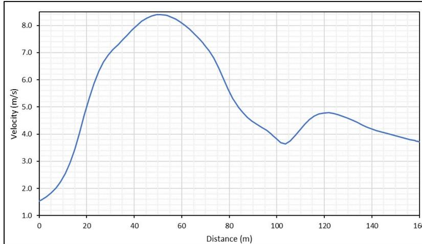
Figure 7-65 Test 6B Maximum Velocity Magnitude Along XS 1 from SRH-2D
