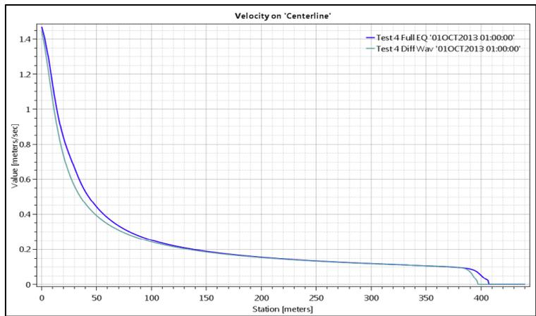
Figure 5-39 Cross Section from Inflow to Point 5 – Velocity versus Distance at 1 Hour from RD-51 (2018)
