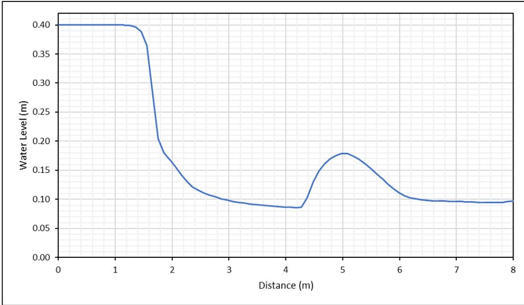
Figure 7-23 Test 6A Maximum Water Surface Elevation Along XS 1 from SRH-2D
