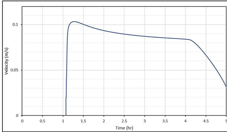
Figure 5-32 Test Point 6 – Velocity versus Time from SRH-2D
