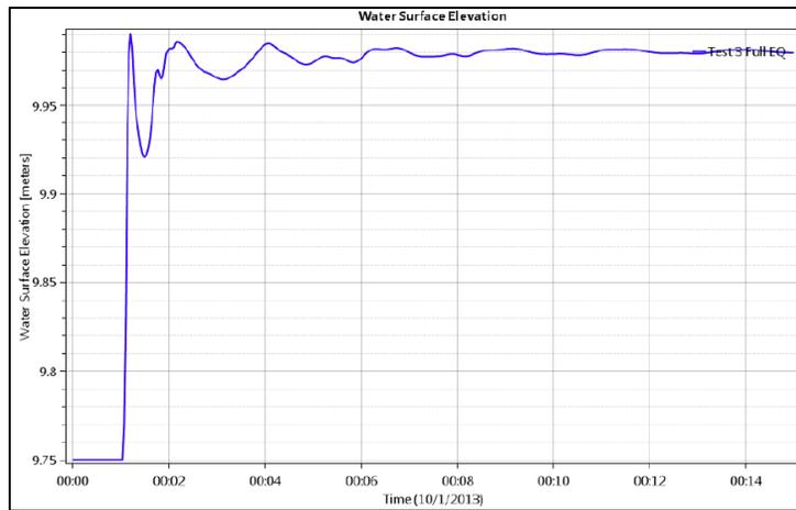
Figure 4-4 Test Point 1 – Water Level versus Time from RD-51 (2018)
