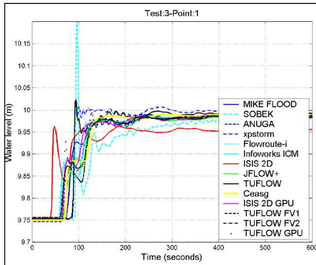
Figure 4-5 Test Point 1 – Water Level versus Time from Report SC120002 (2013)
