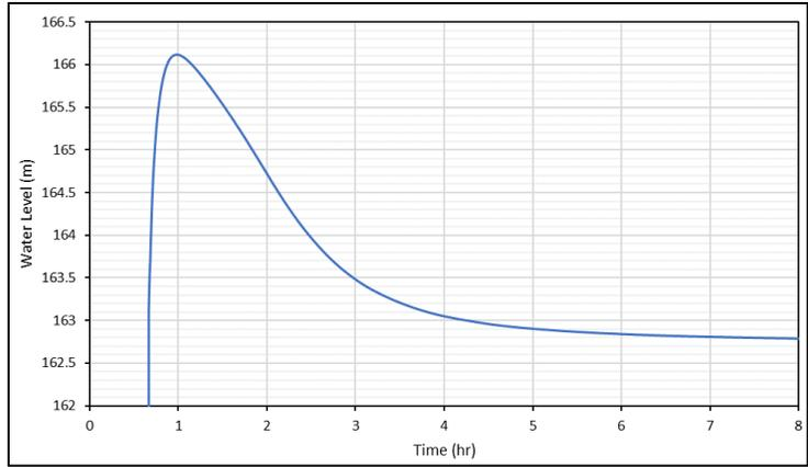
Figure 6-9 Test Point 2 – Water Level versus Time from SRH-2D
