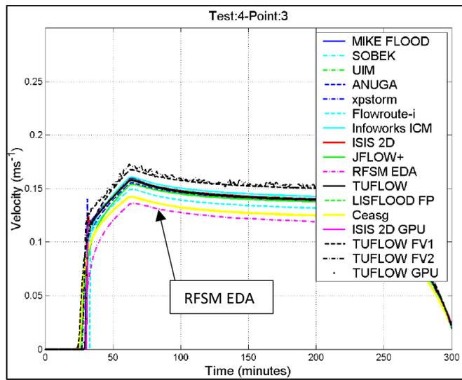
Figure 5-18 Test Point 3 – Velocity versus Time from Report SC120002 (2013)
