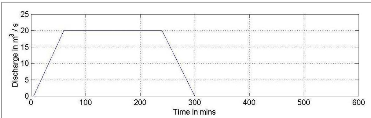
Figure 5-2 Inflow hydrograph used as upstream boundary condition.
