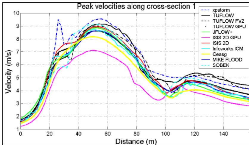
Figure 7-67 Test 6B Maximum Velocity Magnitude Along XS 1 from Report SC120002 (2013)
