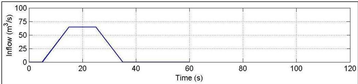
Figure 4-2 Inflow hydrograph used as upstream boundary condition.
