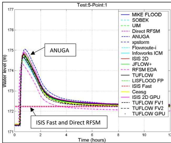
Figure 6-5 Test Point 1 – Water Level versus Time from Report SC120002 (2013)
