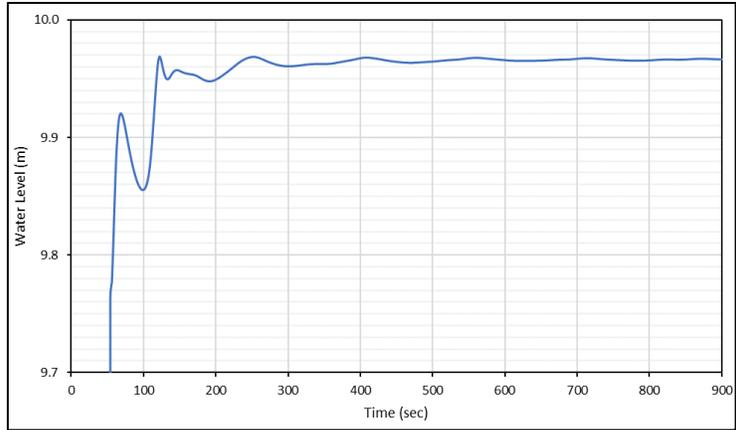
Figure 4-3 Test Point 1 – Water Level versus Time from SRH-2D
