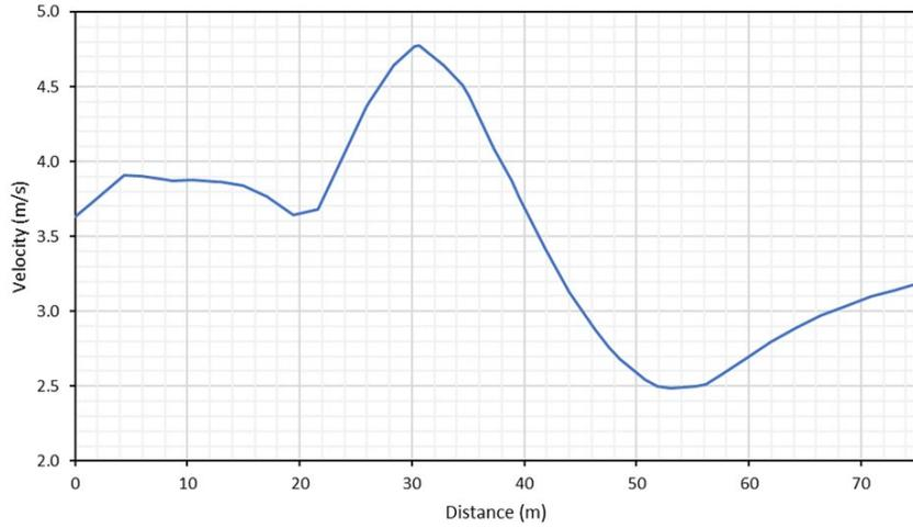
Figure 7-71 Test 6B Maximum Velocity Magnitude Along XS 2 from SRH-2D
