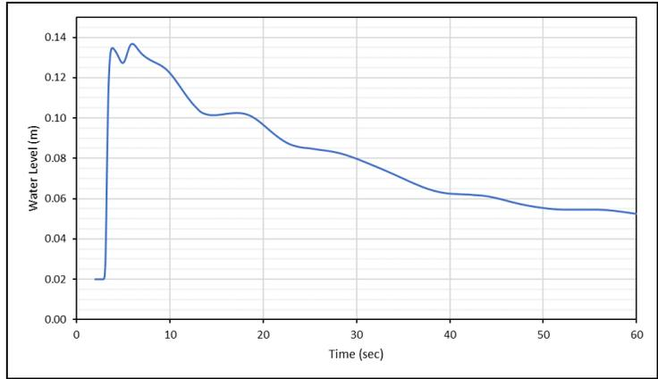
Figure 7-8 Test Point G3 – Water Level versus Time from SRH-2D
