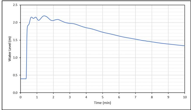
Figure 7-47 Test Point G5 – Water Level versus Time from SRH-2D
