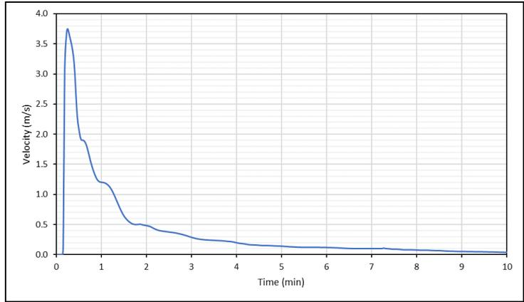
Figure 7-29 Test Point G1 – Velocity versus Time from SRH-2D
