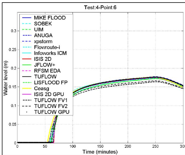
Figure 5-31 Test Point 6 – Water Level versus Time from Report SC120002 (2013)
