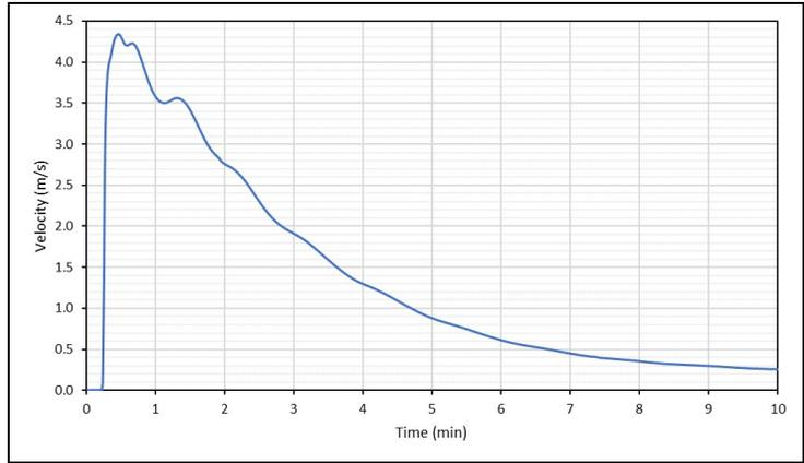
Figure 7-44 Test Point G4 – Velocity versus Time from SRH-2D
