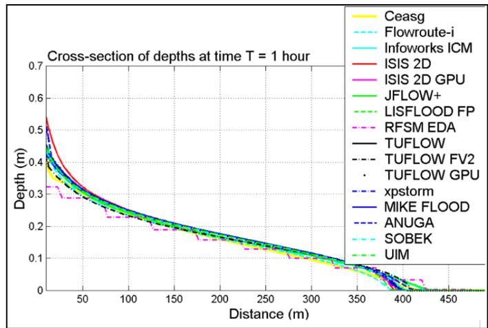
Figure 5-37 Cross Section from Inflow to Point 5 – Water Level versus Distance at 1 Hour from Report SC120002 (2013)
