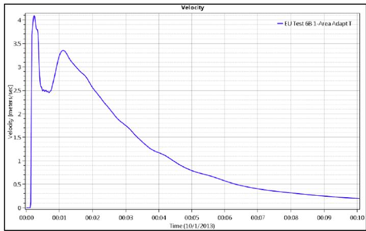
Figure 7-35 Test Point G2 – Velocity versus Time from RD-51 (2018)
