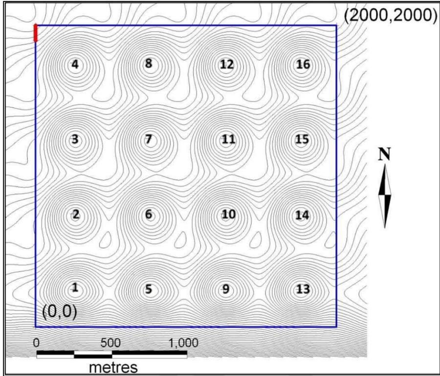
Figure 3-1 Map of the DEM showing the location of the upstream boundary condition (red line), ground elevation contour lines every 0.05 meters, and output point locations (numbers).
