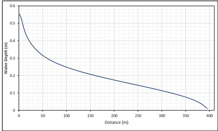
Figure 5-35 Cross Section from Inflow to Point 5 – Water Level versus Distance at 1 Hour from SRH-2D
