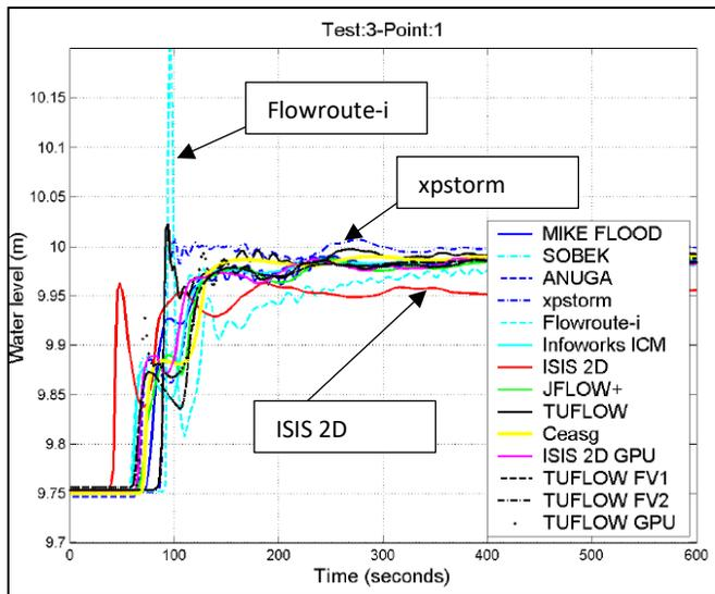
Figure 4-5 Test Point 1 – Water Level versus Time from Report SC120002 (2013)
