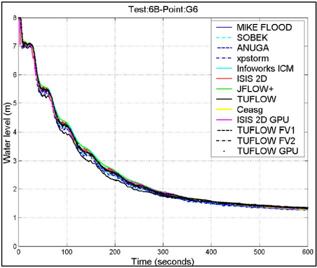
Figure 7-54 Test Point G6 – Water Level versus Time from Report SC120002 (2013)
