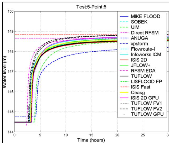
Figure 6-26 Test Point 5 – Water Level versus Time from Report SC120002 (2013)
