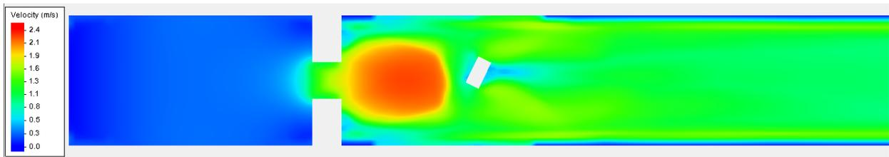
Figure 7-22 Test 6A Maximum Velocity Magnitude (meters per second) from SRH-2D
