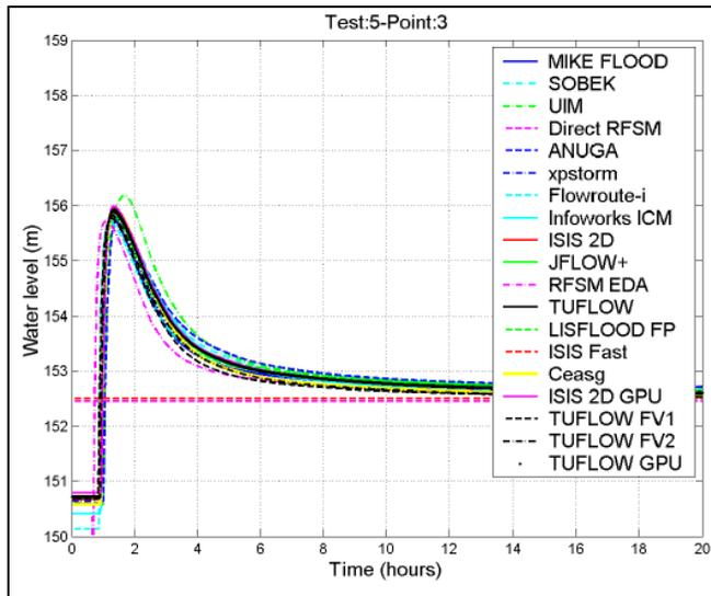
Figure 6-15 Test Point 3 – Water Level versus Time from Report SC120002 (2013)
