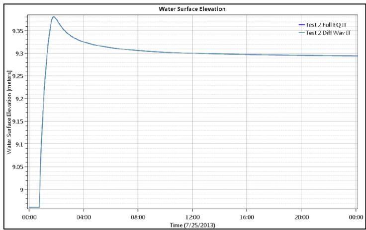
Figure 3-16 Test Point 8 – Water Level versus Time from RD-51 (2018)
