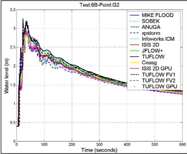
Figure 7-33 Test Point G2 – Water Level versus Time from Report SC120002 (2013)
