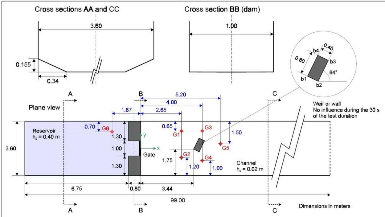
Figure 7-1 Setup for Benchmark Test 6A adapted from Soares-Fraza and Zech (2002).
