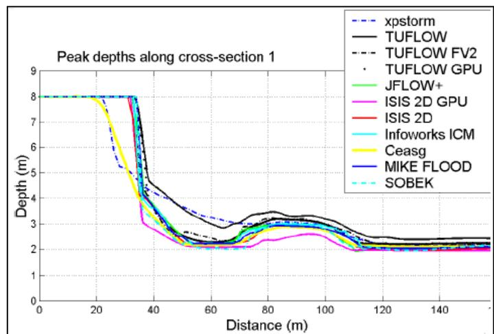
Figure 7-64 Test 6B Maximum Water Surface Elevation Along XS 1 from Report SC120002 (2013)
