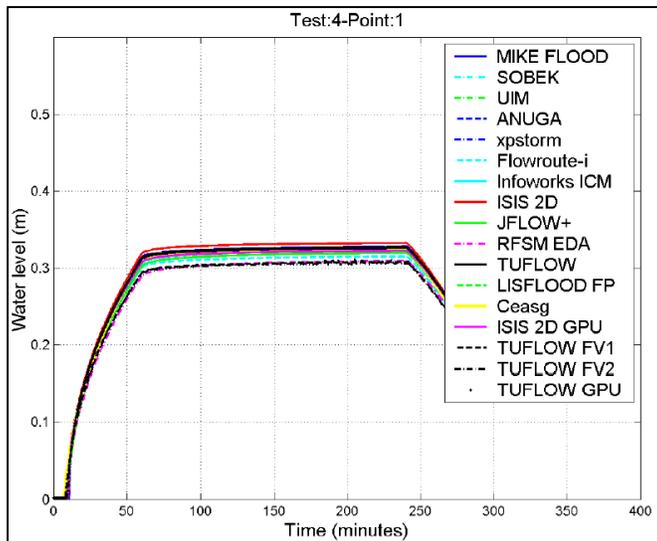
Figure 5-5 Test Point 1 – Water Level versus Time from Report SC120002 (2013)
