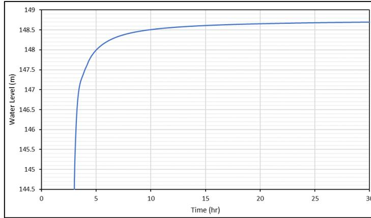
Figure 6-24 Test Point 5 – Water Level versus Time from SRH-2D
