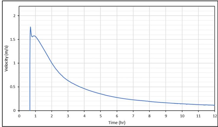
Figure 6-11 Test Point 2 – Velocity versus Time from SRH-2D
