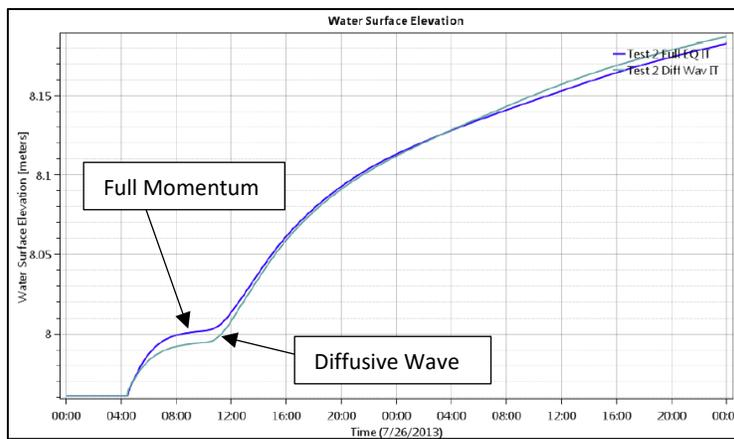
Figure 3-25 Test Point 5 – Water Level versus Time from RD-51 (2018)
