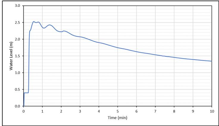
Figure 7-37 Test Point G3 – Water Level versus Time from SRH-2D
