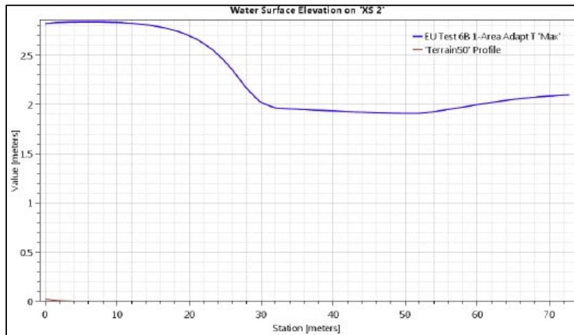
Figure 7-69 Test 6B Maximum Water Surface Elevation Along XS 2 from RD-51 (2018)
