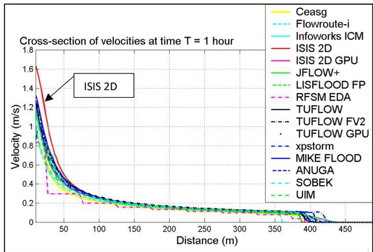
Figure 5-40 Cross Section from Inflow to Point 5 – Velocity versus Distance at 1 Hour from Report SC120002 (2013)
