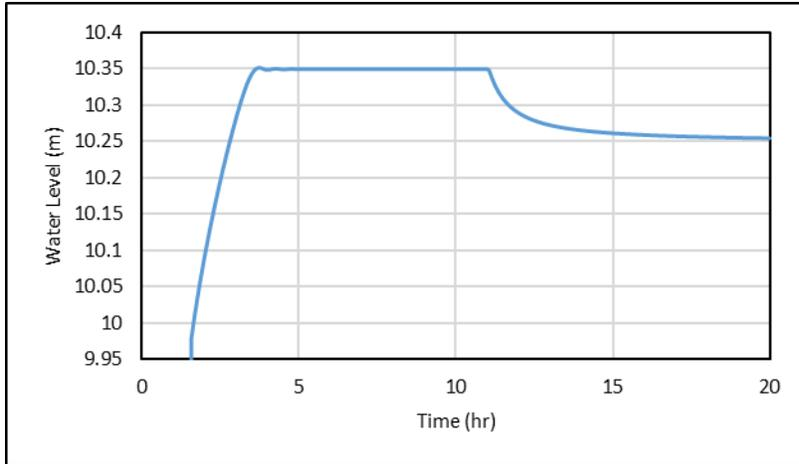
Figure 2-6 Test Point 2 – Water Level versus Time from SRH-2D
