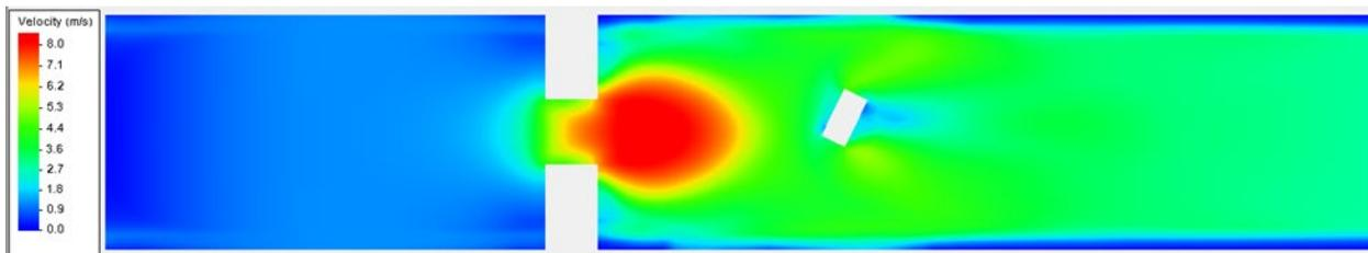
Figure 7-59 Test 6B Maximum Velocity Magnitude (meters per second) from SRH-2D
