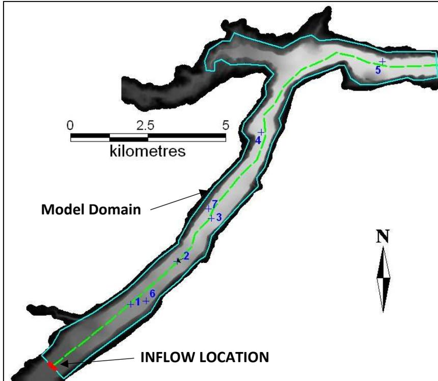
Figure 6-1 Plan view of DEM used in Benchmark Test 5 including output point locations. The red line indicates the location of the boundary condition, and the cyan polygon represents the extents of the model's domain.
