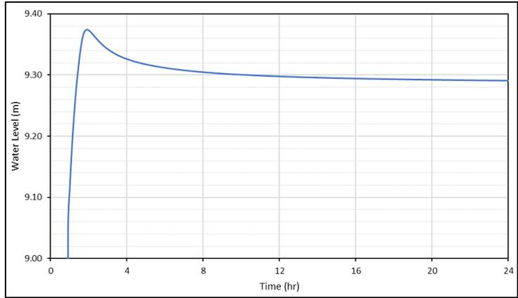
Figure 3-15 Test Point 8 – Water Level versus Time from SRH-2D
