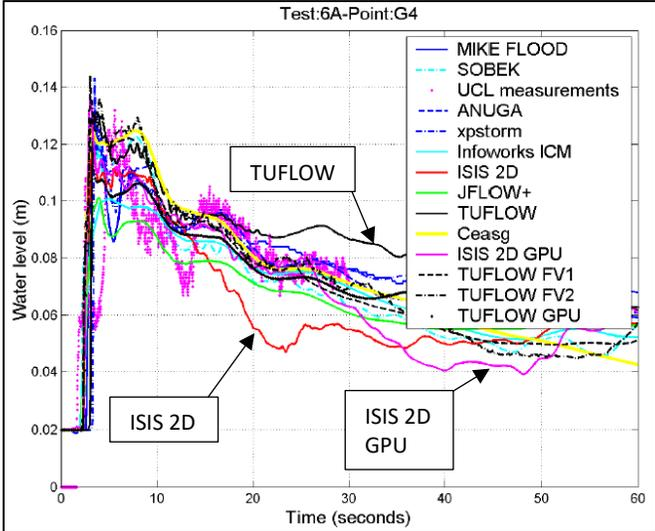
Figure 7-11 Test Point G4 – Water Level versus Time from Report SC120002 (2013)
