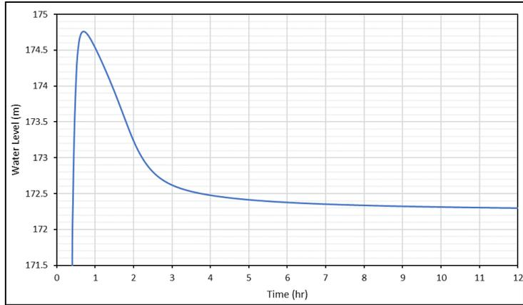
Figure 6-3 Test Point 1 – Water Level versus Time from SRH-2D
