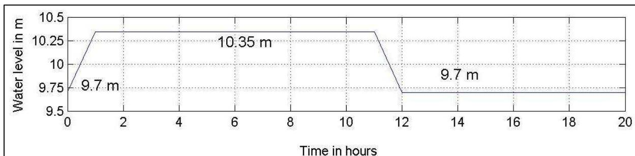
Figure 2-2 Water level hydrograph used as boundary condition.
