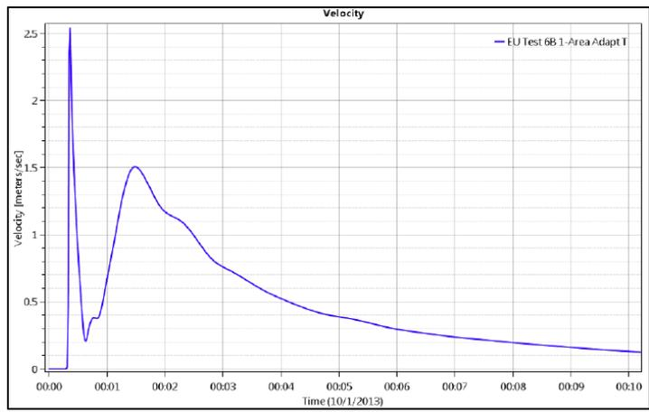
Figure 7-51 Test Point G5 – Velocity versus Time from RD-51 (2018)
