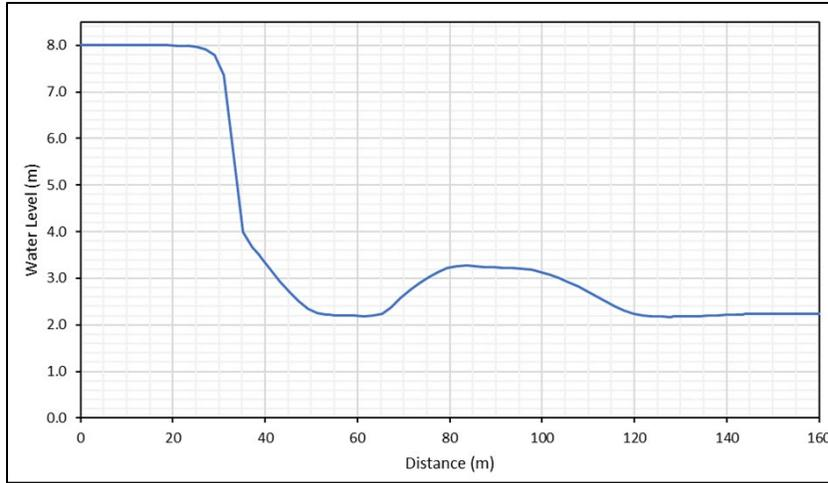
Figure 7-62 Test 6B Maximum Water Surface Elevation Along XS 1 from SRH-2D
