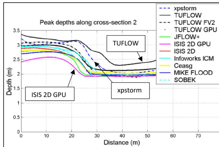
Figure 7-70 Test 6B Maximum Water Surface Elevation Along XS 2 from Report SC120002 (2013)
