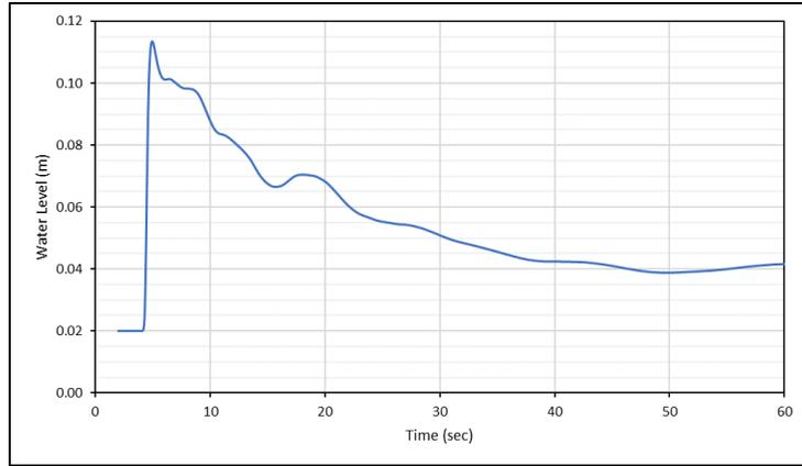
Figure 7-14 Test Point G5 – Water Level versus Time from SRH-2D
