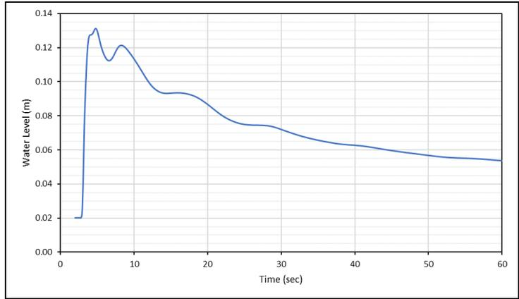
Figure 7-10 Test Point G4 – Water Level versus Time from SRH-2D
