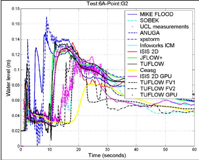
Figure 7-5 Test Point G2 – Water Level versus Time from Report SC120002 (2013)
