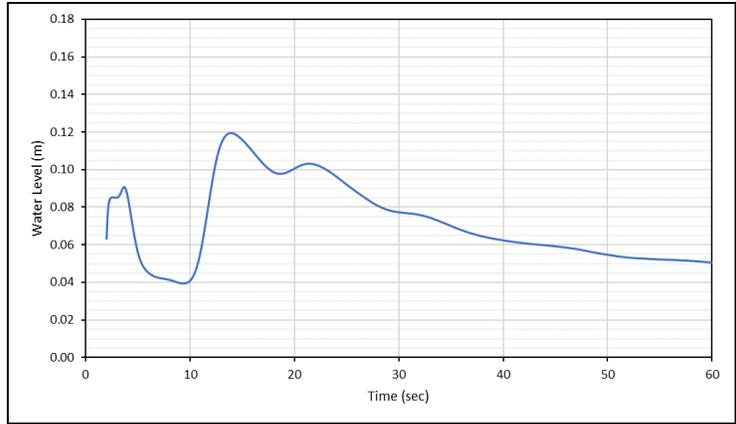
Figure 7-4 Test Point G2 – Water Level versus Time from SRH-2D
