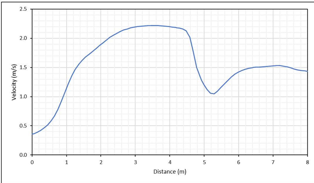
Figure 7-24 Test 6A Maximum Velocity Magnitude Along XS 1 from SRH-2D
