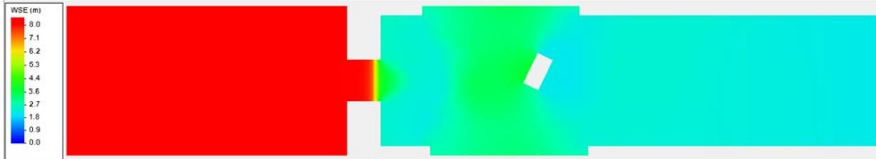
Figure 7-58 Test 6B Maximum Water Surface Elevation (meters) from SRH-2D
