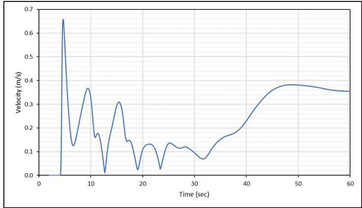
Figure 7-16 Test Point G5 – Velocity versus Time from SRH-2D
