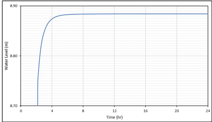
Figure 3-27 Test Point 12 – Water Level versus Time from SRH-2D
