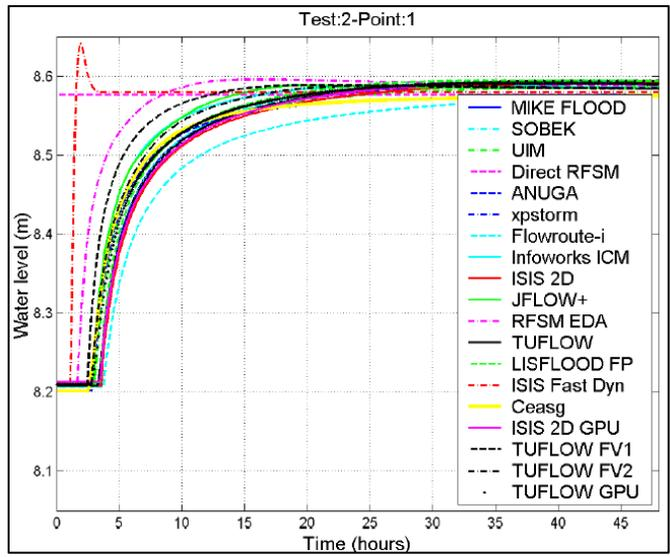
Figure 3-14 Test Point 1 – Water Level versus Time from Report SC120002 (2013)
