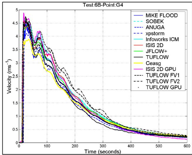
Figure 7-46 Test Point G4 – Velocity versus Time from Report SC120002 (2013)
