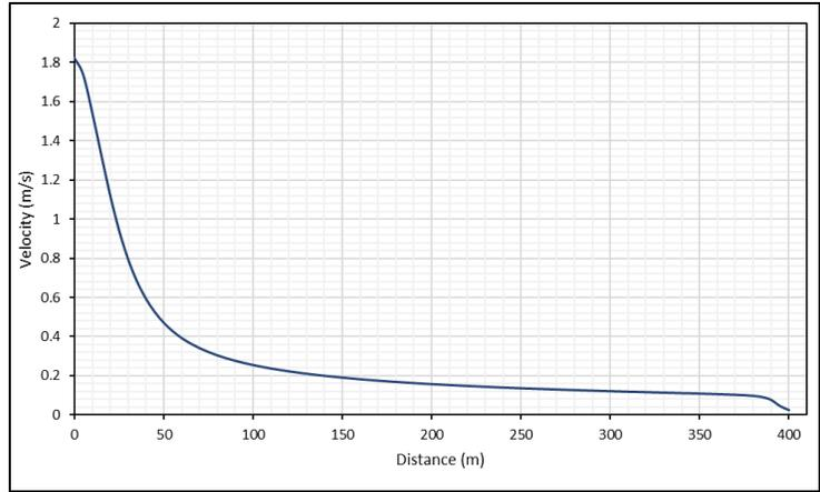
Figure 5-38 Cross Section from Inflow to Point 5 – Velocity versus Distance at 1 Hour from SRH-2D
