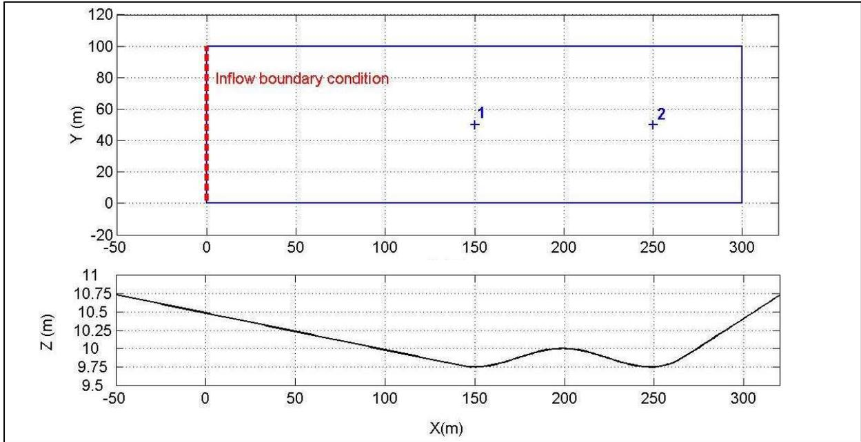
Figure 4-1 Plan (top) and profile (bottom) view of DEM used in Benchmark Test 3.
