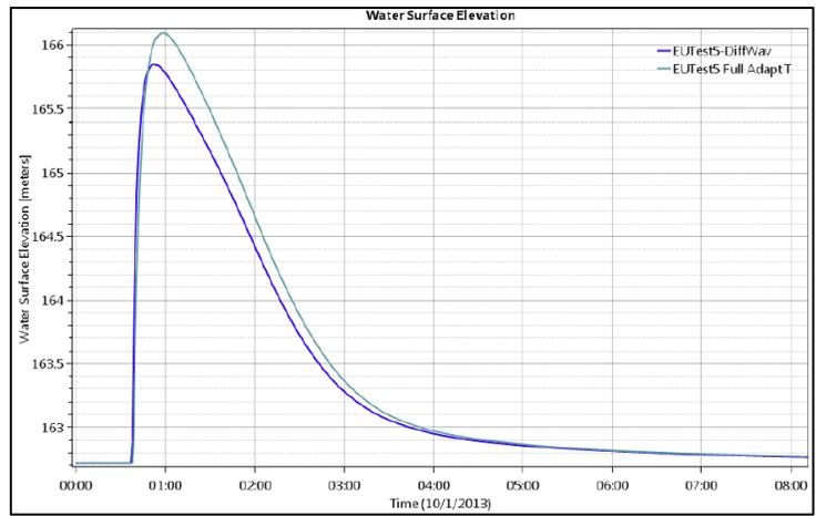
Figure 6-10 Test Point 2 – Water Level versus Time from RD-51 (2018)
