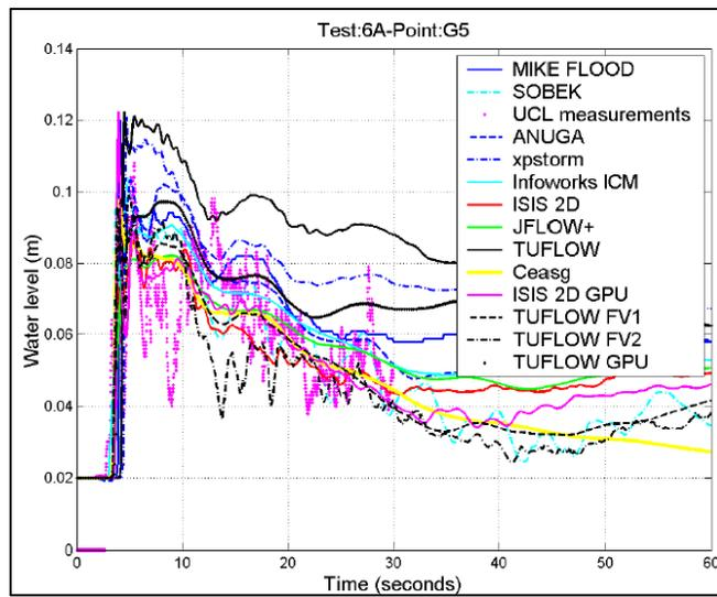
Figure 7-15 Test Point G5 – Water Level versus Time from Report SC120002 (2013)
