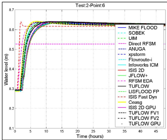
Figure 3-23 Test Point 6 – Water Level versus Time from Report SC120002 (2013)
