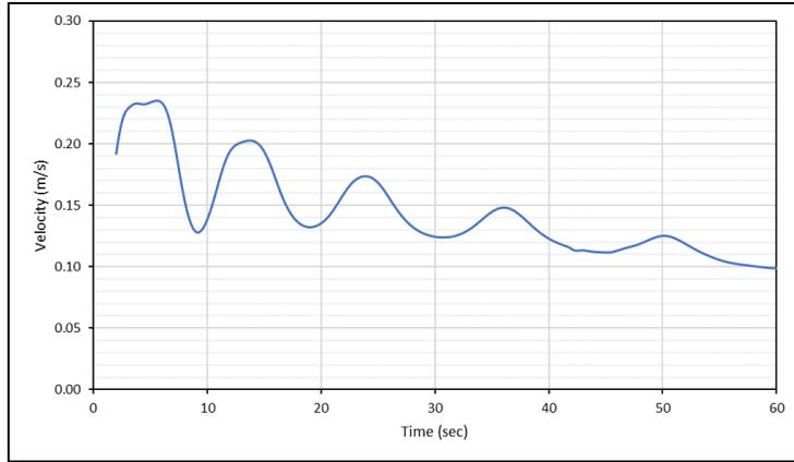
Figure 7-19 Test Point G6 – Velocity versus Time from SRH-2D
