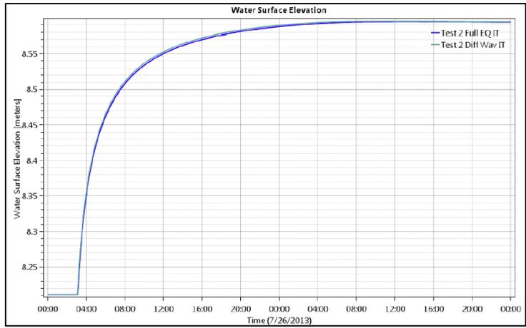
Figure 3-13 Test Point 1 – Water Level versus Time from RD-51 (2018)
