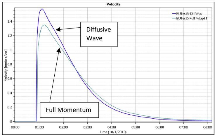
Figure 6-37 Test Point 7 – Velocity versus Time from RD-51 (2018)
