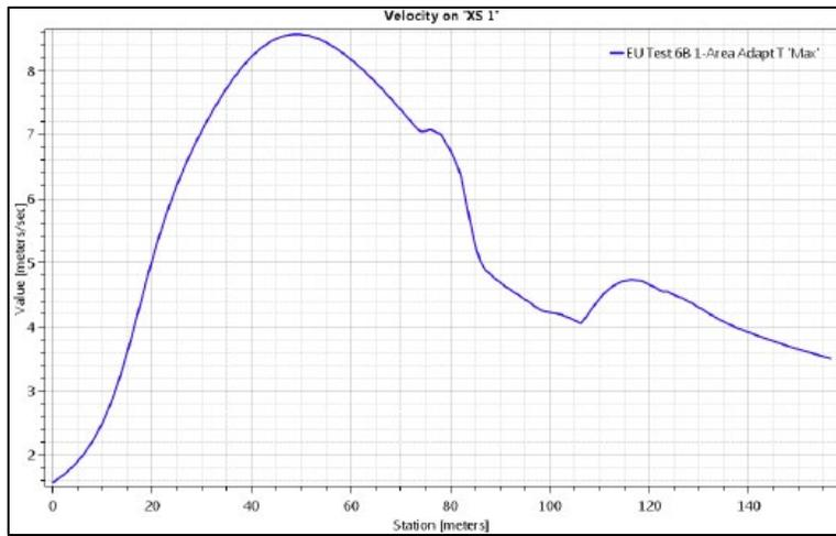
Figure 7-66 Test 6B Maximum Velocity Magnitude Along XS 1 from RD-51 (2018)
