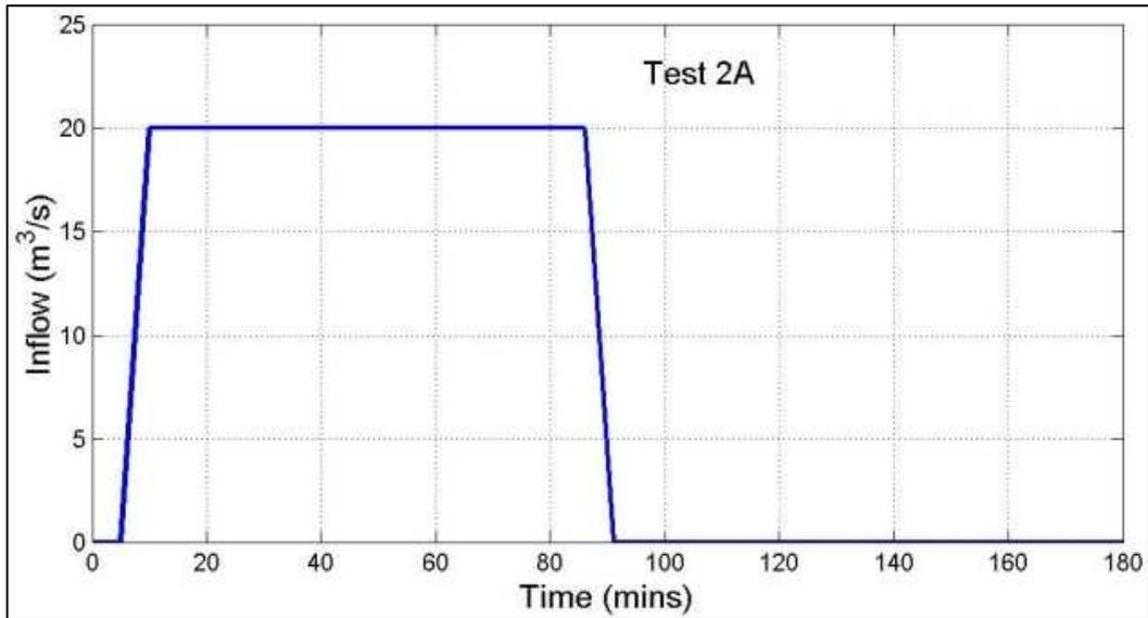
Figure 3-2 Inflow hydrograph used as upstream boundary condition.
