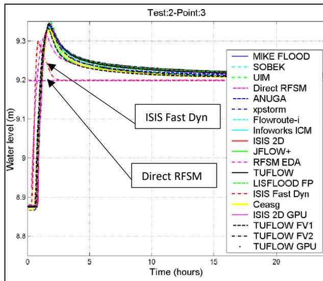
Figure 3-8 Test Point 3 – Water Level versus Time from Report SC120002 (2013)
