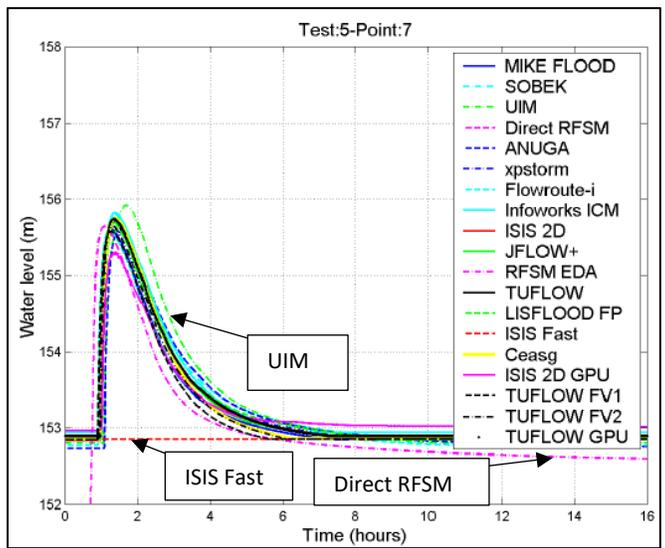
Figure 6-35 Test Point 7 – Water Level versus Time from Report SC120002 (2013)
