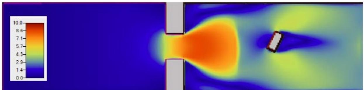
Figure 7-61 Test 6B Maximum Velocity Magnitude (meters per second) from RD-51 (2018)
