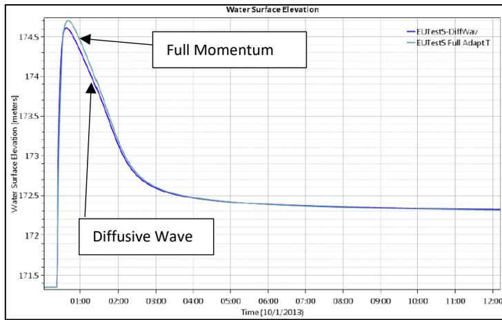
Figure 6-4 Test Point 1 – Water Level versus Time from RD-51 (2018)
