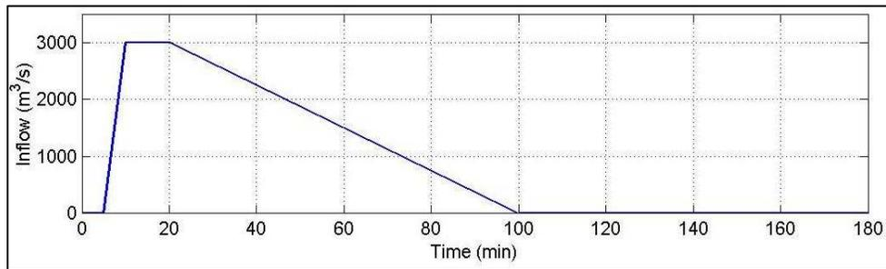
Figure 6-2 Inflow hydrograph used as upstream boundary condition.
