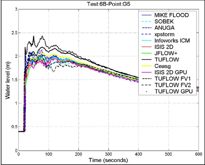
Figure 7-49 Test Point G5 – Water Level versus Time from Report SC120002 (2013)
