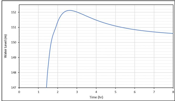
Figure 6-19 Test Point 4 – Water Level versus Time from SRH-2D
