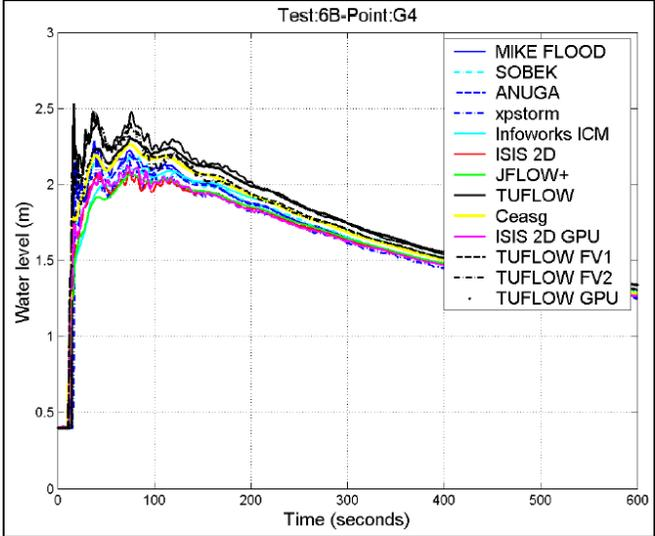
Figure 7-43 Test Point G4 – Water Level versus Time from Report SC120002 (2013)
