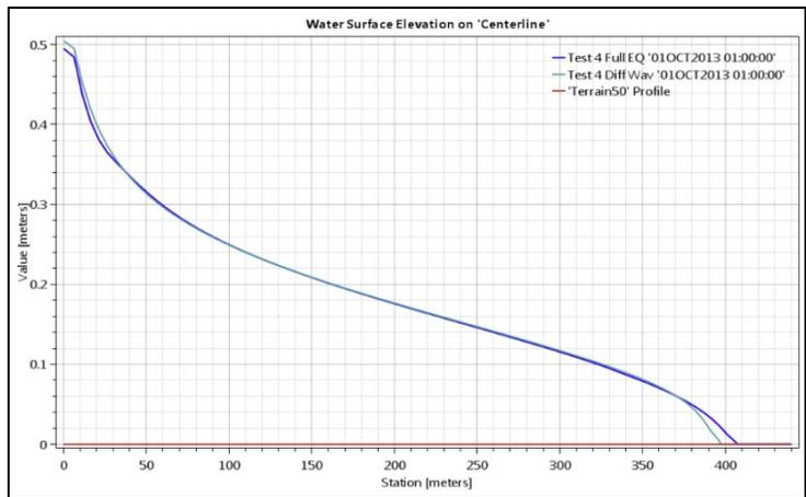
Figure 5-36 Cross Section from Inflow to Point 5 – Water Level versus Distance at 1 Hour from RD-51 (2018)
