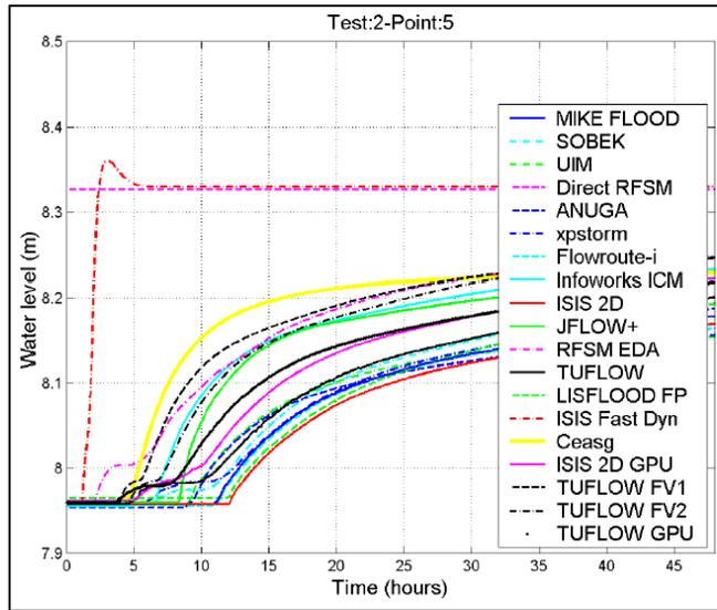
Figure 3-26 Test Point 5 – Water Level versus Time from Report SC120002 (2013)
