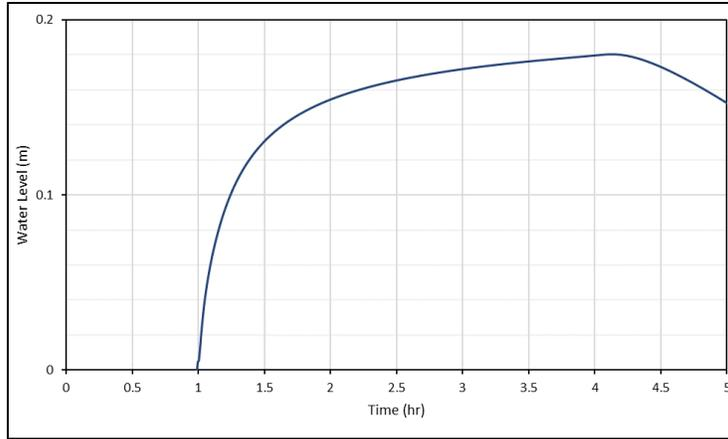
Figure 5-23 Test Point 5 – Water Level versus Time from SRH-2D
