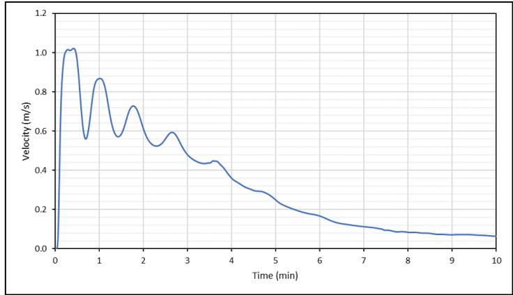
Figure 7-55 Test Point G6 – Velocity versus Time from SRH-2D
