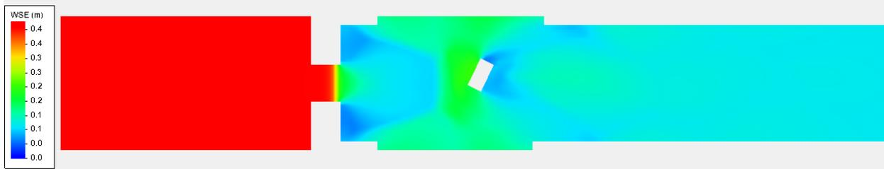
Figure 7-21 Test 6A Maximum Water Surface Elevation (meters) from SRH-2D
