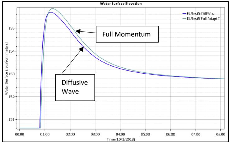
Figure 6-14 Test Point 3 – Water Level versus Time from RD-51 (2018)
