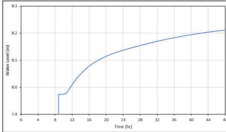
Figure 3-24 Test Point 5 – Water Level versus Time from SRH-2D
