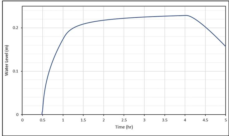
Figure 5-13 Test Point 3 – Water Level versus Time from SRH-2D
