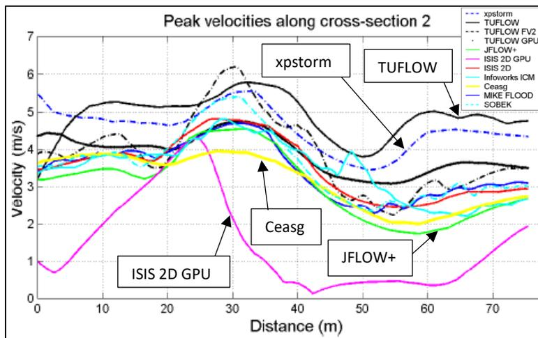
Figure 7-73 Test 6B Maximum Velocity Magnitude Along XS 2 from Report SC120002 (2013)
