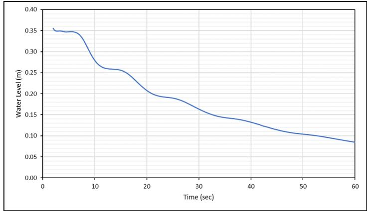
Figure 7-17 Test Point G6 – Water Level versus Time from SRH-2D
