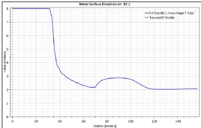
Figure 7-63 Test 6B Maximum Water Surface Elevation Along XS 1 from RD-51 (2018)
