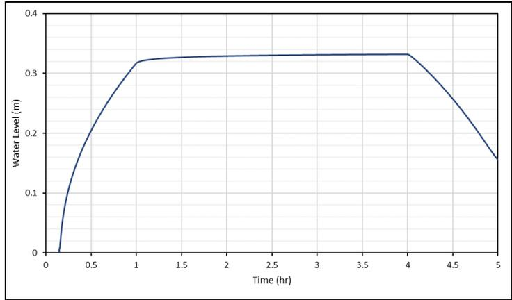
Figure 5-3 Test Point 1 – Water Level versus Time from SRH-2D
