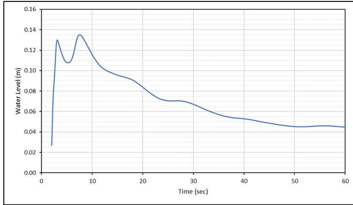
Figure 7-2 Test Point G1 – Water Level versus Time from SRH-2D
