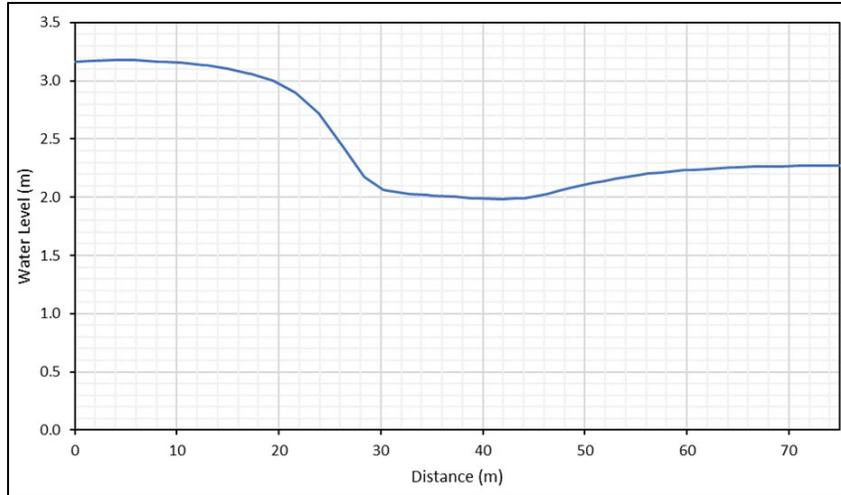
Figure 7-68 Test 6B Maximum Water Surface Elevation Along XS 2 from SRH-2D
