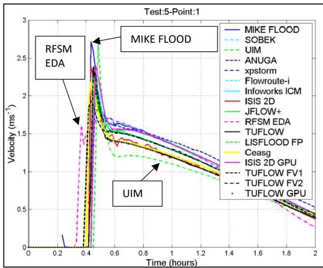
Figure 6-8 Test Point 1 – Velocity versus Time from Report SC120002 (2013)
