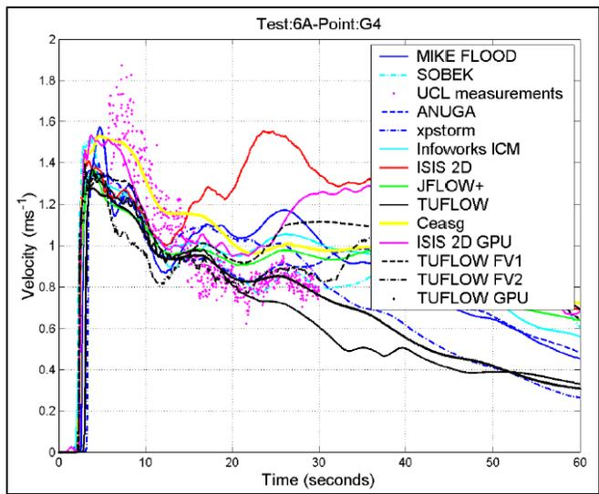
Figure 7-13 Test Point G4 – Velocity versus Time from Report SC120002 (2013)
