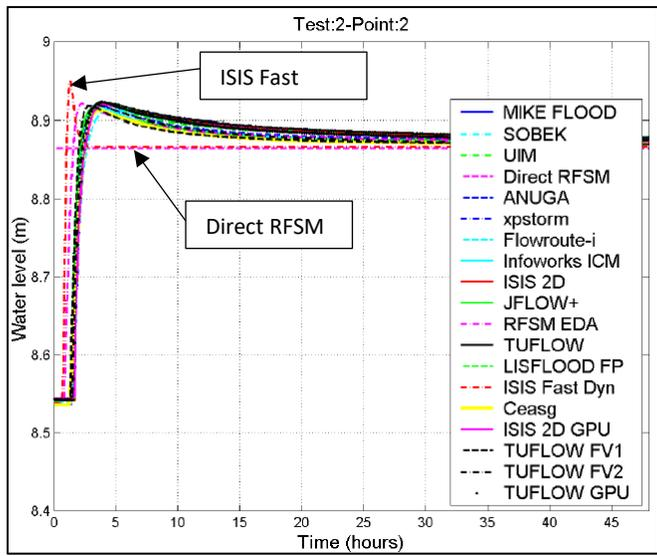
Figure 3-11 Test Point 2 – Water Level versus Time from Report SC120002 (2013)
