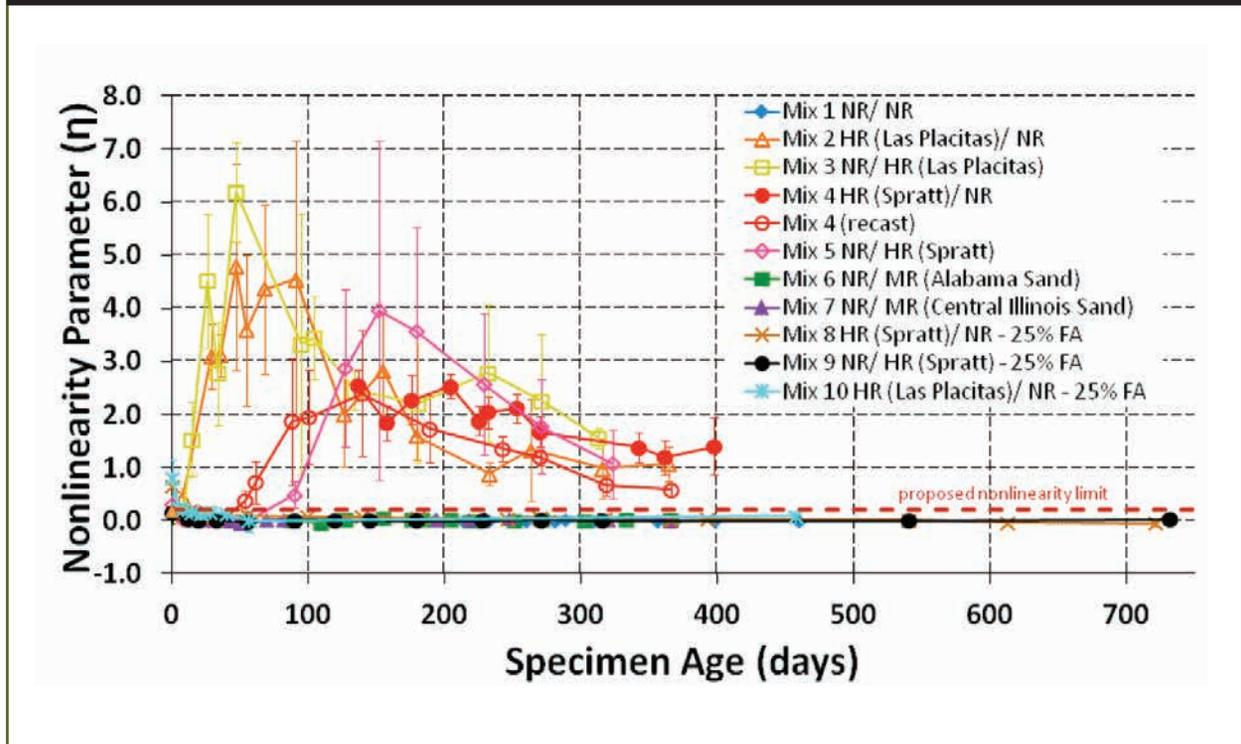
averaged and plotted at each test date. For this representation, the nonlinearity parameter is shown as a function of the time that samples were exposed to ASTM C1293 testing conditions.
