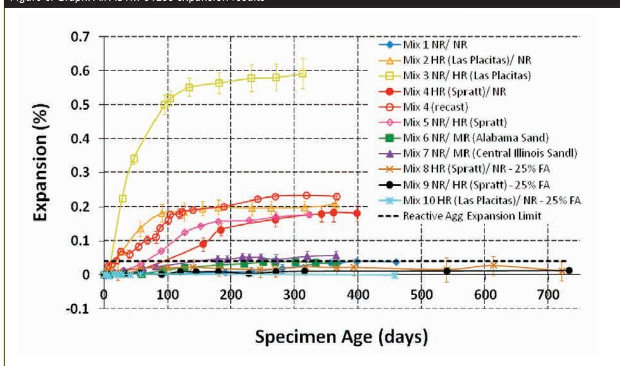
Figure 7. Graph. Greater detail in ASTM C1293 expansion results for the less expansive mixes
