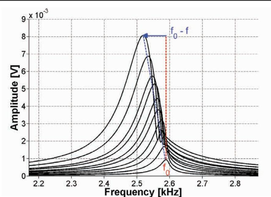
of excitation. Note that  $\eta$  is the negative of the slope of  $(f_0 - f)$  versus the amplitude (the y-axis) in figure 2.
