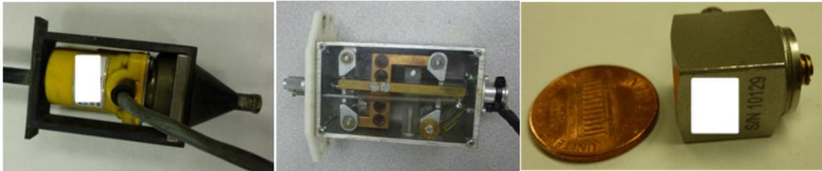
**Figure 245. Photos. Geophone (left), seismometer (center), and high-accuracy piezoelectric accelerometer (right).**
