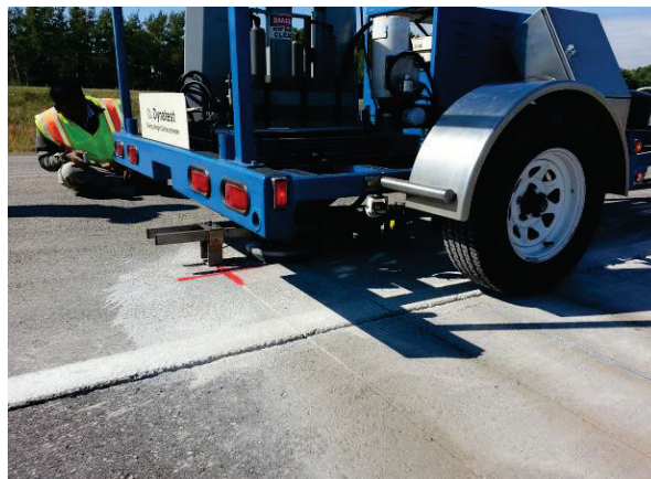
Figure 29. Photo. Alignment of project sensor with FWD sensor.
