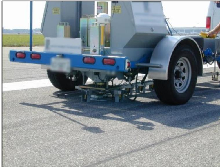
**Figure 4. Photo. Impulse loading or FWD device.**
