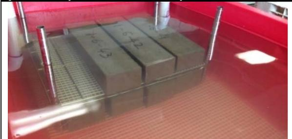
**Figure 6. View of specimens being cured in interconnected lime water tanks. (Source: FHWA)**
