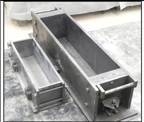
In this case, the combined mass of the concrete specimen and the mold is approximately 45 lb (20.5 kg), i.e. less than 50 percent of the total mass of the standard size beam. This is a dramatic reduction in total mass and makes the smaller size specimens much easier and safer to use. Figure 3 visually compares the mold for both beam sizes. For the sake of brevity, the two sizes will be
