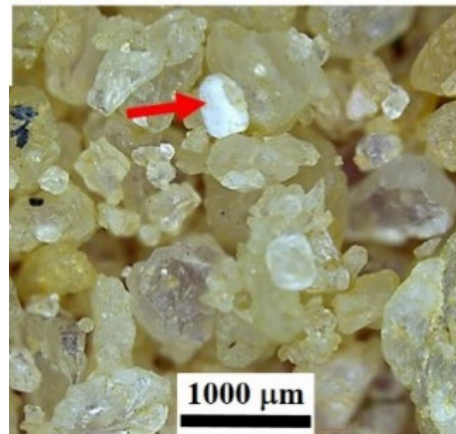
Source: FHWA. Note: The arrow shows a white coating on a surface of a sand grain. D. Example of representative portions of sand.
