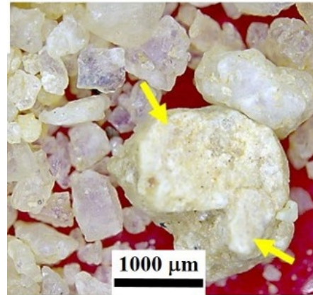
Source: FHWA. Note: The arrows show what seems to be a secondary deposit attached to a sand grain. C. Example of representative portions of sand.
