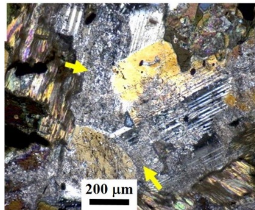
Source: FHWA. Note: the arrows denote alteration of some plagioclase feldspars into fine-grained micas and clay (shown by arrows).
