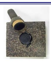
**Figure 3.** Pull-off test specimen on diabase stone after testing.
