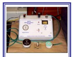
Figure 2. The Pneumatic Adhesion Tensile Testing Instrument (PATTI) is shown.
