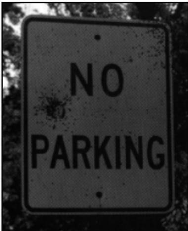
This sign has been struck by several shotgun blasts. The retro-reflective material is severely damaged and while the sign is still legible during the day, it is not at night.
