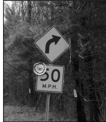
This sign is adequate under normal conditions but when tampered with, it can induce a lack of respect in the driver, additionally the drivers attention is diverted from the warning message. Local community employees should be trained to report or resolve such conditions immediately.
