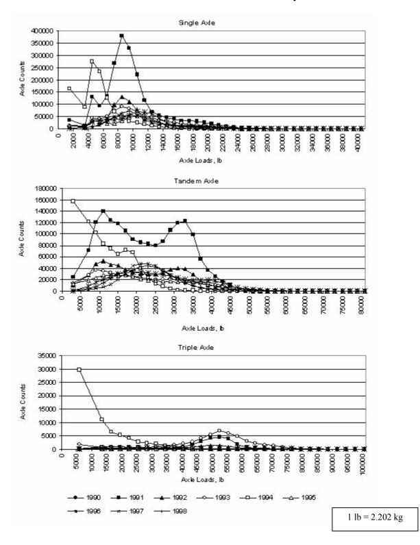
Figure 15. Use of the mean of 1991 and 1992 annual axle load spectra to obtain base annual spectrum.
