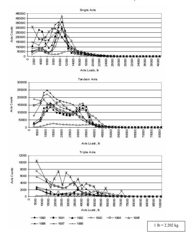
Figure 14. Use of the mean of 1991, 1992, and 1995 annual axle load spectra to obtain base annual spectrum.
