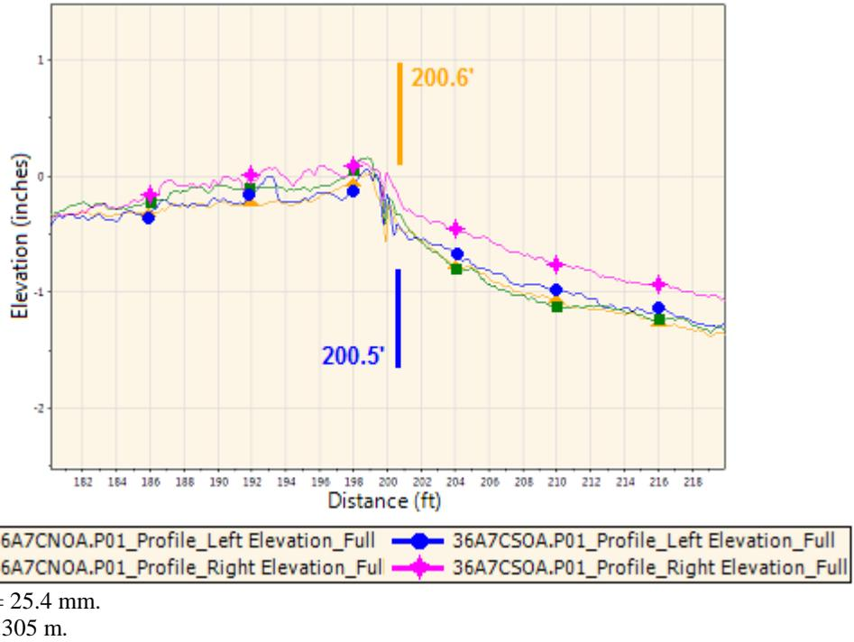
**Figure 17. Chart. Example of a conventional bridge profile in St. Lawrence County, NY, at first interface (northbound direction).**
