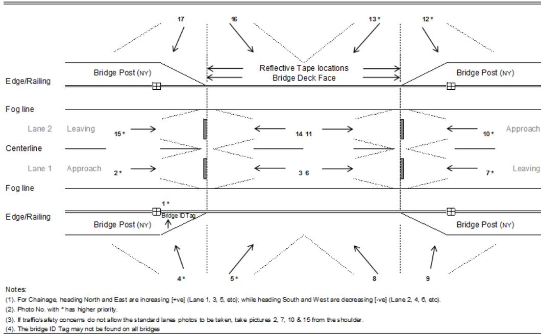
Figure 7. Log. Form 2B—photo diagram.
