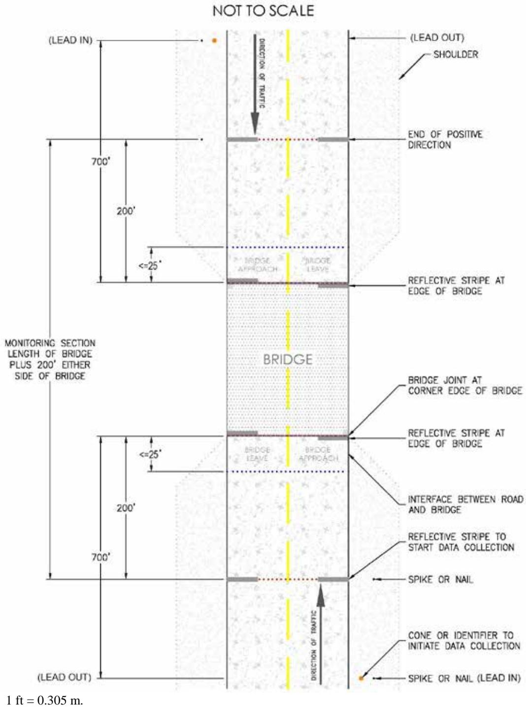
**Figure 2. Drawing. Layout of bridge site with perpendicular joints.**
