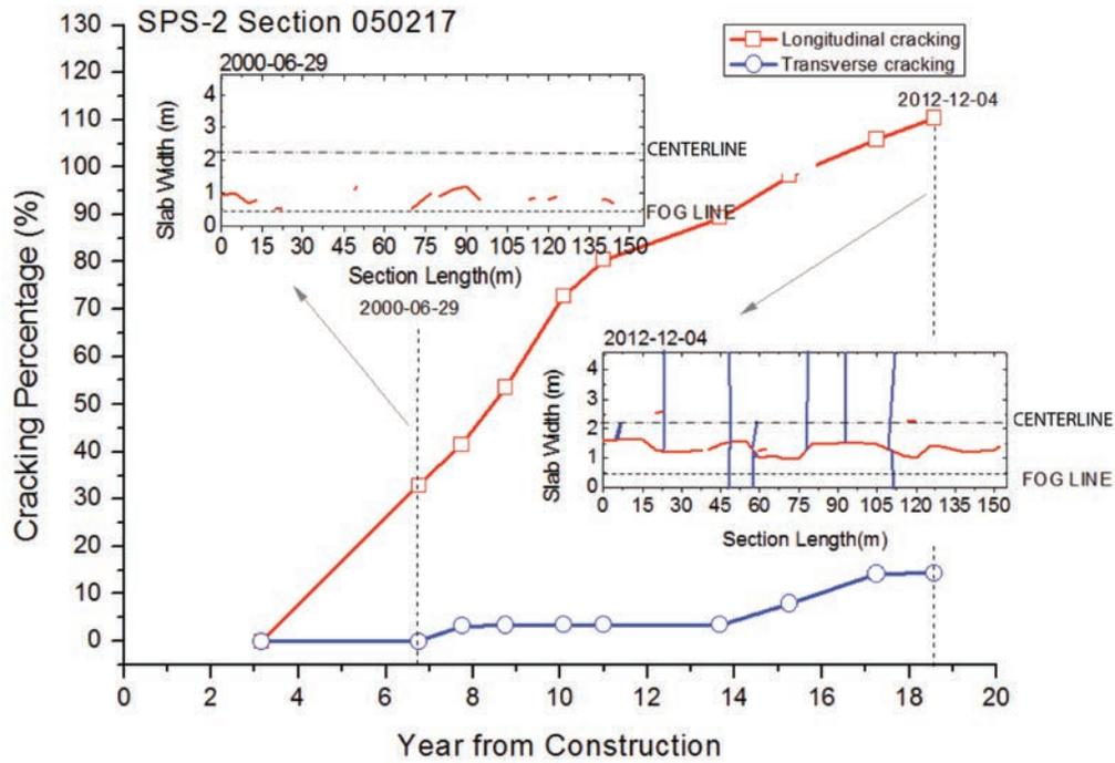
Figure 20. The development of cracking in Arkansas-0218 section.
