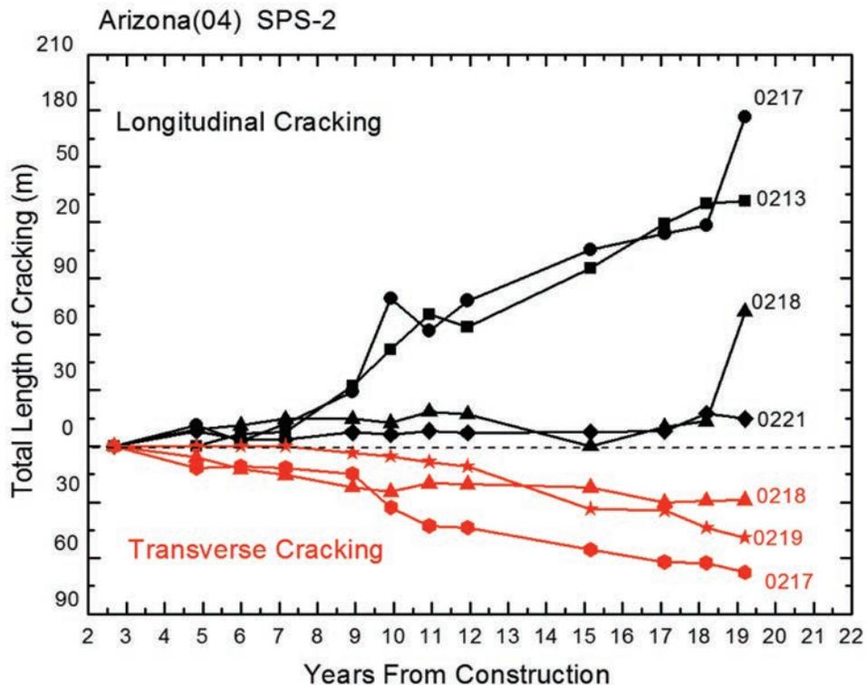
Figure 15. The development of cracking in Arizona-0213 section.
