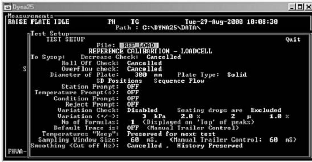
Figure G-1.25 Test Setup - Reference Calibration - Loadcell
