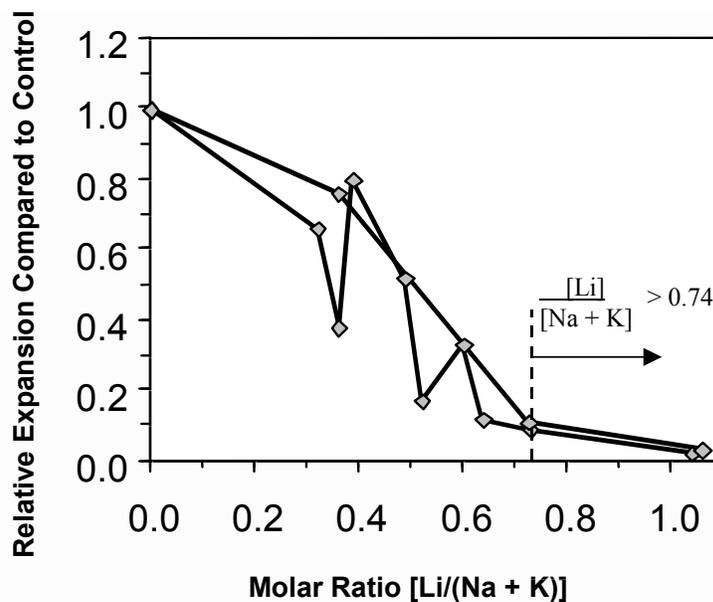
Figure 11. Relative Expansion of Mortar Bars Containing Lithium Compounds (After McCoy and Caldwell, 1951).
