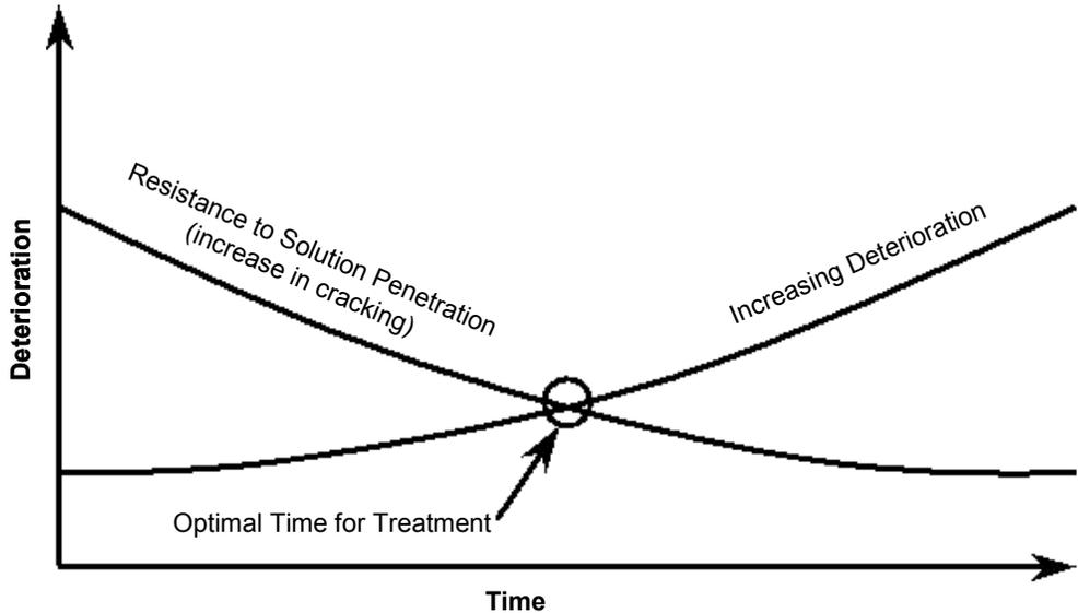
Figure 40. Optimal Time for Lithium Treatment Applied Topically (Johnston, et al., 2000).
