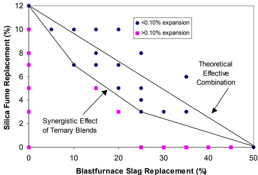
Figure 10. Synergistic Effects of Ternary Blends in Controlling ASR Expansion Using ASTM C 1260 (After Bleszynski, et al., 2000).
