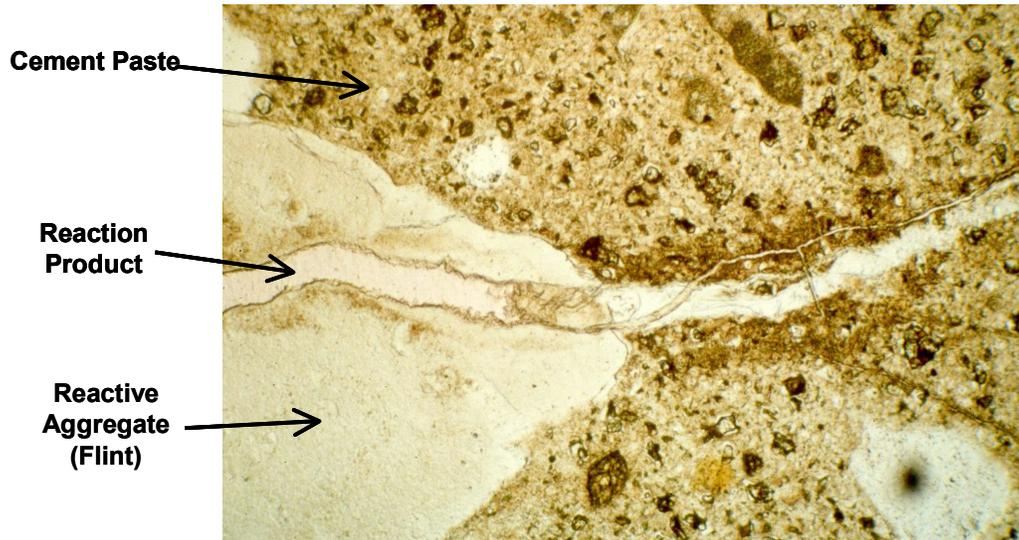
Figure 5. Thin-Section Cut of ASR-Damaged Concrete, Showing ASR Gel and Typical Crack Pattern (Through Aggregate and Into Surrounding Matrix).
