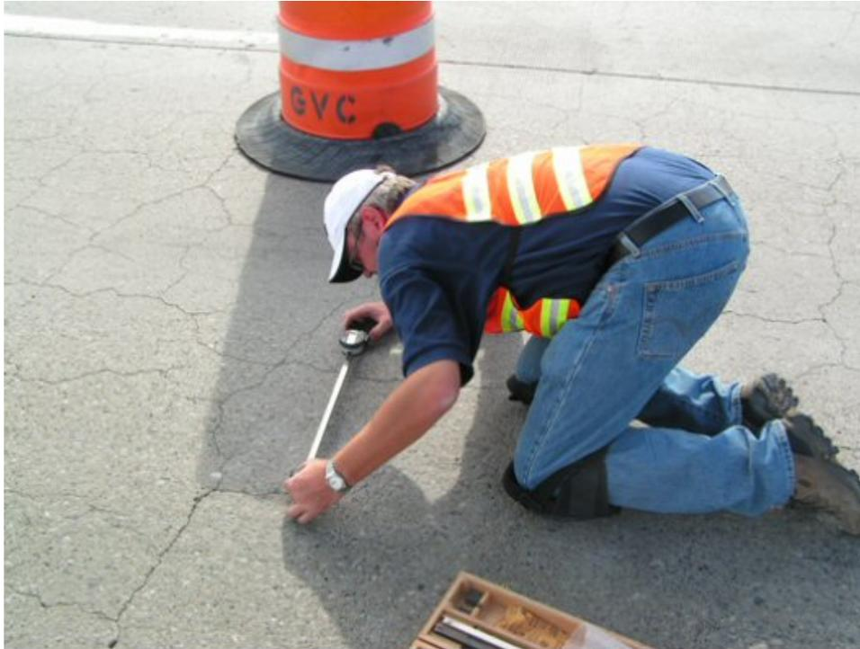
Figure 37. Making Length-Change Measurements on a Treated Pavement in Mountain Home, ID.
