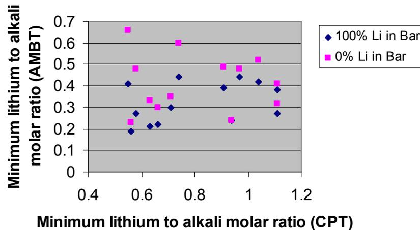
Figure 13. Comparison Between the Minimum Lithium to Alkali Molar Ratios to Control ASR Expansion Based on CPT and AMBT Results (Plot of Data in Table 9) (Tremblay, et al. 2005).
