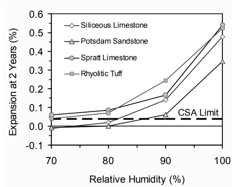
Figure 3. Effects of Relative Humidity on Expansion Using the ASTM C 1293 Storage Regime (Pedneault, 1996).
