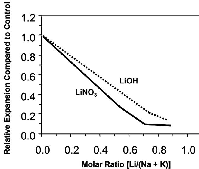
Figure 12. Relative Expansion of Concrete Prisms Containing Lithium Compounds.
