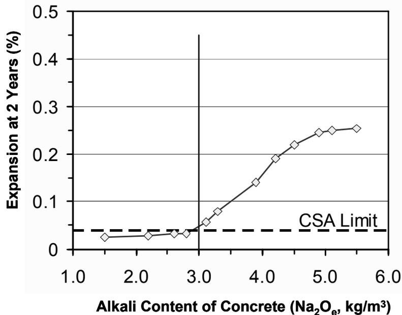
Figure 2. Effects of Alkali Content on Expansion of Prisms Stored Over Water at 38 °C (After Thomas, 2002).
