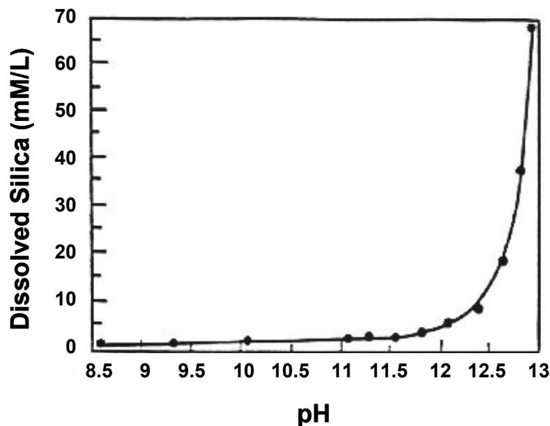
Figure 4. Effects of pH on Dissolution of Amorphous Silica (Tang and Su-Fen, 1980).
