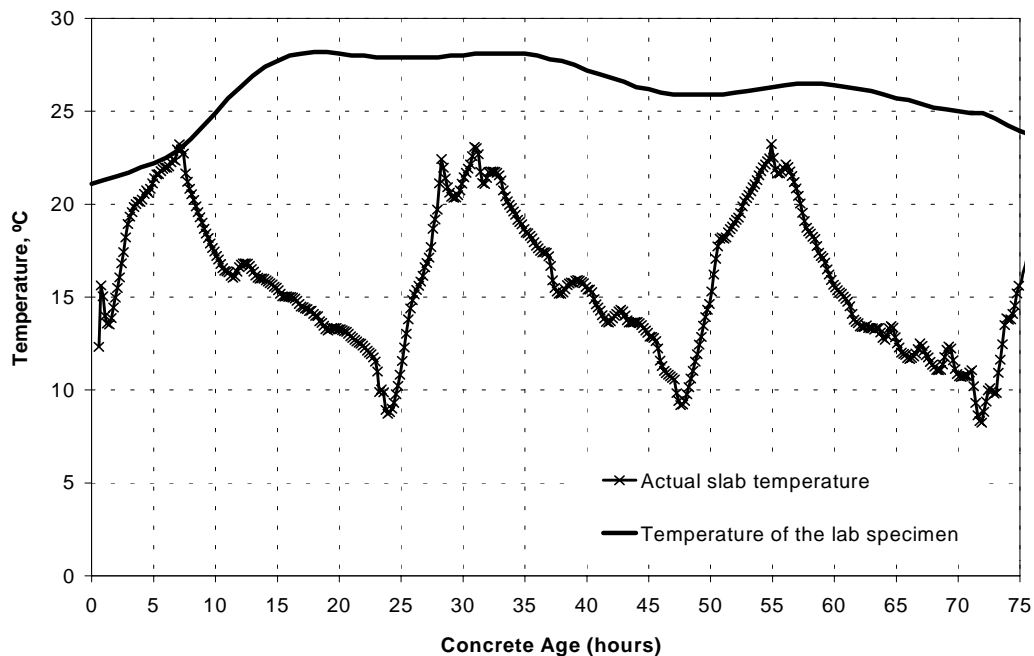
Figure 1. The temperature histories of the concrete slab and the lab specimen.
