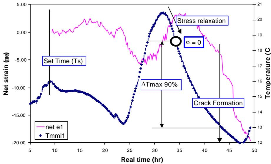
Figure 3. Schematic of stress relaxation in young concrete and determination of  $\Delta T_{\max}$  90 percent for axial stress ( $\sigma_{\text{axial}}$ ) calculation.
