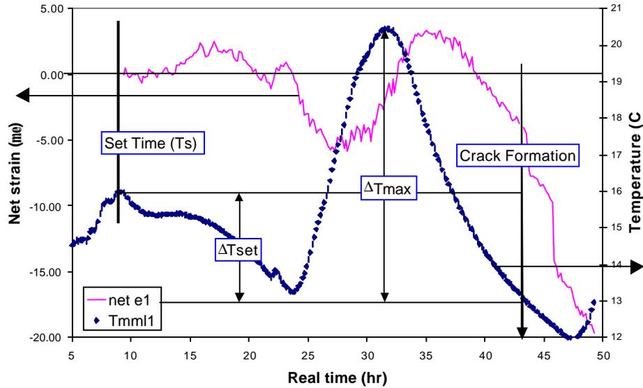
Figure 2. Plot of temperature and net strain vs. time for PCC pavement.
