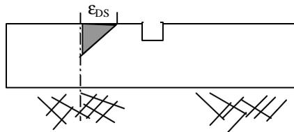
Figure 4. Drying shrinkage distribution through the thickness of the pavement.
