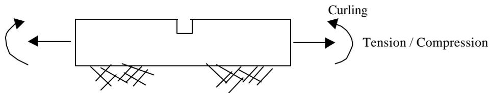
Figure 1. Free-body diagram of loads acting on the pavement.
