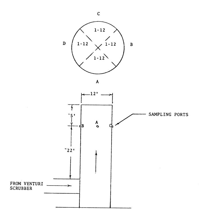
FIGURE 3. SCRUBBER OUTLET STACK DIMENSIONS & SAMPLING POINT LOCATIONS
