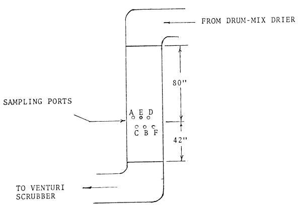
FIGURE 2. VENTURI INLET DUCT DIMENSIONS & SAMPLING POINT LOCATIONS
