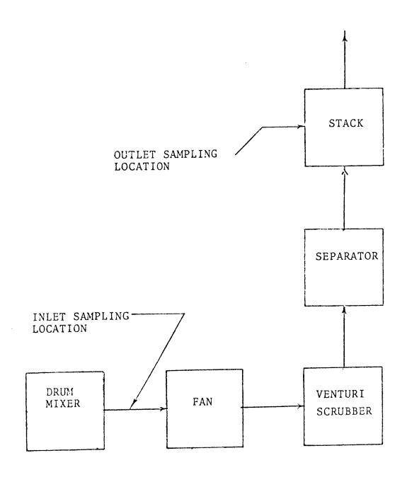
FIGURE 1. PROCESS AIR FLOW SCHEMATIC & SAMPLING LOCATIONS
