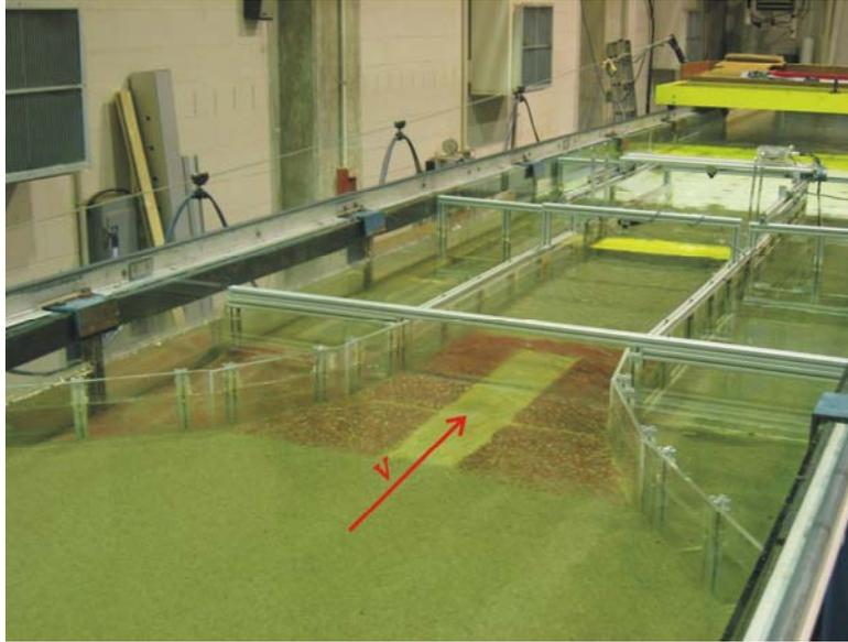
Figure 8. Photo. Approach section of the test flume.
