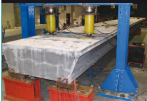
Figure 2. Full-scale shear test.
