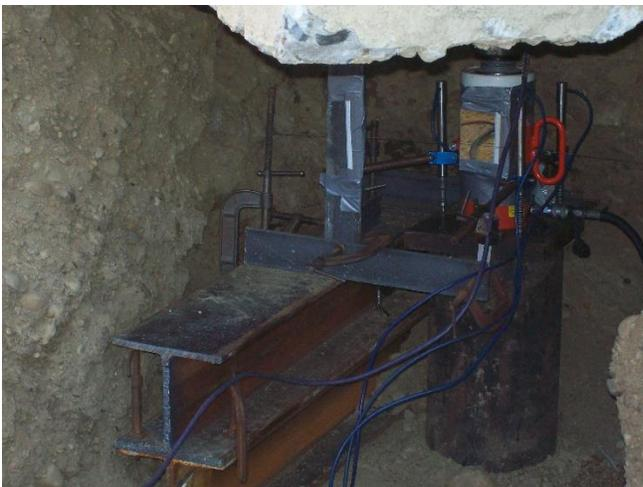
A. Load test setup for north abutment
