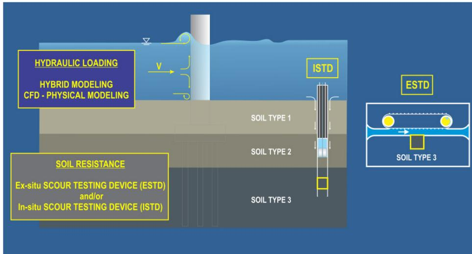
**Figure 2. Diagram. Hydraulic Loading—Soil Resistance Approach.<sup>(6)</sup>**
