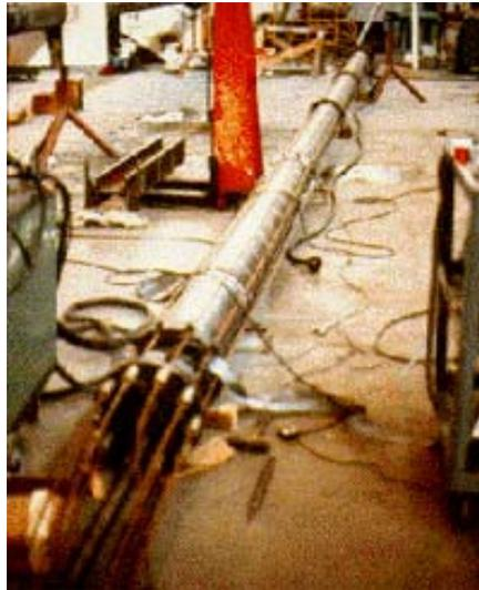
**Figure 5. Photo. Laboratory instrumentation of a pipe pile for field load testing.<sup>(7)</sup>**
