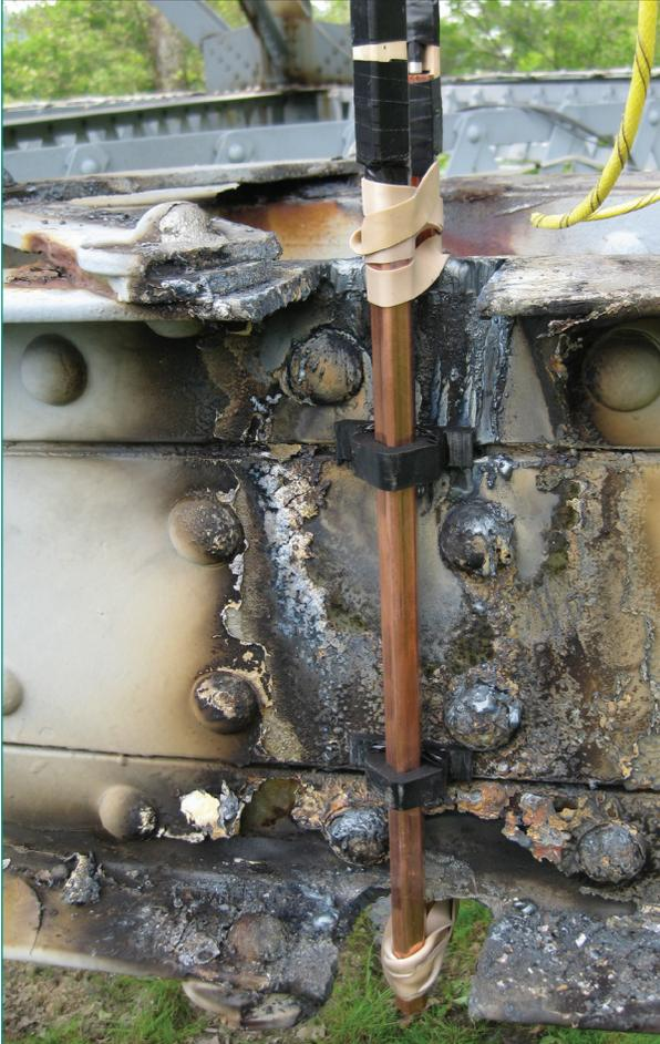
For all members that were instrumented, the dynamic amplification from the first blast ranged from 1.08 to 1.30. For the second blast event, the amplification factors ranged from 1.17 to 1.41.
