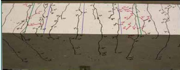
Figure 4. Cracking in splice beam with HG mix and stirrups after failure (top surface of beam shown).
