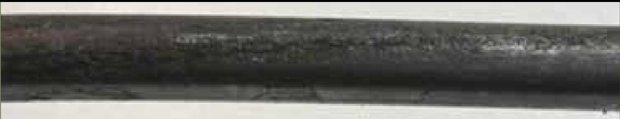
Figure 19. Crevice corrosion between two stressed wires on 0.8 percent chloride concentration multi-strand specimen.
