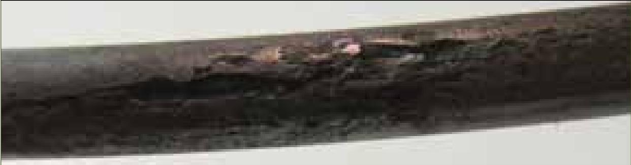
Figure 18. Crevice corrosion between two stressed wires on 0.4 percent chloride concentration multi-strand specimen.
