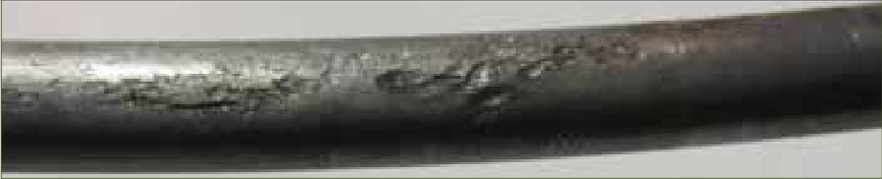
Figure 17. Pitting corrosion observed on a stressed wire of 0.8 percent chloride concentration multi-strand specimen.
