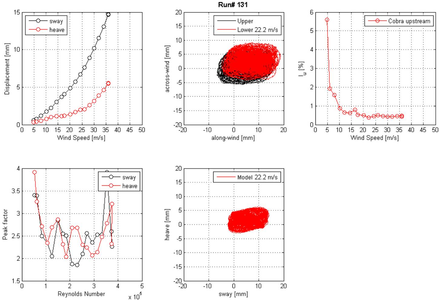
**Figure 113. Graph. Mean displacement and peak factor from the laser, motion path at one wind speed, and intensity of turbulence measured at the entrance of the test section for run 131.**
