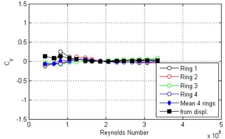
Figure 156. Graph. Response of the cable as a function of wind speed or Reynolds number as measured by the lasers, accelerometers, and surface pressures for run 219.
