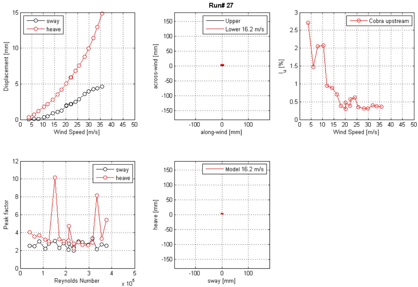
**Figure 60. Graph. Mean displacement and peak factor from the laser, motion path at one wind speed, and intensity of turbulence measured at the entrance of the test section for run 27.**
