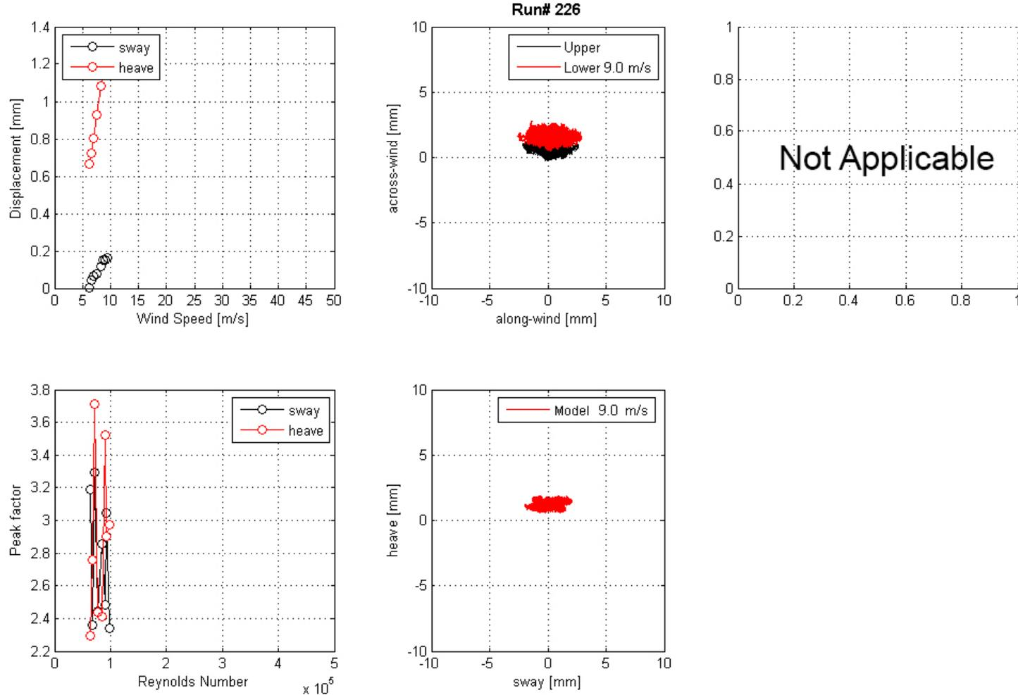
**Figure 163. Graph. Mean displacement and peak factor from the laser, motion path at one wind speed, and intensity of turbulence measured at the entrance of the test section for run 226.**
