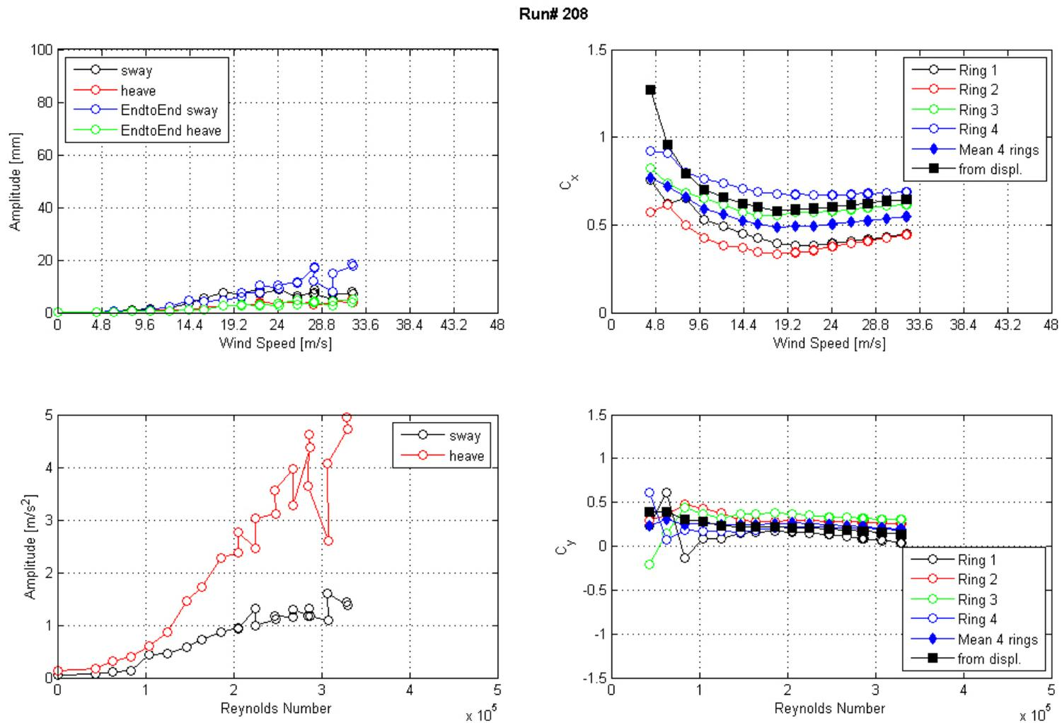
**Figure 148. Graph. Response of the cable as a function of wind speed or Reynolds number as measured by the lasers, accelerometers, and surface pressures for run 208.**
