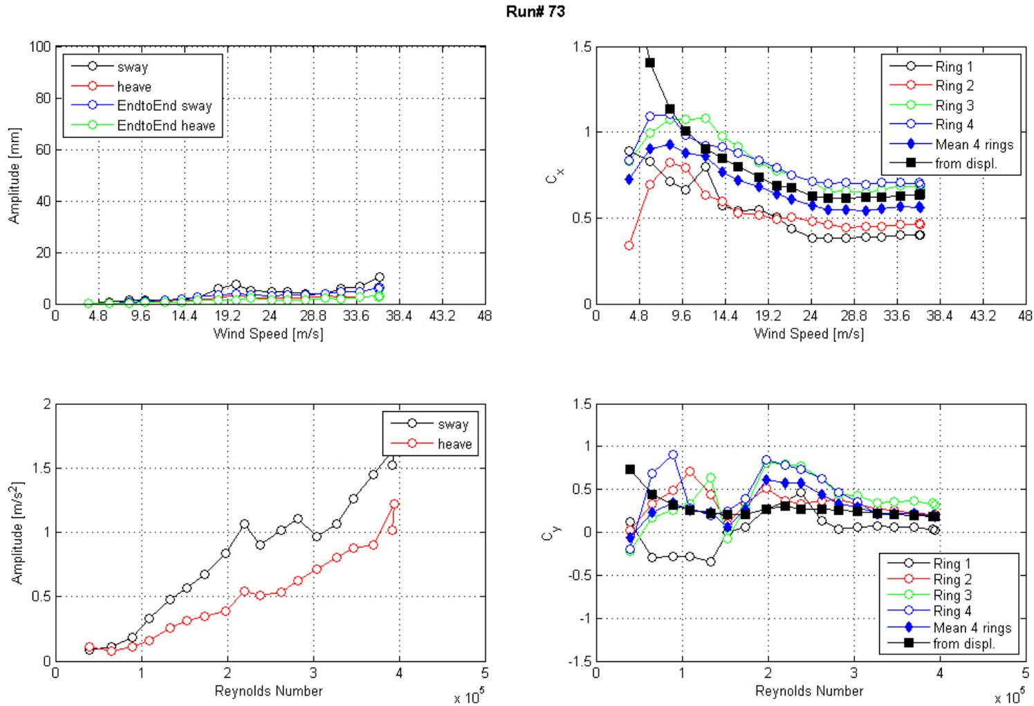
**Figure 90. Graph. Response of the cable as a function of wind speed or Reynolds number as measured by the lasers, accelerometers, and surface pressures for run 73.**
