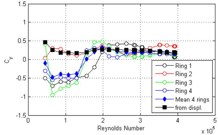
Figure 106. Graph. Response of the cable as a function of wind speed or Reynolds number as measured by the lasers, accelerometers, and surface pressures for run 122.
