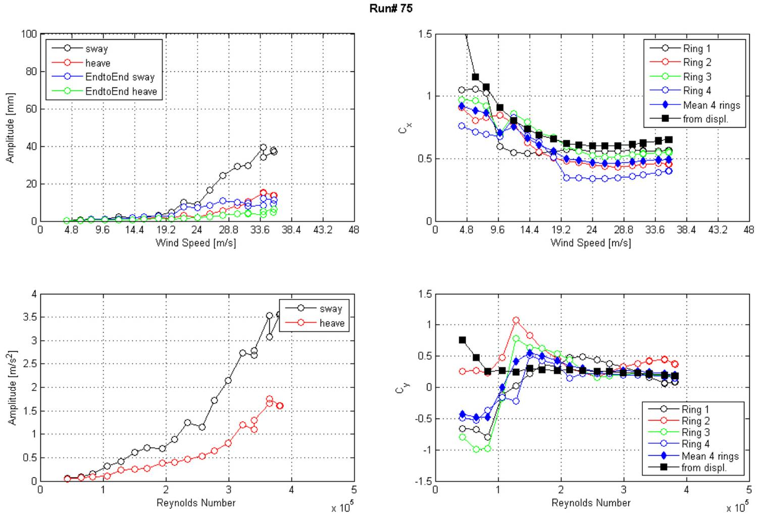
**Figure 92. Graph. Response of the cable as a function of wind speed or Reynolds number as measured by the lasers, accelerometers, and surface pressures for run 75.**
