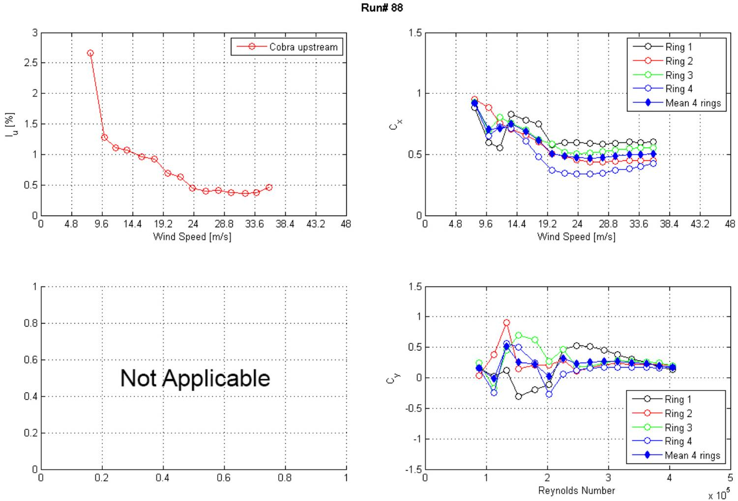
**Figure 96. Graph. Intensity of turbulence measured at the entrance of the test section and  $C_x$  and  $C_y$  calculated from surface pressure measurements as a function of Reynolds number and wind speed for run 88.**
