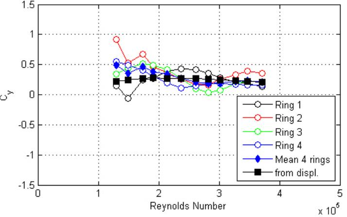
Figure 108. Graph. Response of the cable as a function of wind speed or Reynolds number as measured by the lasers, accelerometers, and surface pressures for run 123.
