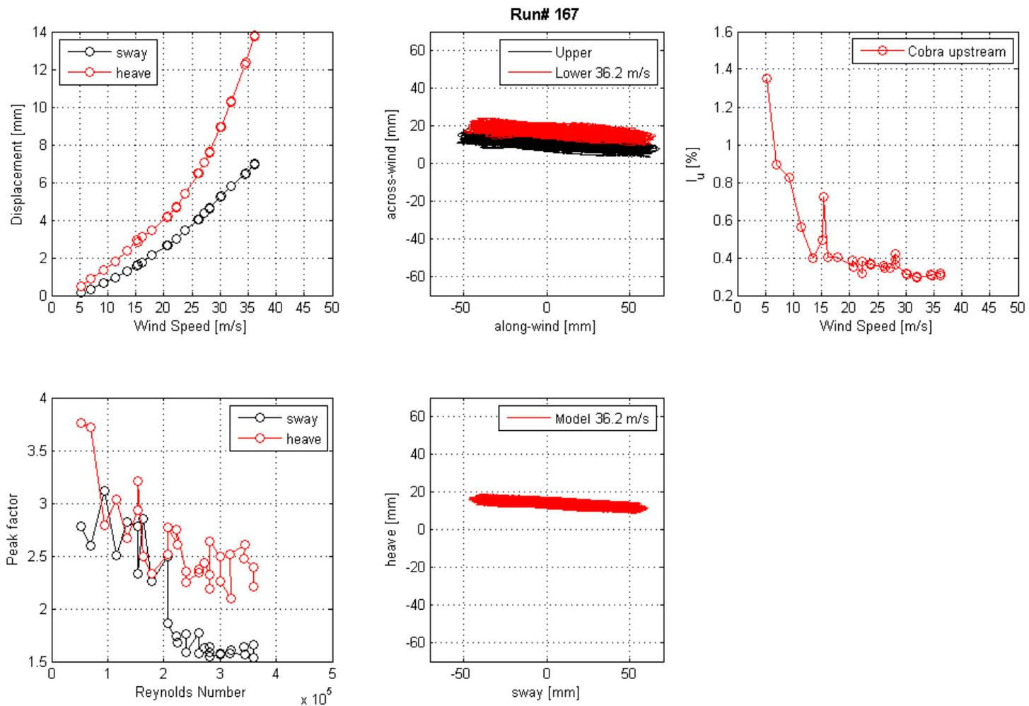
**Figure 135. Graph. Mean displacement and peak factor from the laser, motion path at one wind speed, and intensity of turbulence measured at the entrance of the test section for run 167.**
