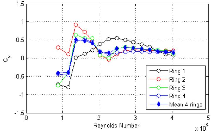
Figure 98. Graph. Intensity of turbulence measured at the entrance of the test section and  $C_x$  and  $C_y$  calculated from surface pressure measurements as a function of Reynolds number and wind speed for run 92.
