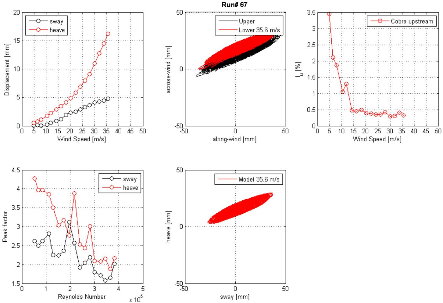
**Figure 85. Graph. Mean displacement and peak factor from the laser, motion path at one wind speed, and intensity of turbulence measured at the entrance of the test section for run 67.**
