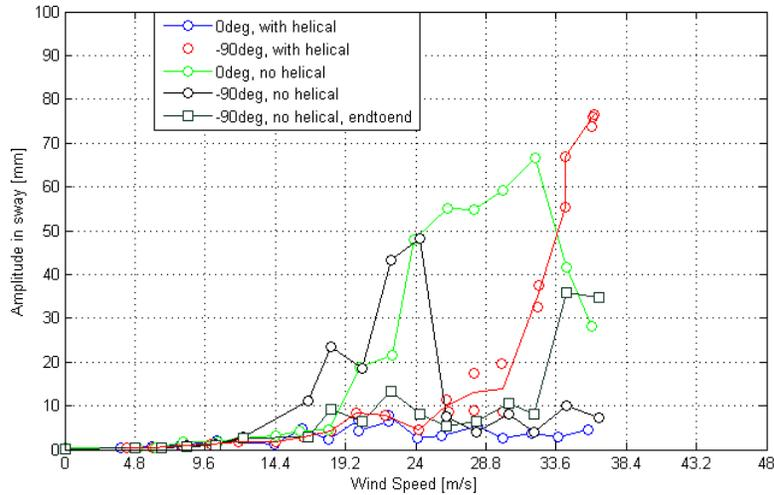
**Figure 44. Graph. Amplitude of motion in sway and end-to-end sway for cable rotated at -90 and 0 degrees and inclined at 60 degrees in smooth flow with and without a helical fillet.**
