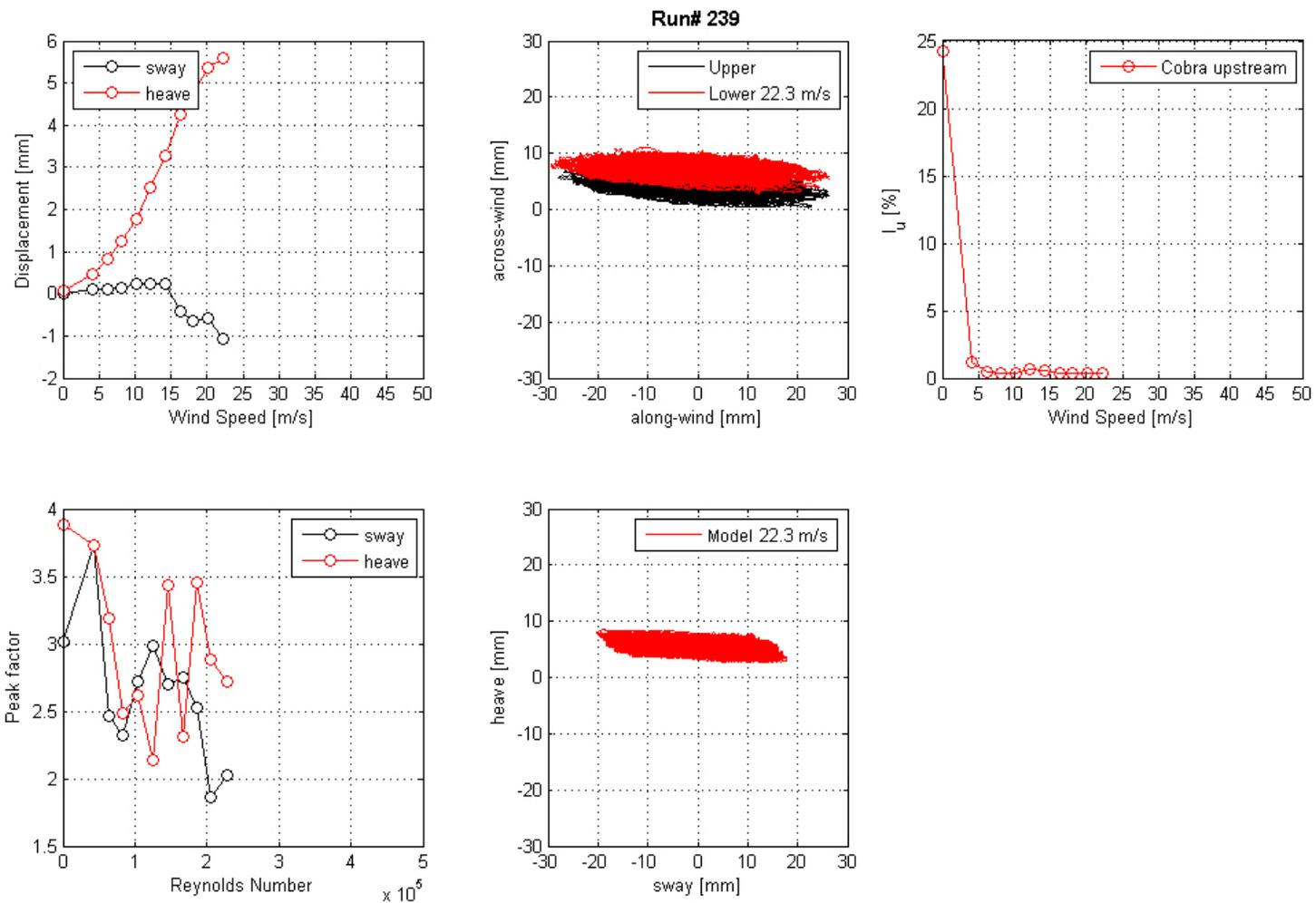
**Figure 171. Graph. Mean displacement and peak factor from the laser, motion path at one wind speed, and intensity of turbulence measured at the entrance of the test section for run 239.**
