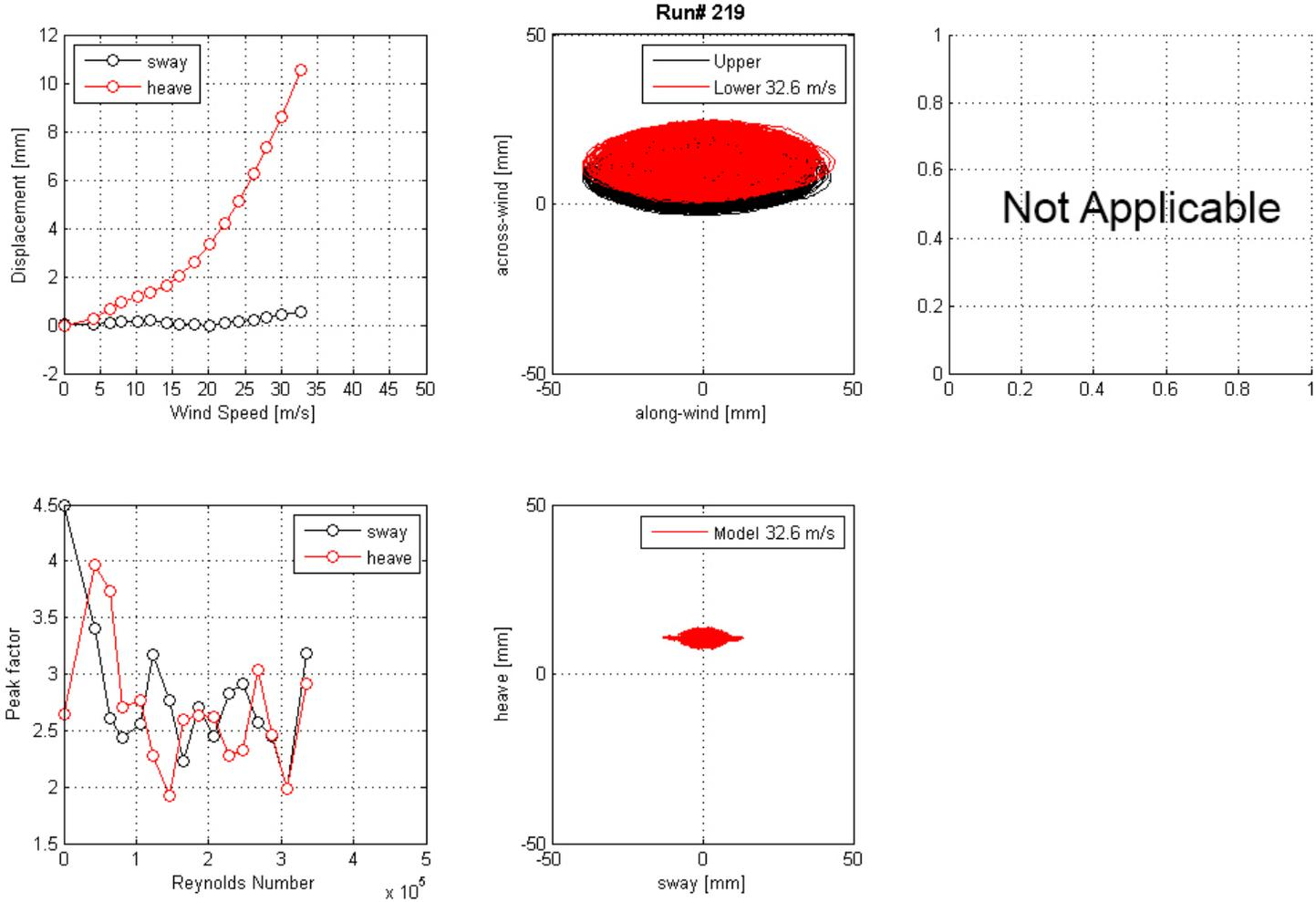
**Figure 157. Graph. Mean displacement and peak factor from the laser, motion path at one wind speed, and intensity of turbulence measured at the entrance of the test section for run 219.**
