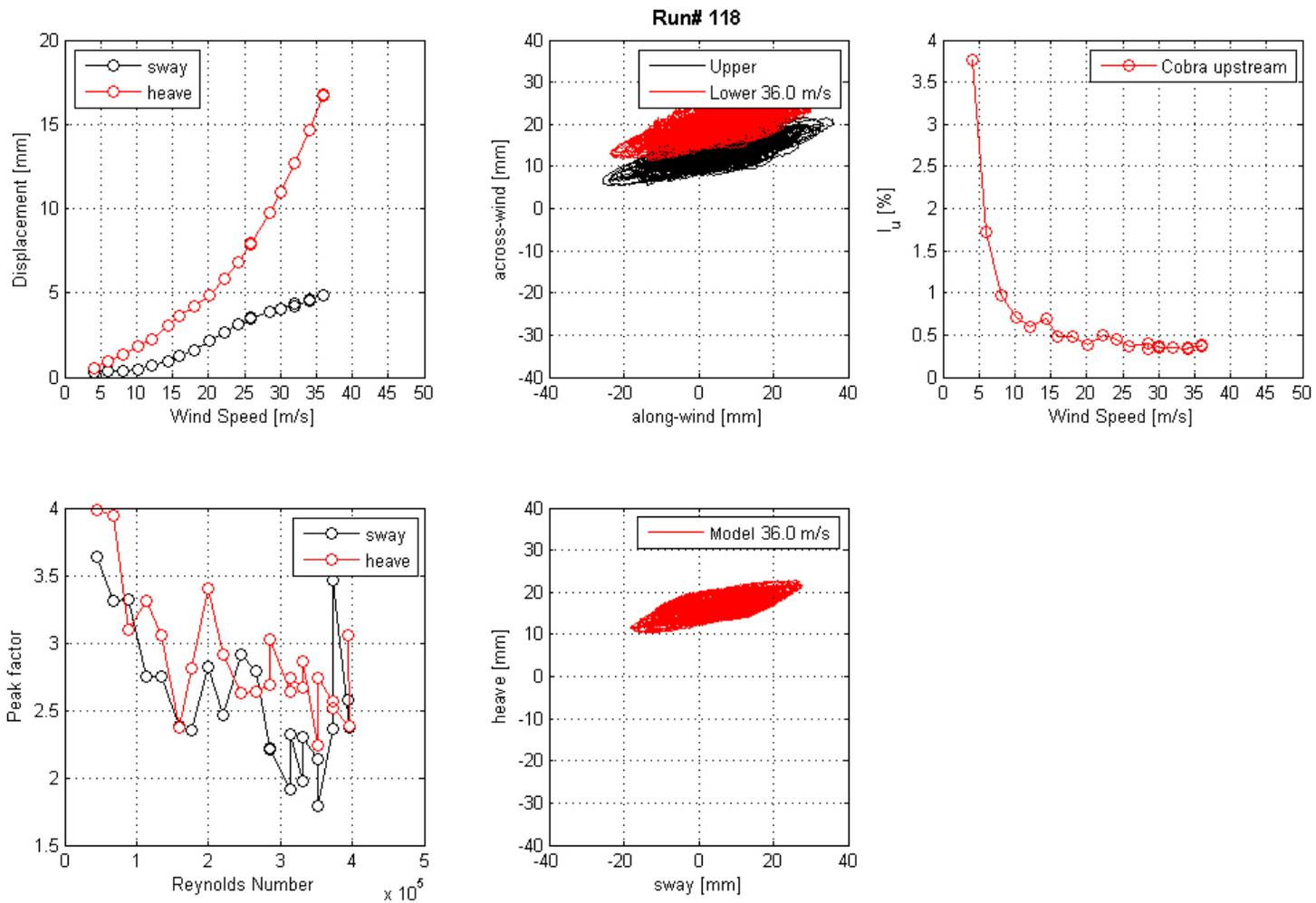
**Figure 105. Graph. Mean displacement and peak factor from the laser, motion path at one wind speed, and intensity of turbulence measured at the entrance of the test section for run 118.**
