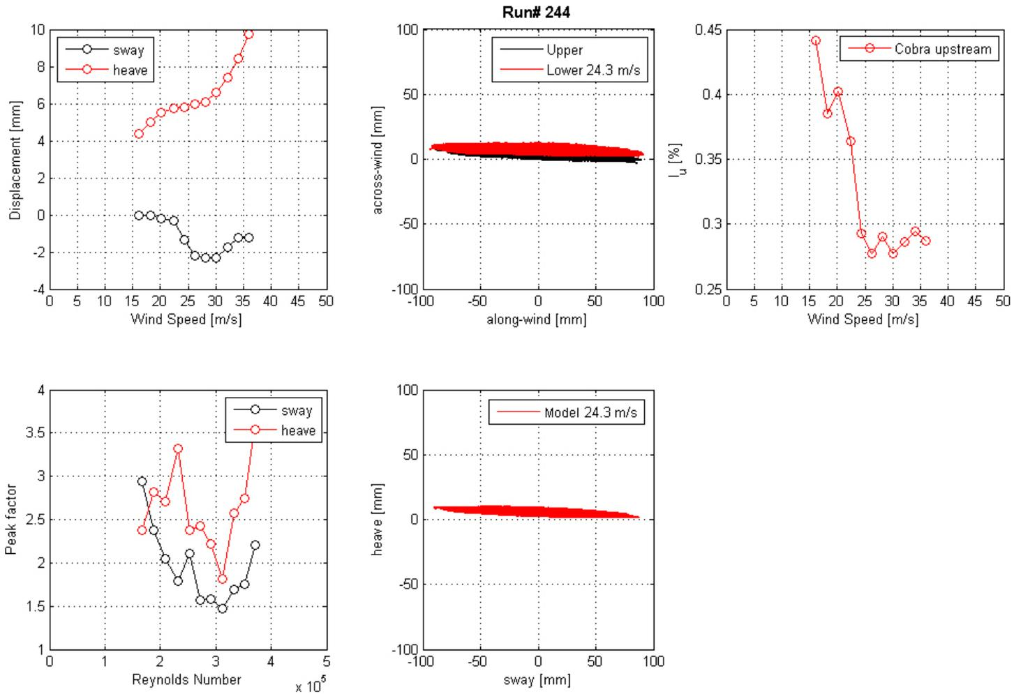
**Figure 173. Graph. Mean displacement and peak factor from the laser, motion path at one wind speed, and intensity of turbulence measured at the entrance of the test section for run 244.**
