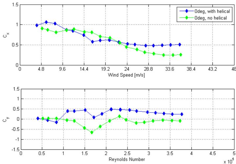
**Figure 45. Graph. Mean force coefficients for cable rotated at 0 degrees and inclined at 60 degrees in smooth flow with and without helical fillet.**
