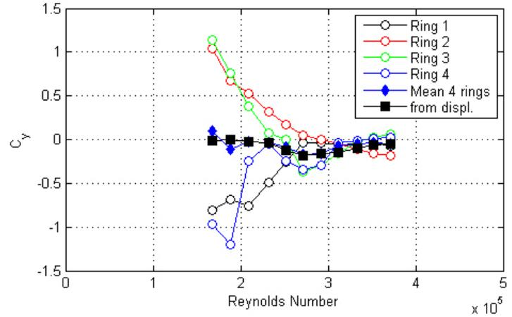
Figure 172. Graph. Response of the cable as a function of wind speed or Reynolds number as measured by the lasers, accelerometers, and surface pressures for run 244.
