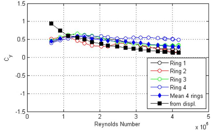
Figure 116. Graph. Response of the cable as a function of wind speed or Reynolds number as measured by the lasers, accelerometers, and surface pressures for run 137.
