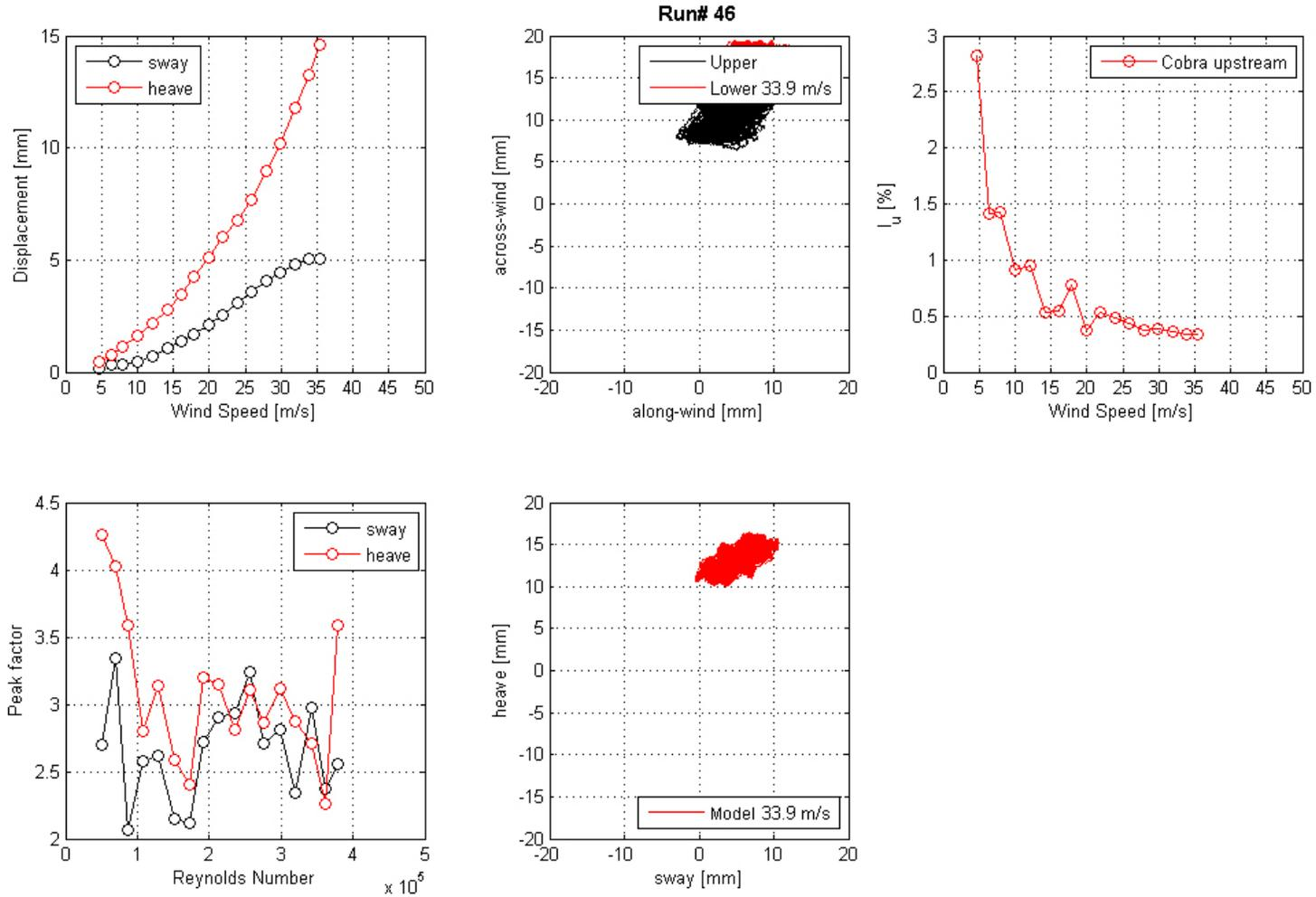
**Figure 71. Graph. Mean displacement and peak factor from the laser, motion path at one wind speed, and intensity of turbulence measured at the entrance of the test section for run 46.**
