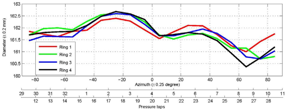
**Figure 4. Graph. Variations of the cable model diameter with azimuth at four span-wise locations.**
