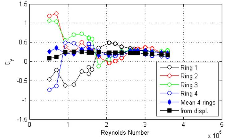
Figure 134. Graph. Response of the cable as a function of wind speed or Reynolds number as measured by the lasers, accelerometers, and surface pressures for run 167.
