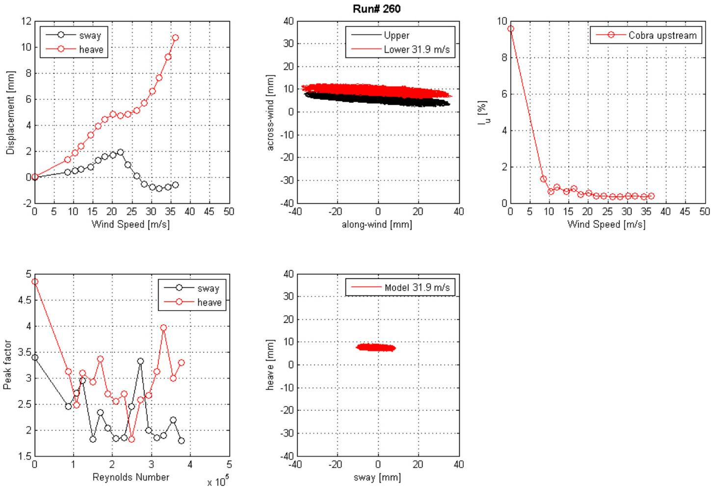
**Figure 183. Graph. Mean displacement and peak factor from the laser, motion path at one wind speed, and intensity of turbulence measured at the entrance of the test section for run 260.**
