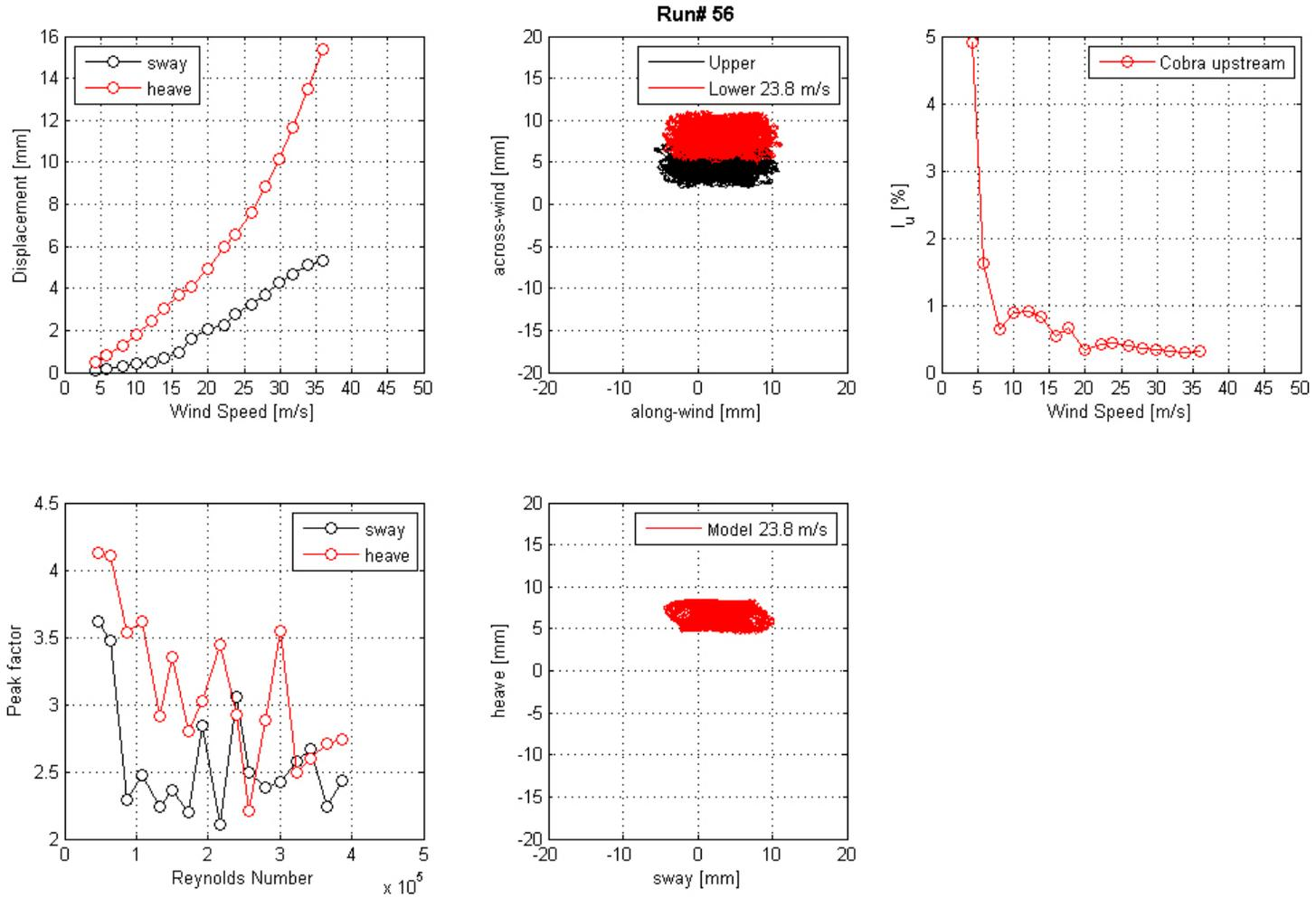
**Figure 77. Graph. Mean displacement and peak factor from the laser, motion path at one wind speed, and intensity of turbulence measured at the entrance of the test section for run 56.**
