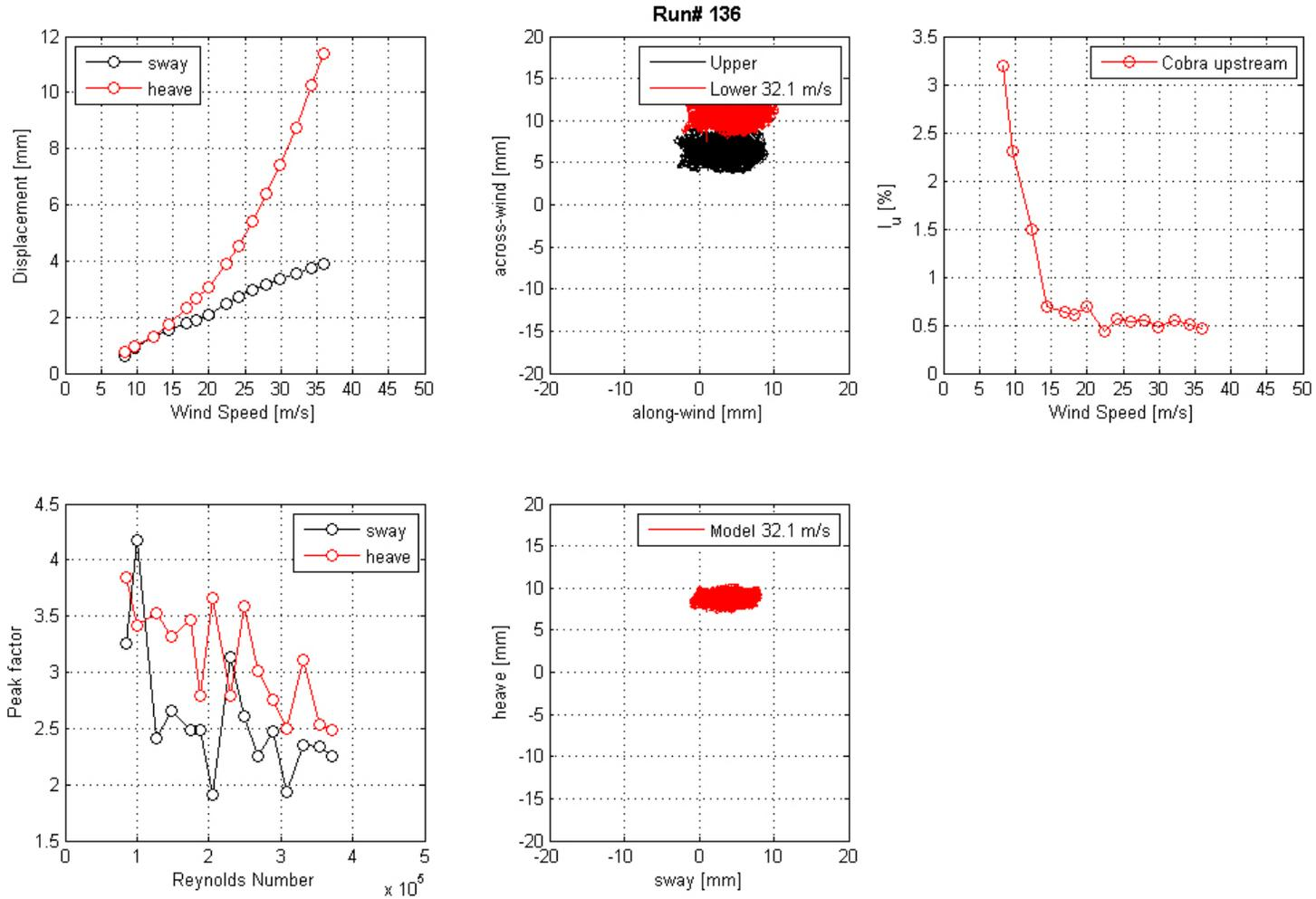
**Figure 115. Graph. Mean displacement and peak factor from the laser, motion path at one wind speed, and intensity of turbulence measured at the entrance of the test section for run 136.**
