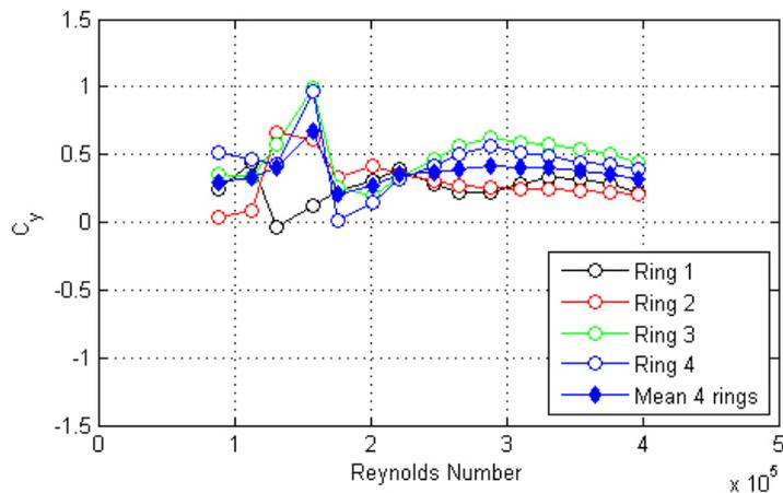
Figure 67. Graph. Intensity of turbulence measured at the entrance of the test section and  $C_x$  and  $C_y$  calculated from surface pressure measurements as a function of Reynolds number and wind speed for run 41.
