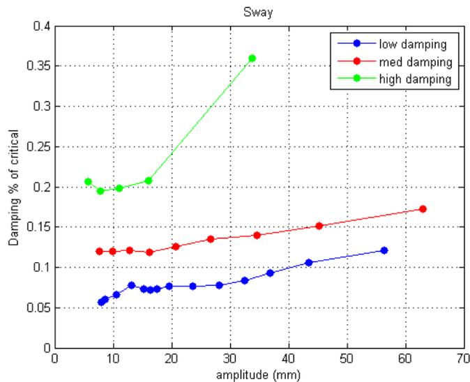
**Figure 36. Graph. Structural damping level as a function of amplitude of motion of the cable for the sway mode.**
