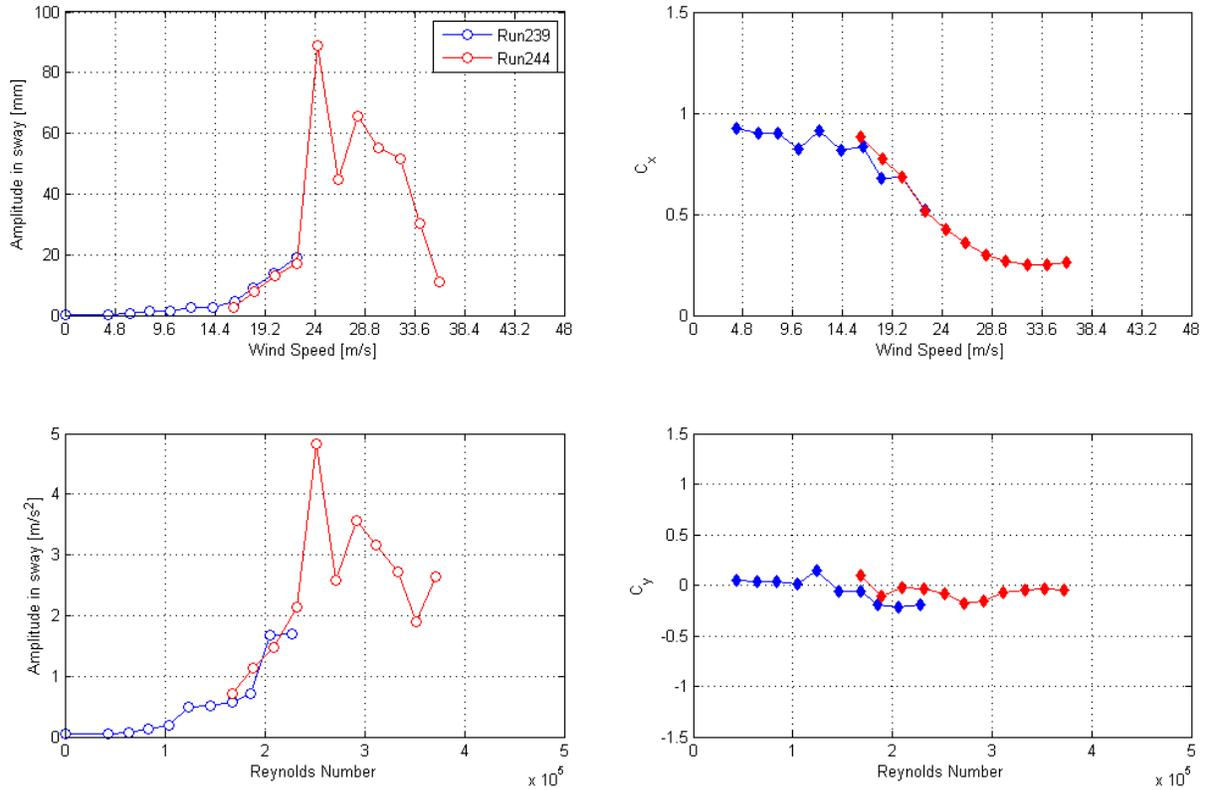
**Figure 57. Graph. Response of the cable for two consecutive runs for the cable inclined at 60 degrees and rotated at 2 degrees in smooth flow and without the helical fillet.**
