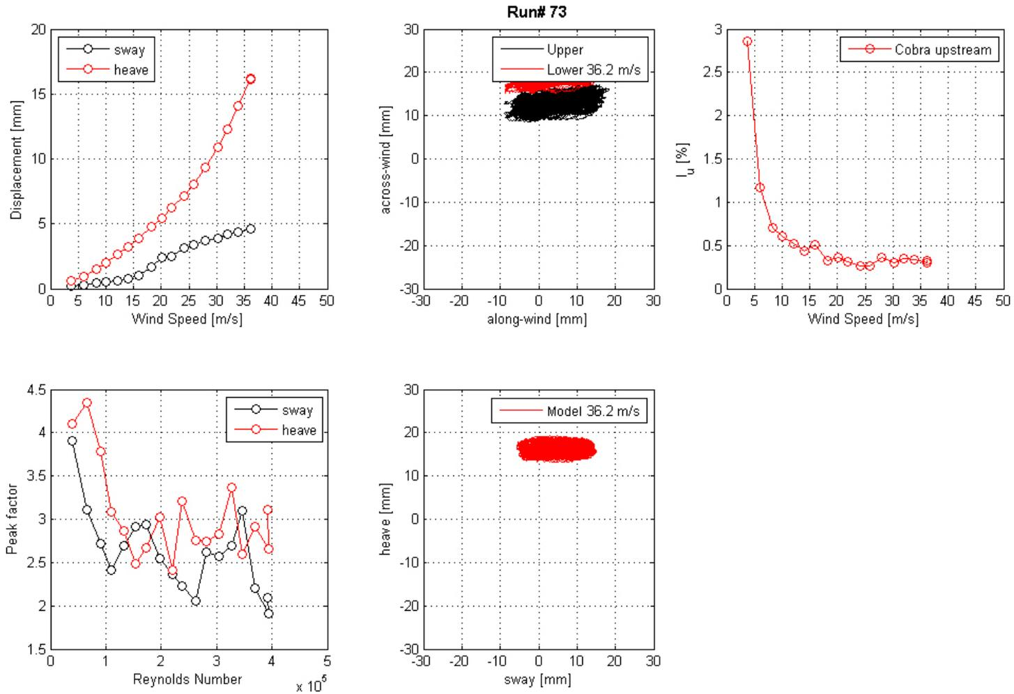
**Figure 91. Graph. Mean displacement and peak factor from the laser, motion path at one wind speed, and intensity of turbulence measured at the entrance of the test section for run 73.**
