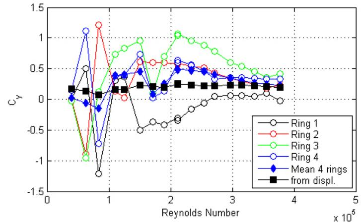
**Figure 59. Graph. Response of the cable as a function of wind speed or Reynolds number as measured by the lasers, accelerometers, and surface pressures for run 27.**
