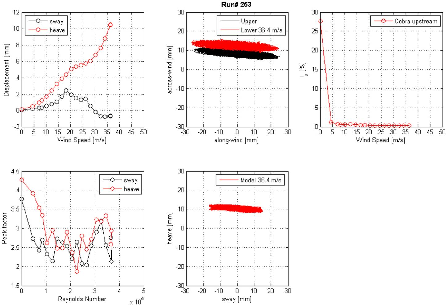
**Figure 177. Graph. Mean displacement and peak factor from the laser, motion path at one wind speed, and intensity of turbulence measured at the entrance of the test section for run 253.**
