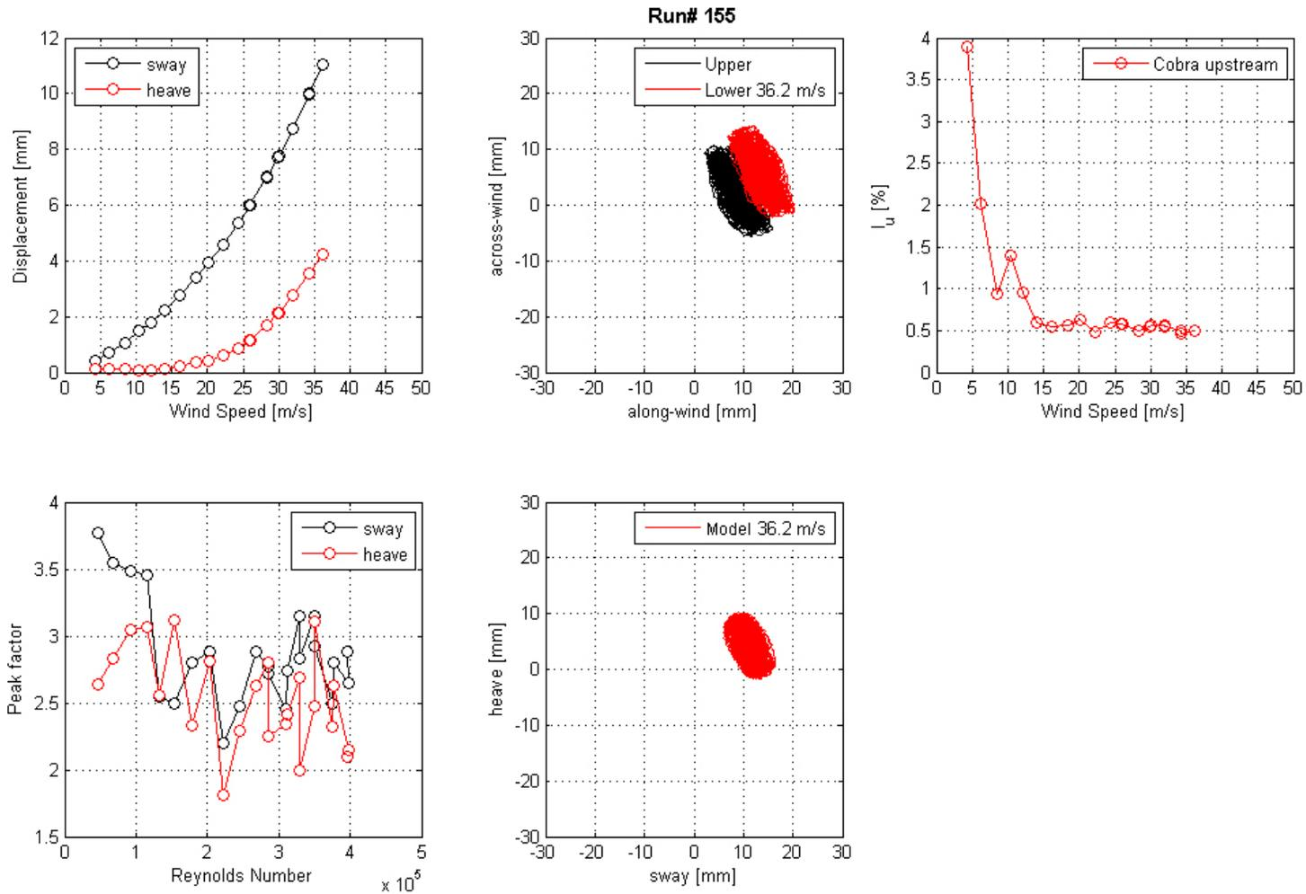
**Figure 129. Graph. Mean displacement and peak factor from the laser, motion path at one wind speed, and intensity of turbulence measured at the entrance of the test section for run 155.**
