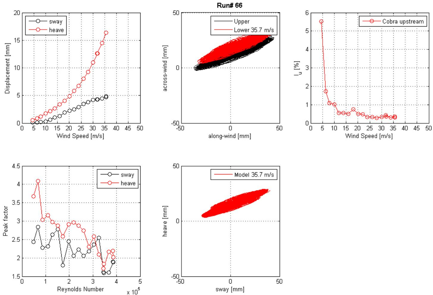
**Figure 83. Graph. Mean displacement and peak factor from the laser, motion path at one wind speed, and intensity of turbulence measured at the entrance of the test section for run 66.**
