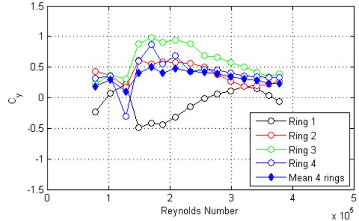
Figure 64. Graph. Intensity of turbulence measured at the entrance of the test section and  $C_x$  and  $C_y$  calculated from surface pressure measurements as a function of Reynolds number and wind speed for run 35.
