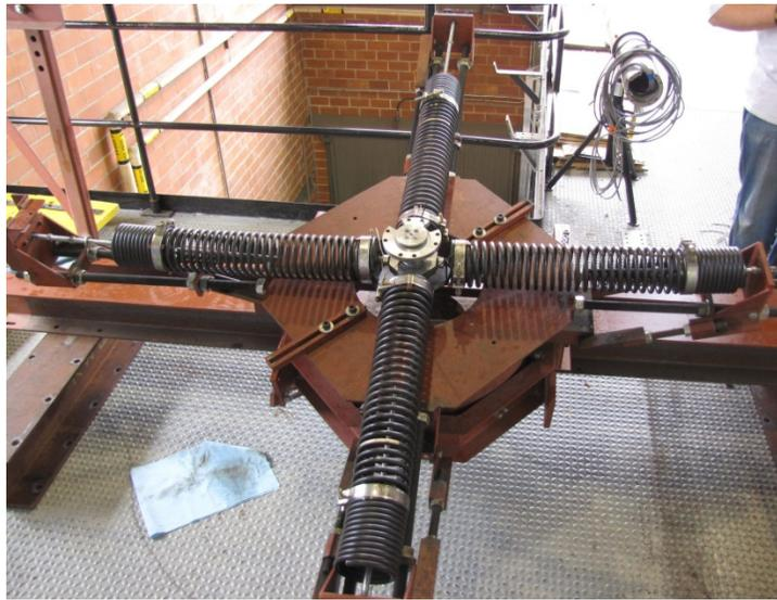
**Figure 7. Photo. Lower rig with spring rotation at 0 degrees.**
