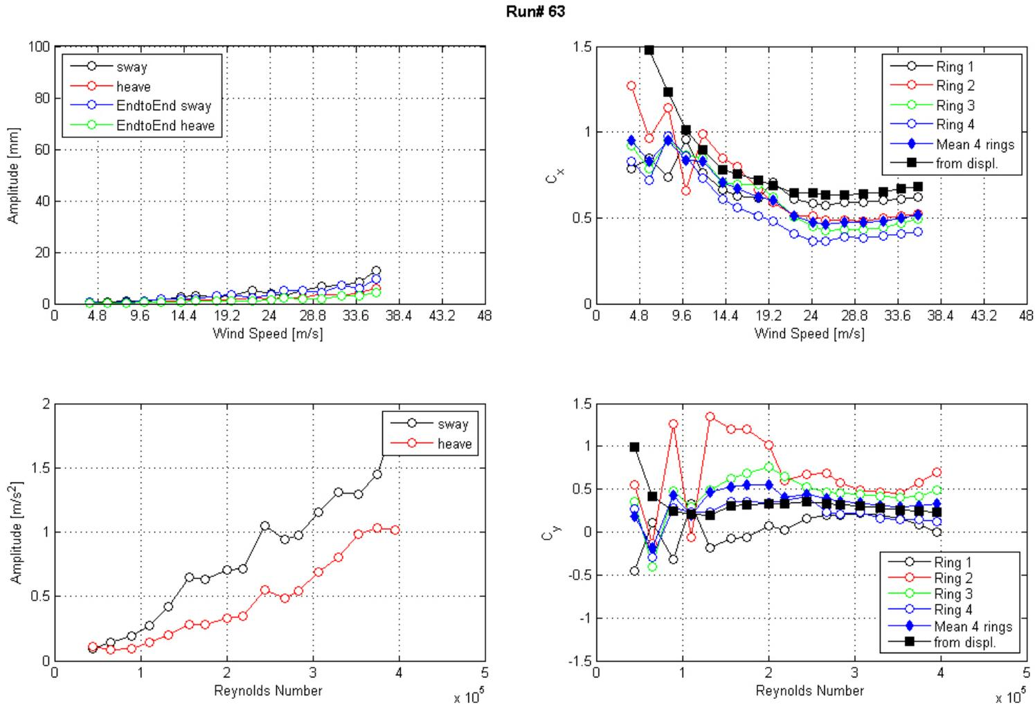
**Figure 80. Graph. Response of the cable as a function of wind speed or Reynolds number as measured by the lasers, accelerometers, and surface pressures for run 63.**
