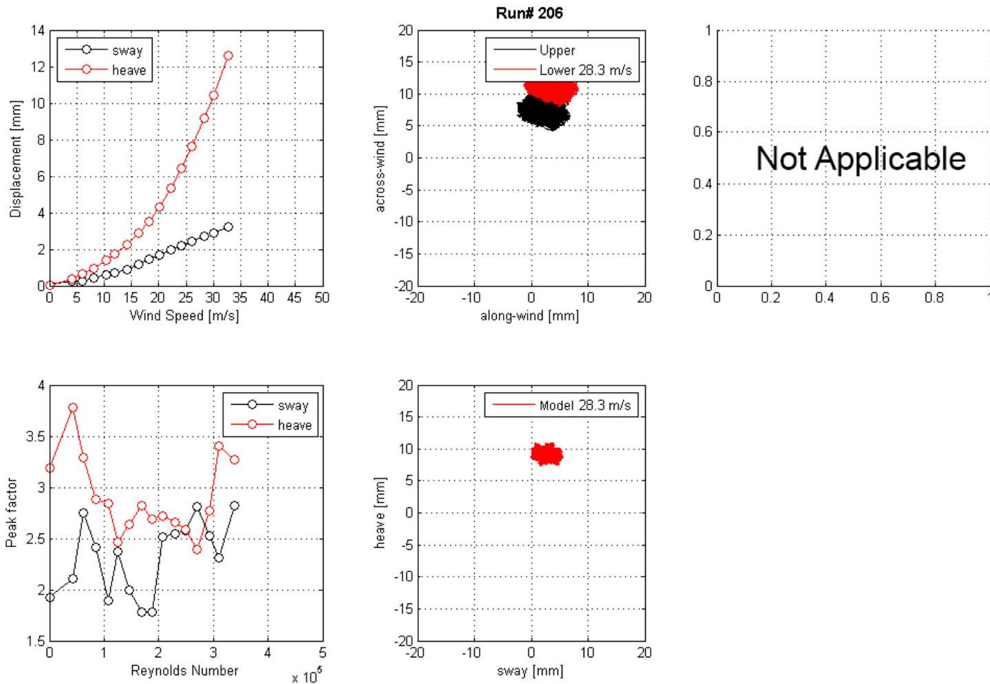
**Figure 147. Graph. Mean displacement and peak factor from the laser, motion path at one wind speed, and intensity of turbulence measured at the entrance of the test section for run 206.**
