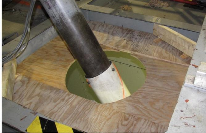
**Figure 12. Photo. Top of the open interface between the cable model and the roof of the wind tunnel.**
