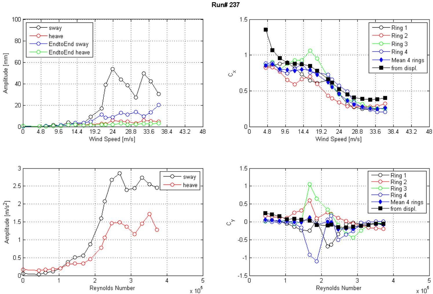
**Figure 168. Graph. Response of the cable as a function of wind speed or Reynolds number as measured by the lasers, accelerometers, and surface pressures for run 237.**
