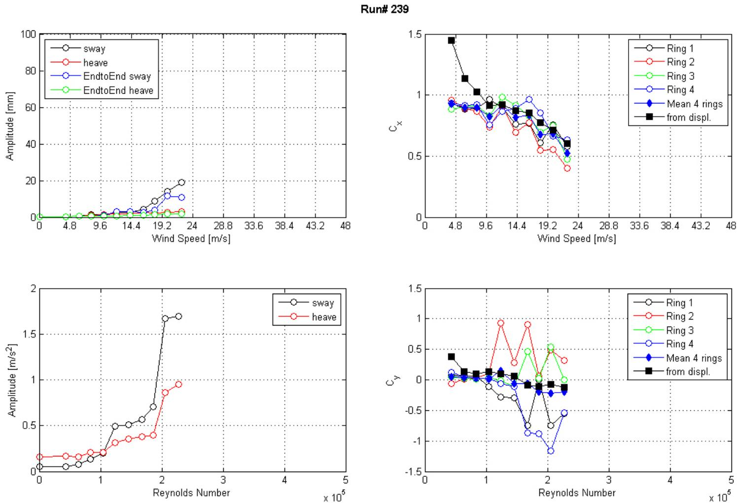
**Figure 170. Graph. Response of the cable as a function of wind speed or Reynolds number as measured by the lasers, accelerometers, and surface pressures for run 239.**
