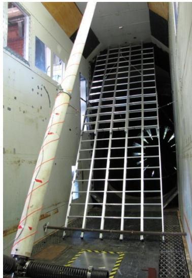
**Figure 16. Photo. Grid of ladders used to generate the turbulent flow field for position 1.**
