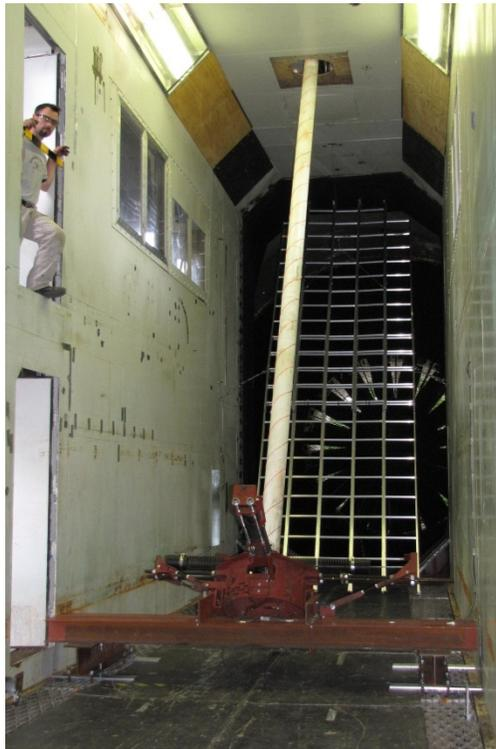
**Figure 39. Photo. Cable model at 60-degree inclination and 0-degree spring rotation in turbulent flow.**
