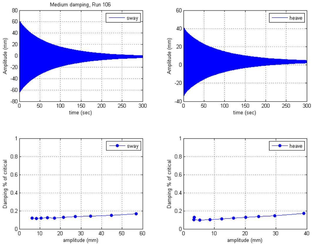
**Figure 185. Graph. Damping traces and level for the sway and heave modes for the medium damping case.**
