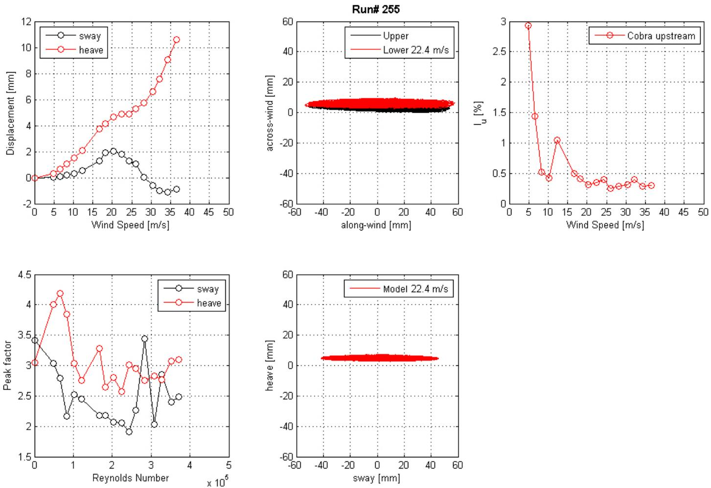
**Figure 179. Graph. Mean displacement and peak factor from the laser, motion path at one wind speed, and intensity of turbulence measured at the entrance of the test section for run 255.**
