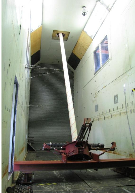
**Figure 10. Photo. Cable model at an inclination of 60 degrees from inside the test section of the 3-by-6-m Propulsion and Icing Wind Tunnel.**
