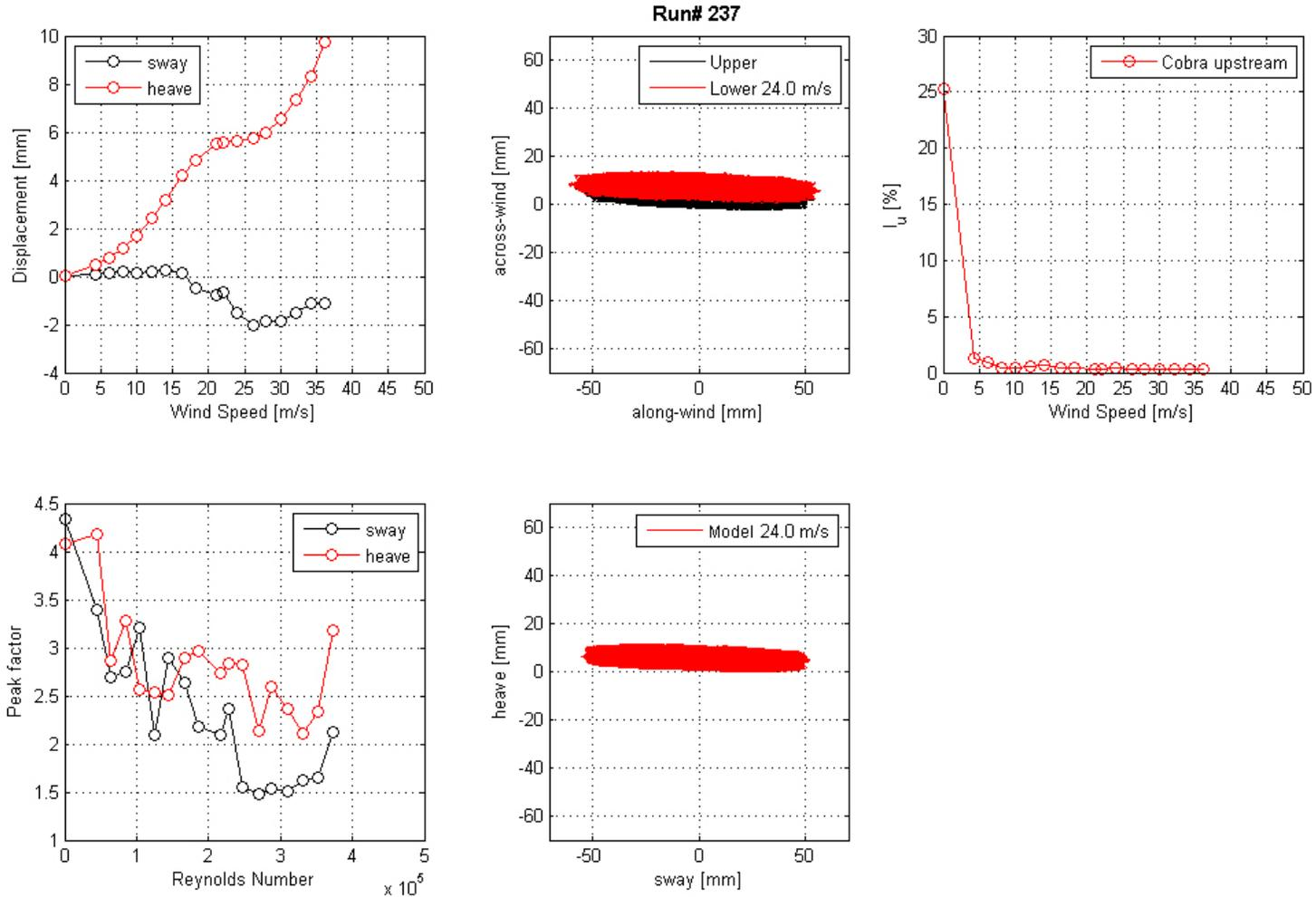
**Figure 169. Graph. Mean displacement and peak factor from the laser, motion path at one wind speed, and intensity of turbulence measured at the entrance of the test section for run 237.**
