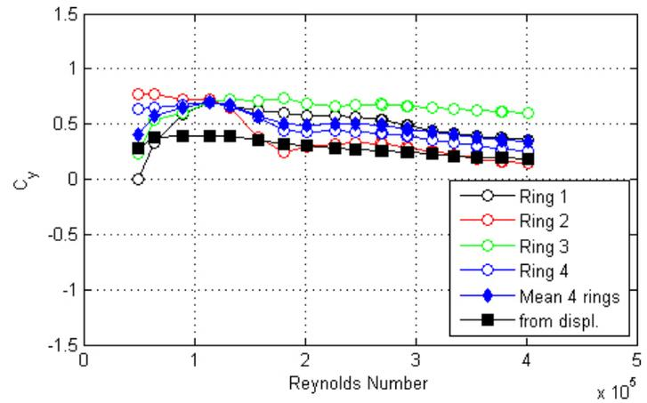
Figure 124. Graph. Response of the cable as a function of wind speed or Reynolds number as measured by the lasers, accelerometers, and surface pressures for run 149.
