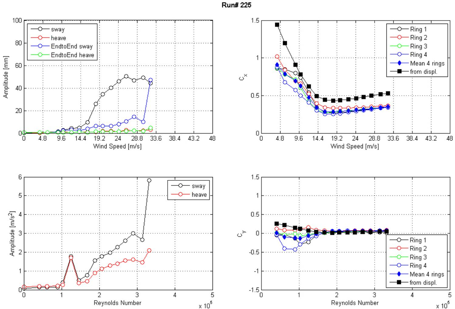
**Figure 160. Graph. Response of the cable as a function of wind speed or Reynolds number as measured by the lasers, accelerometers, and surface pressures for run 225.**
