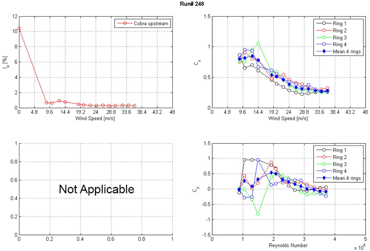
**Figure 174. Graph. Intensity of turbulence measured at the entrance of the test section and  $C_x$  and  $C_y$  calculated from surface pressure measurements as a function of Reynolds number and wind speed for run 248.**
