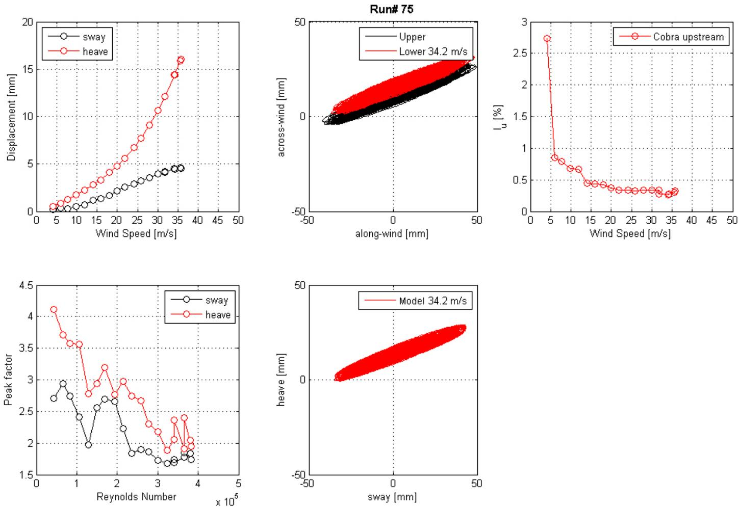
**Figure 93. Graph. Mean displacement and peak factor from the laser, motion path at one wind speed, and intensity of turbulence measured at the entrance of the test section for run 75.**
