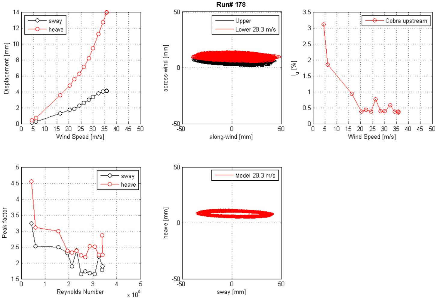
**Figure 139. Graph. Mean displacement and peak factor from the laser, motion path at one wind speed, and intensity of turbulence measured at the entrance of the test section for run 178.**
