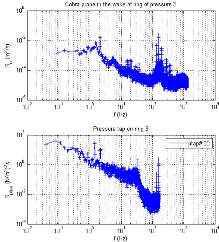
**Figure 50. Graph. Spectrum of the longitudinal flow velocity fluctuations located in the wake of the model and spectrum of the surface pressure signal of port 30 on ring 3 with a wind speed of 24 m/s.**
