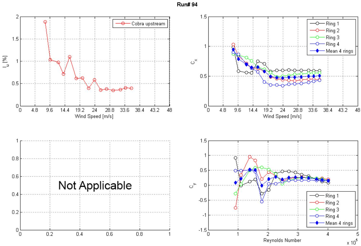
**Figure 99. Graph. Intensity of turbulence measured at the entrance of the test section and  $C_x$  and  $C_y$  calculated from surface pressure measurements as a function of Reynolds number and wind speed for run 94.**
