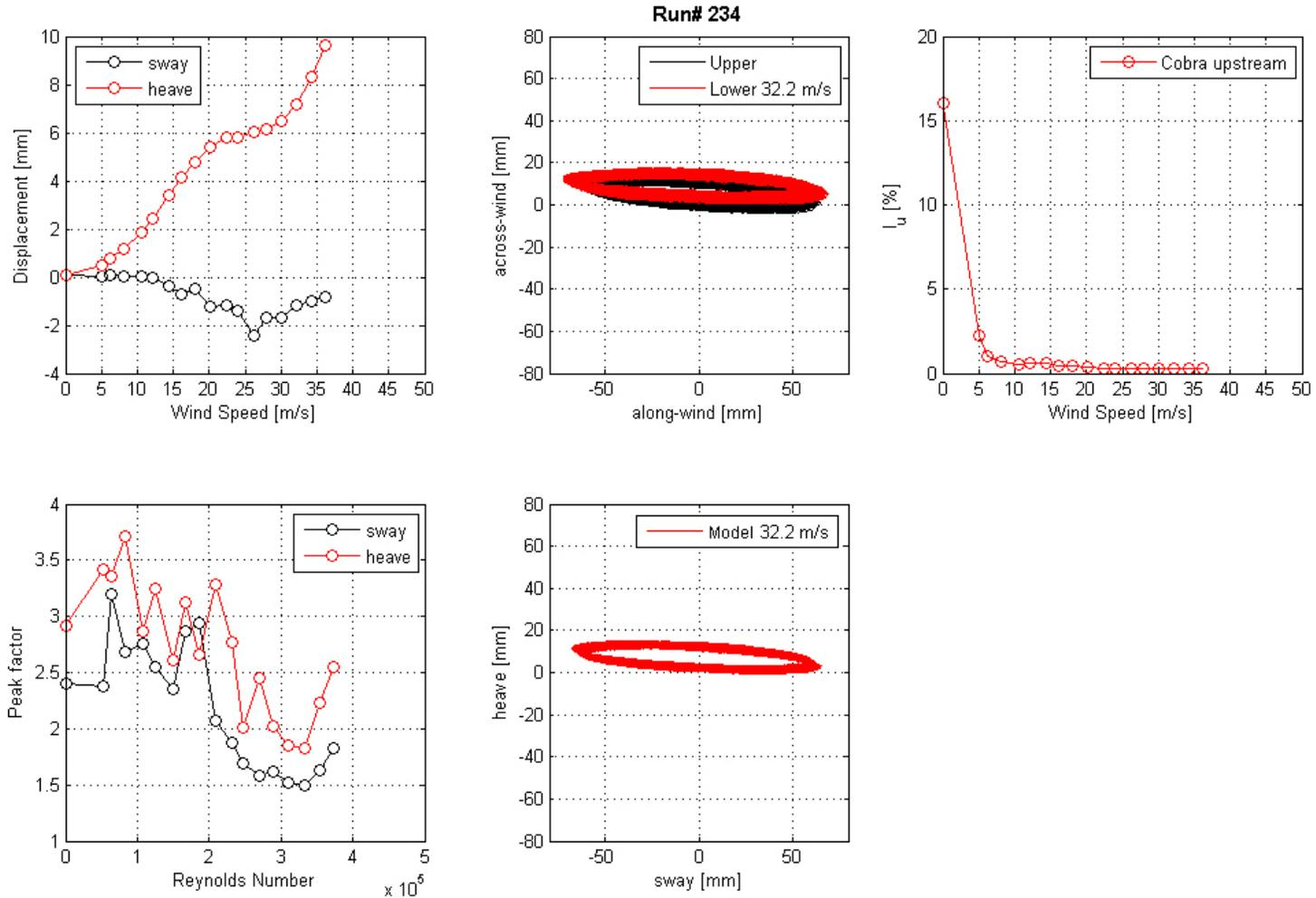
**Figure 167. Graph. Mean displacement and peak factor from the laser, motion path at one wind speed, and intensity of turbulence measured at the entrance of the test section for run 234.**
