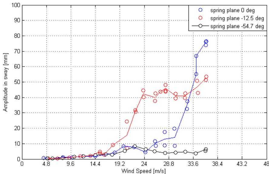
**Figure 30. Graph. Amplitude of motion in sway for three different spring plane rotations for the cable inclined at 60 degrees with helical fillet and in smooth flow.**
