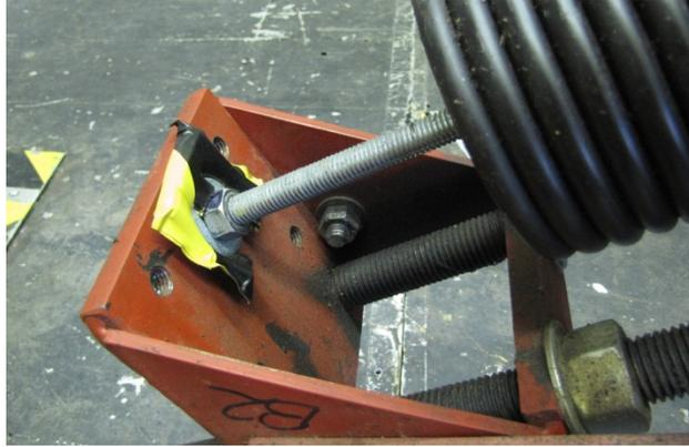
**Figure 35. Photo. Viscoelastic washer used to increase the structural damping of the suspension system.**
