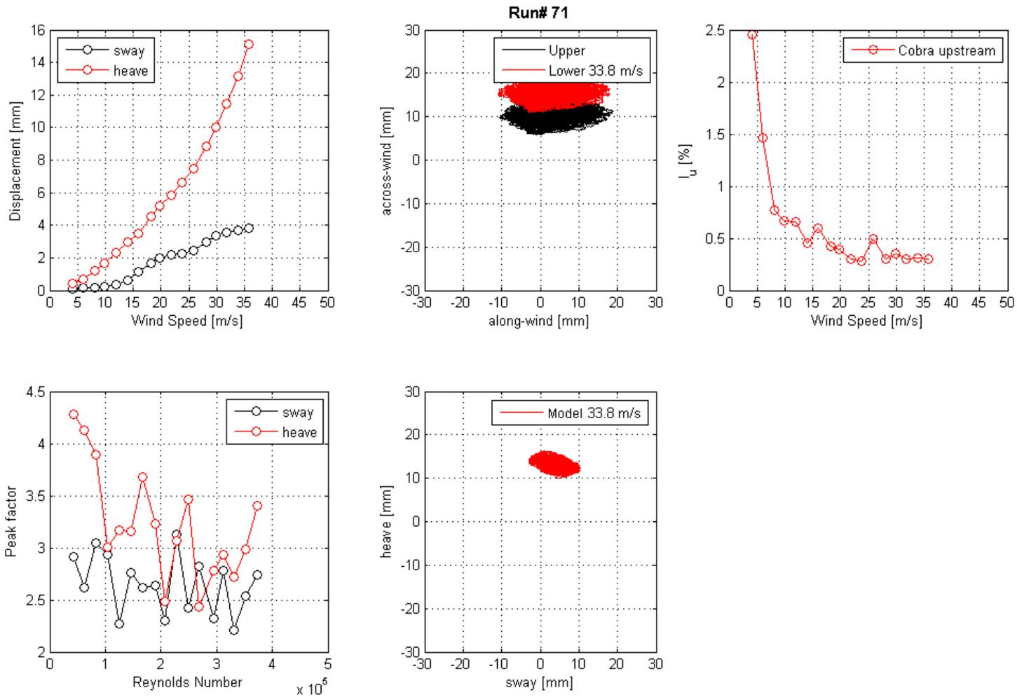
**Figure 89. Graph. Mean displacement and peak factor from the laser, motion path at one wind speed, and intensity of turbulence measured at the entrance of the test section for run 71.**
