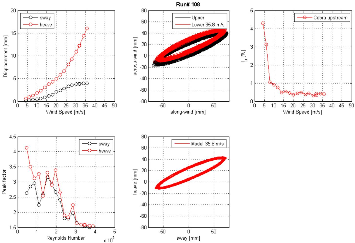
**Figure 103. Graph. Mean displacement and peak factor from the laser, motion path at one wind speed, and intensity of turbulence measured at the entrance of the test section for run 108.**
