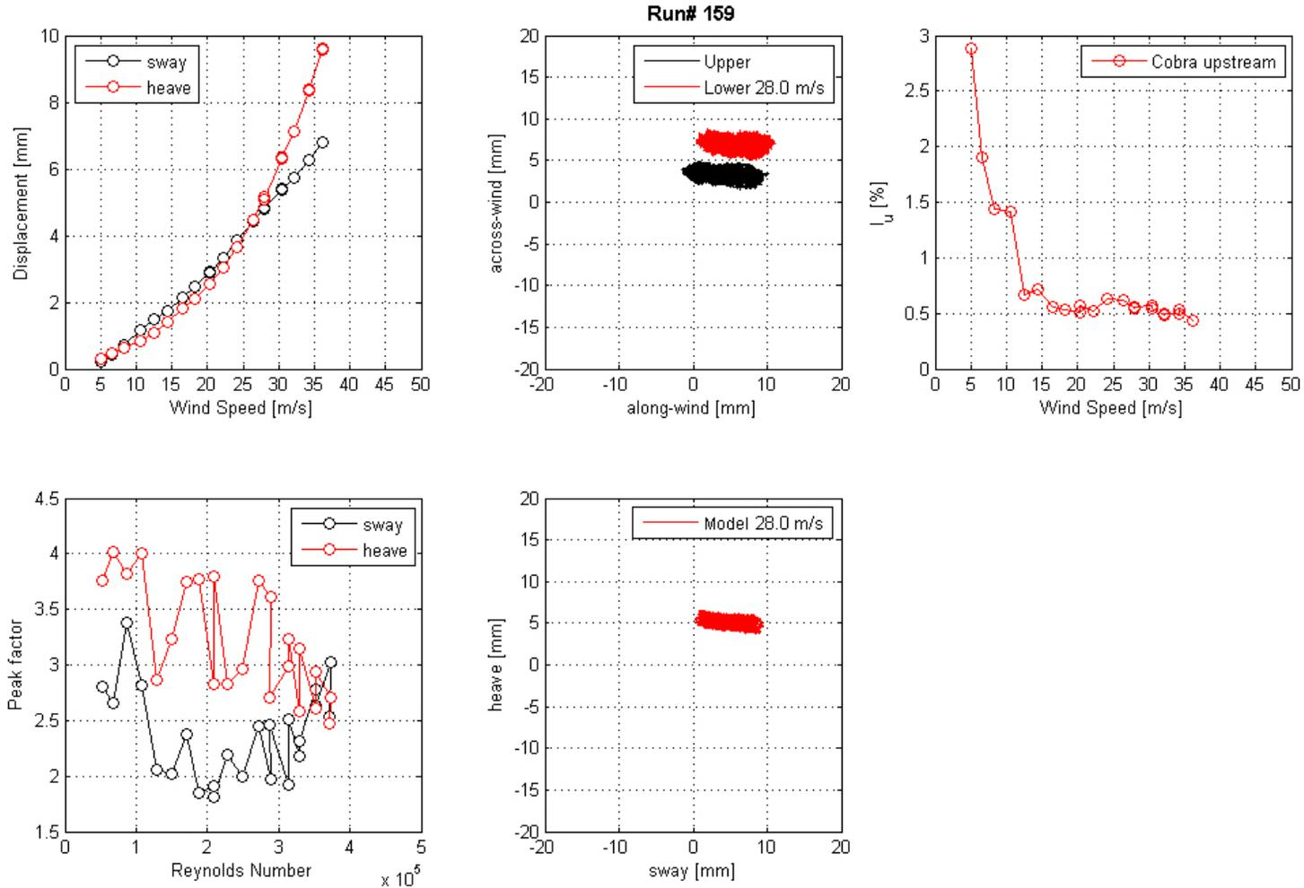
**Figure 131. Graph. Mean displacement and peak factor from the laser, motion path at one wind speed, and intensity of turbulence measured at the entrance of the test section for run 159.**
