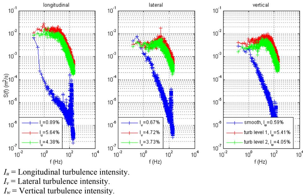
**Figure 19. Graph. Variations of the normalized spectral densities of the wind velocity fluctuations with frequencies for the smooth and turbulent flow cases.**
