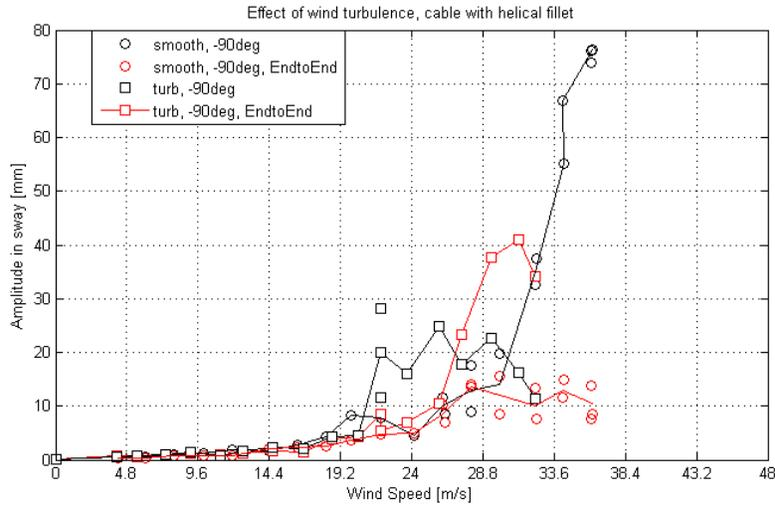
**Figure 40. Graph. Amplitude of motion in sway and end-to-end sway at cable rotation of -90 degrees and inclined at 60 degrees with a helical fillet in smooth and turbulent flow.**
