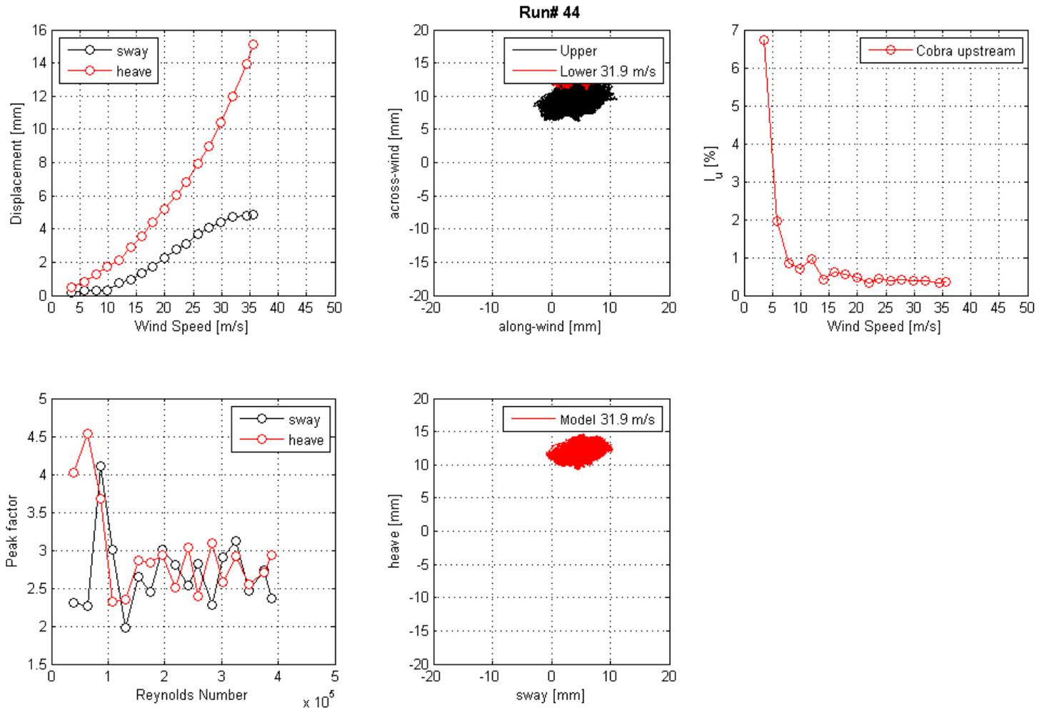
**Figure 69. Graph. Mean displacement and peak factor from the laser, motion path at one wind speed, and intensity of turbulence measured at the entrance of the test section for run 44.**
