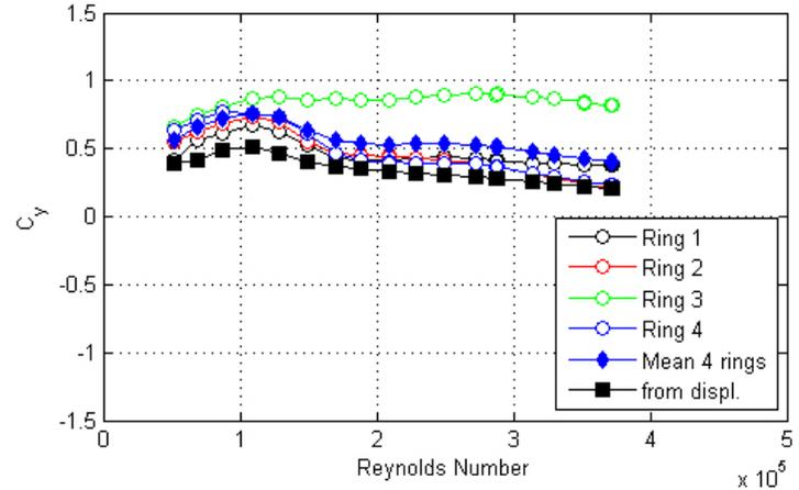
Figure 130. Graph. Response of the cable as a function of wind speed or Reynolds number as measured by the lasers, accelerometers, and surface pressures for run 159.
