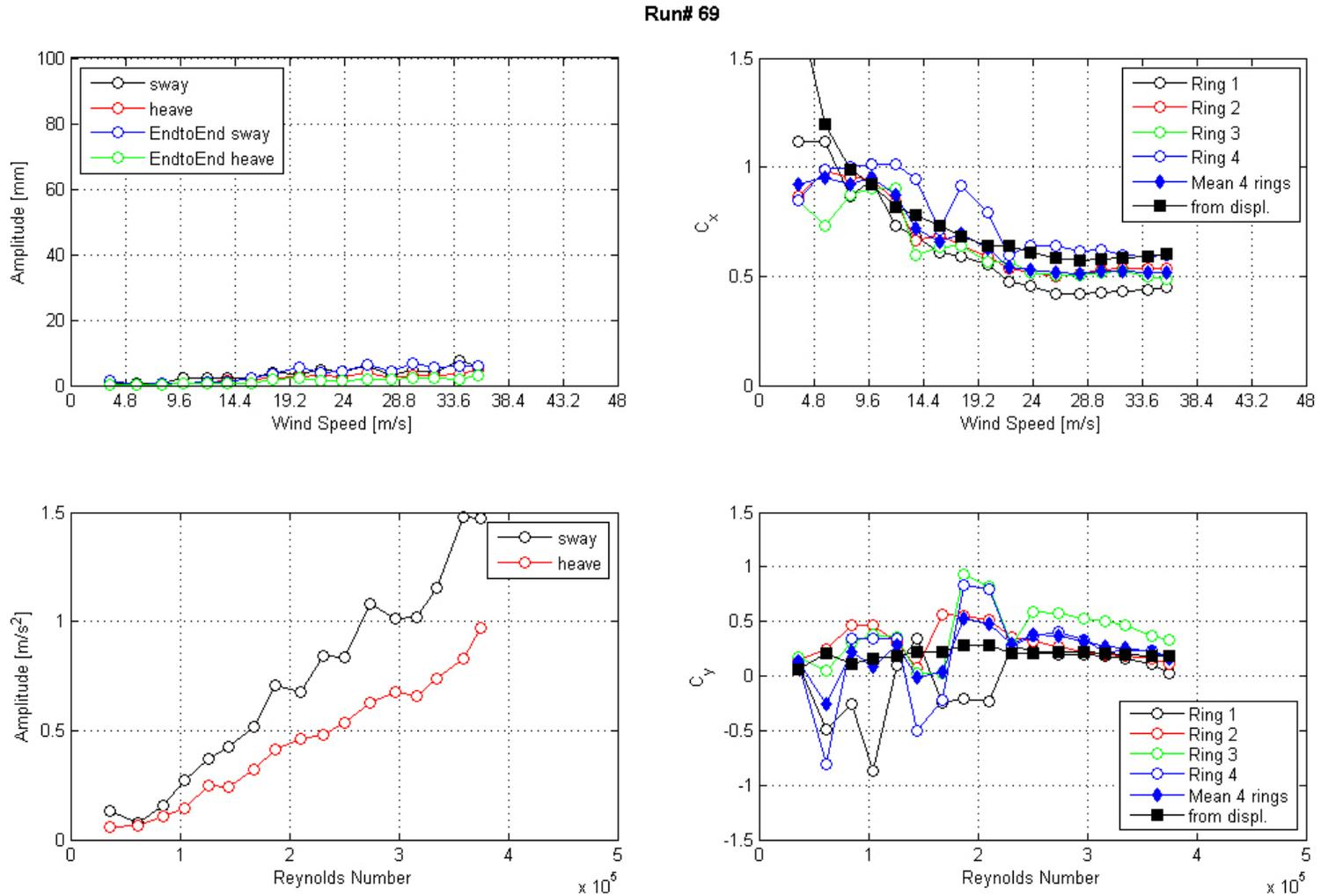
**Figure 86. Graph. Response of the cable as a function of wind speed or Reynolds number as measured by the lasers, accelerometers, and surface pressures for run 69.**
