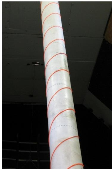
**Figure 6. Photo. Overview of double helical right-handed fillet.**
