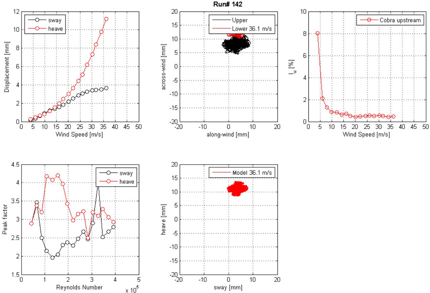
**Figure 121. Graph. Mean displacement and peak factor from the laser, motion path at one wind speed, and intensity of turbulence measured at the entrance of the test section for run 142.**
