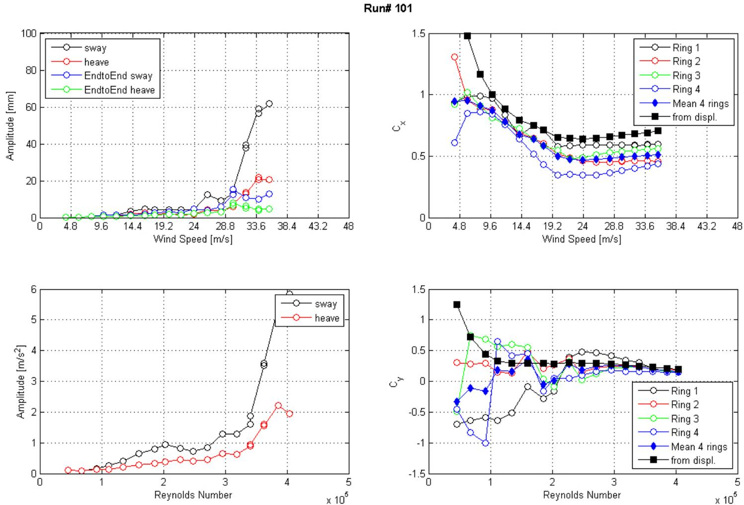
**Figure 100. Graph. Response of the cable as a function of wind speed or Reynolds number as measured by the lasers, accelerometers, and surface pressures for run 101.**
