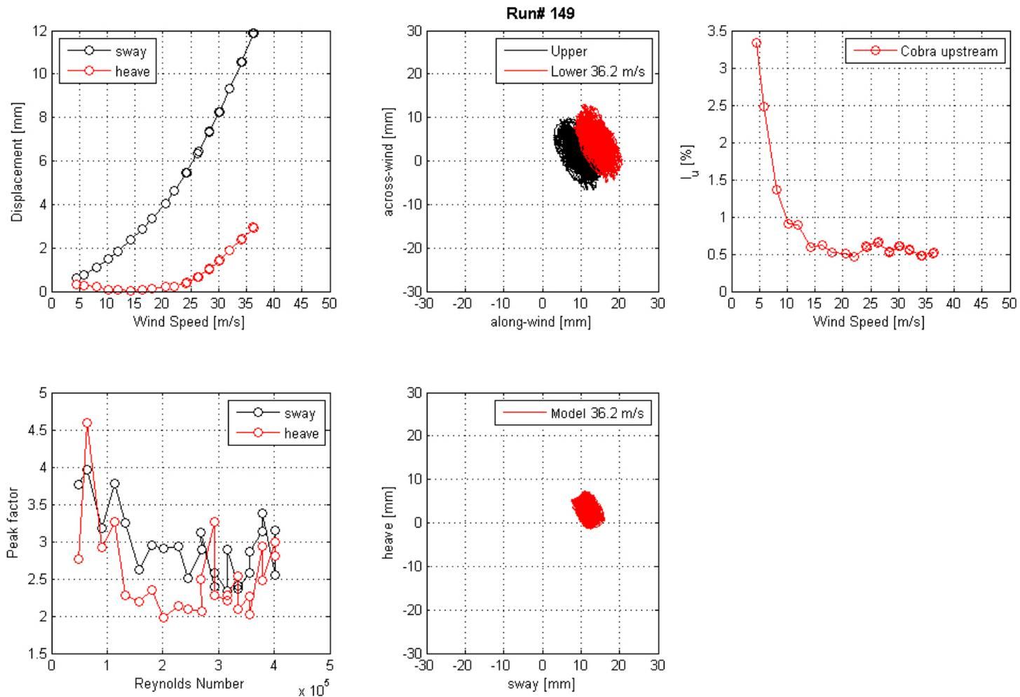
**Figure 125. Graph. Mean displacement and peak factor from the laser, motion path at one wind speed, and intensity of turbulence measured at the entrance of the test section for run 149.**
