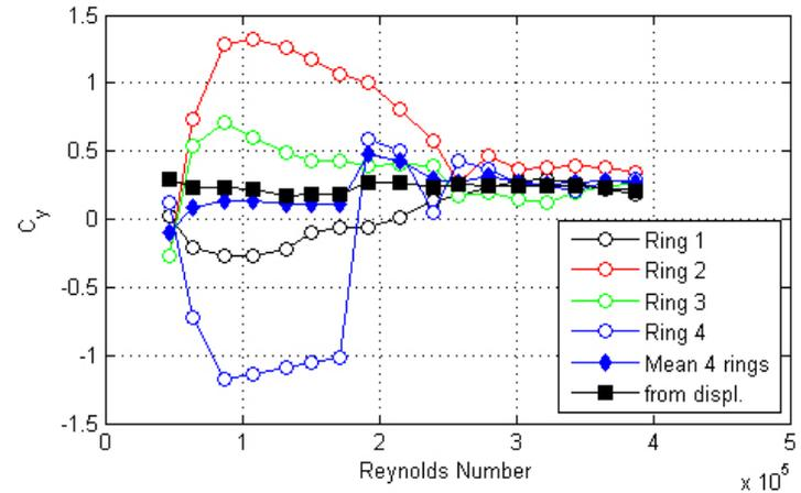
Figure 76. Graph. Response of the cable as a function of wind speed or Reynolds number as measured by the lasers, accelerometers, and surface pressures for run 56.
