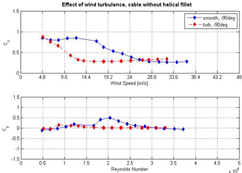
**Figure 43. Graph. Mean force coefficients at cable rotation of -90 degrees and inclined at 60 degrees without a helical fillet in smooth and turbulent flow.**
