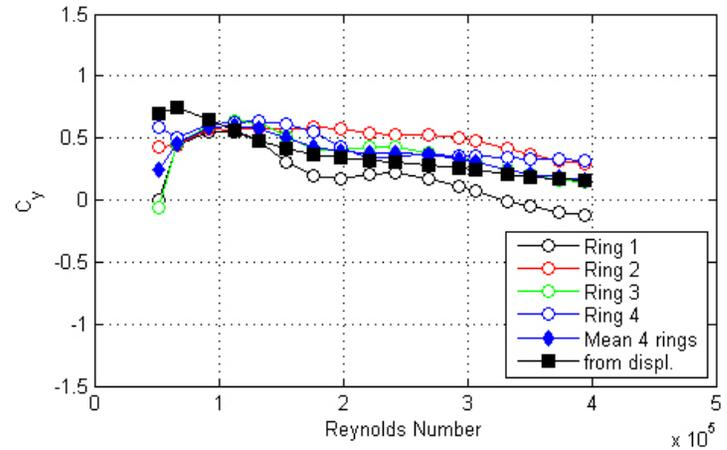
Figure 118. Graph. Response of the cable as a function of wind speed or Reynolds number as measured by the lasers, accelerometers, and surface pressures for run 140.
