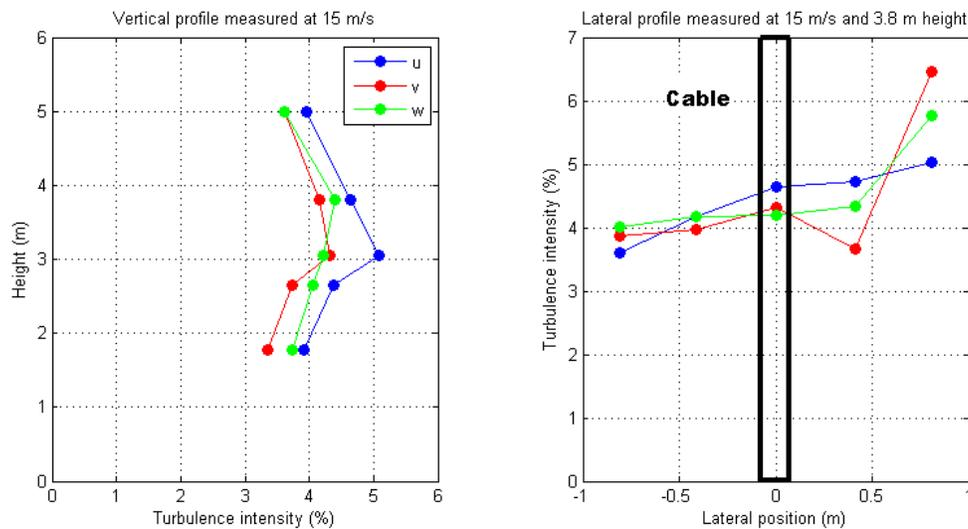
**Figure 20. Graph. Vertical and lateral profiles of the intensity of turbulence for the three wind components for the turbulent flow for position 2.**
