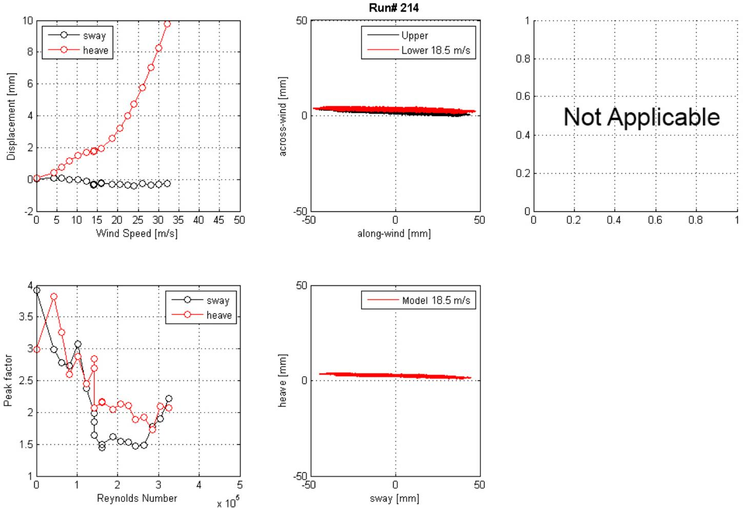
**Figure 153. Graph. Mean displacement and peak factor from the laser, motion path at one wind speed, and intensity of turbulence measured at the entrance of the test section for run 214.**
