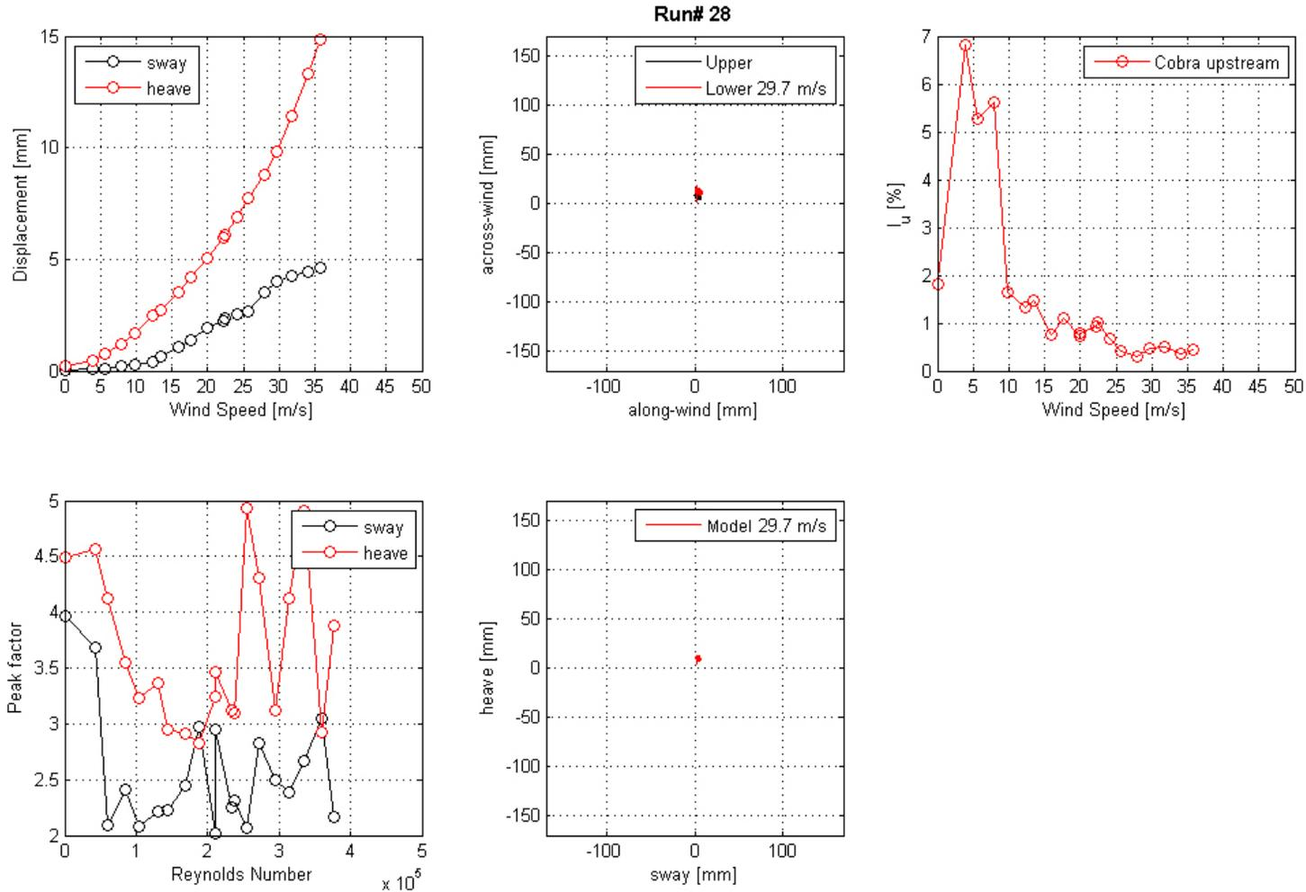
**Figure 62. Graph. Mean displacement and peak factor from the laser, motion path at one wind speed, and intensity of turbulence measured at the entrance of the test section for run 28.**
