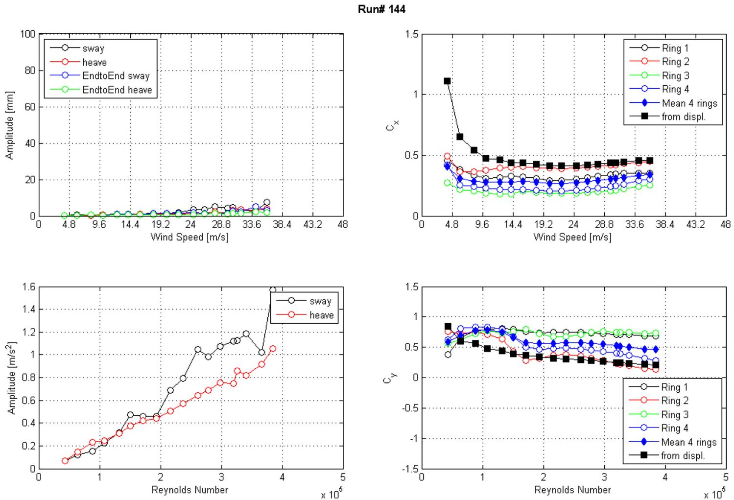
**Figure 122. Graph. Response of the cable as a function of wind speed or Reynolds number as measured by the lasers, accelerometers, and surface pressures for run 144.**
