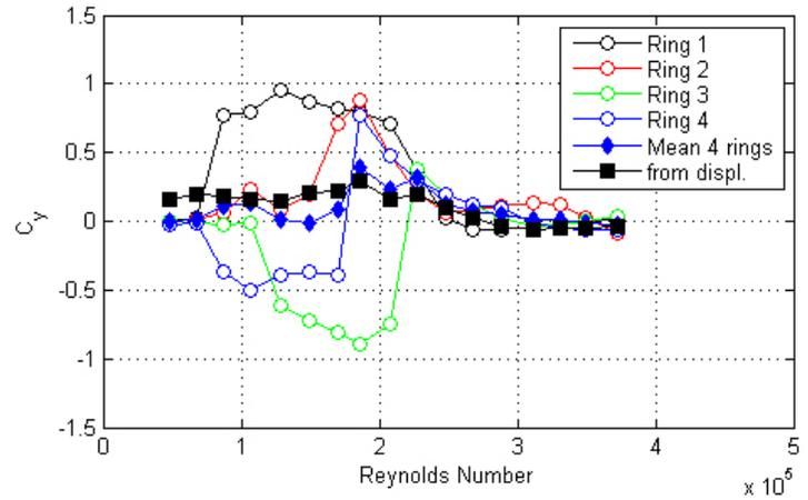
Figure 180. Graph. Response of the cable as a function of wind speed or Reynolds number as measured by the lasers, accelerometers, and surface pressures for run 257.
