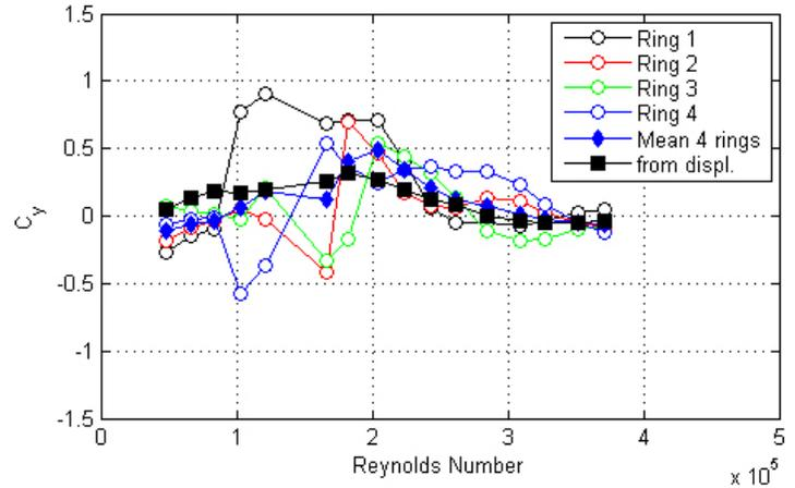
Figure 178. Graph. Response of the cable as a function of wind speed or Reynolds number as measured by the lasers, accelerometers, and surface pressures for run 255.
