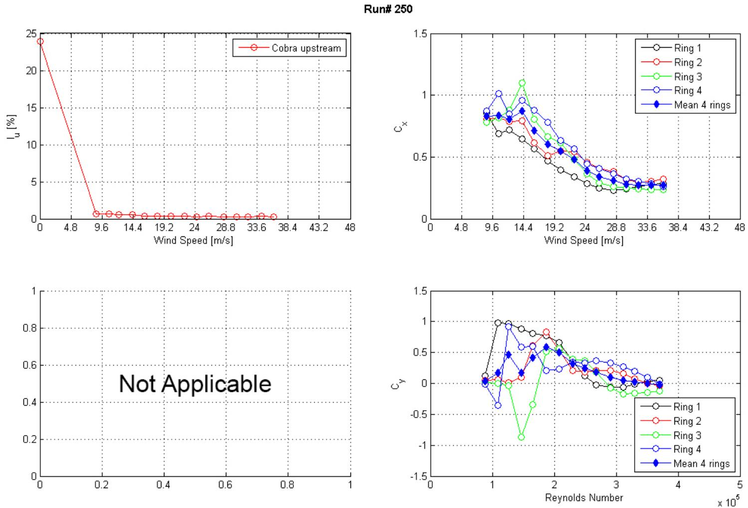
**Figure 175. Graph. Intensity of turbulence measured at the entrance of the test section and  $C_x$  and  $C_y$  calculated from surface pressure measurements as a function of Reynolds number and wind speed for run 250.**
