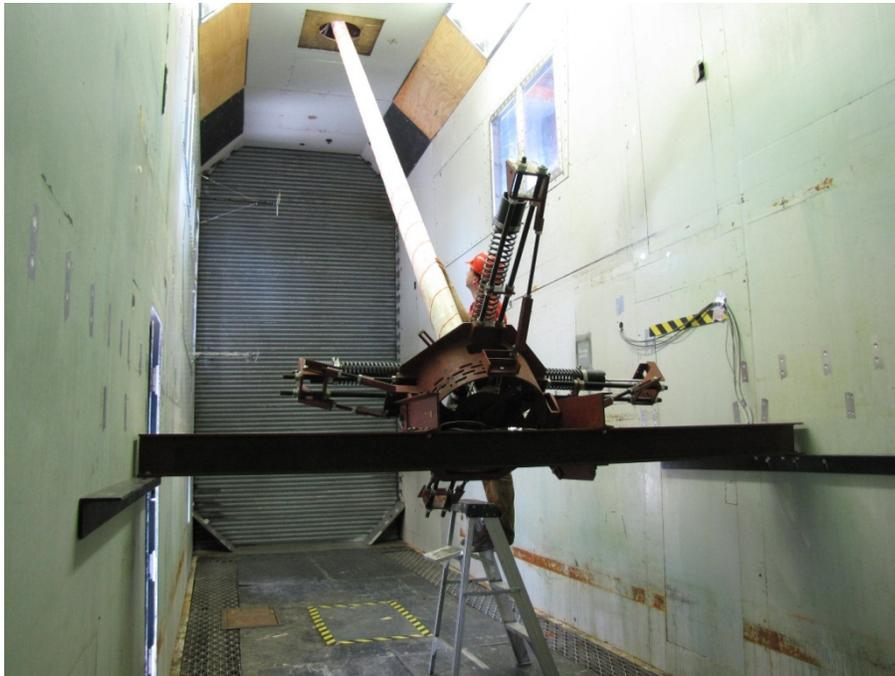
**Figure 31. Photo. Cable model at 45-degree inclination and 0-degree spring rotation with smooth flow.**
