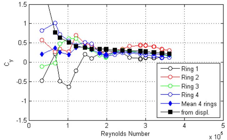
Figure 132. Graph. Response of the cable as a function of wind speed or Reynolds number as measured by the lasers, accelerometers, and surface pressures for run 163.
