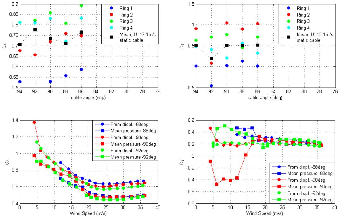
**Figure 48. Graph. Mean force coefficients as a function of cable rotation for the static cable and as a function of wind speed for cable in motion.**
