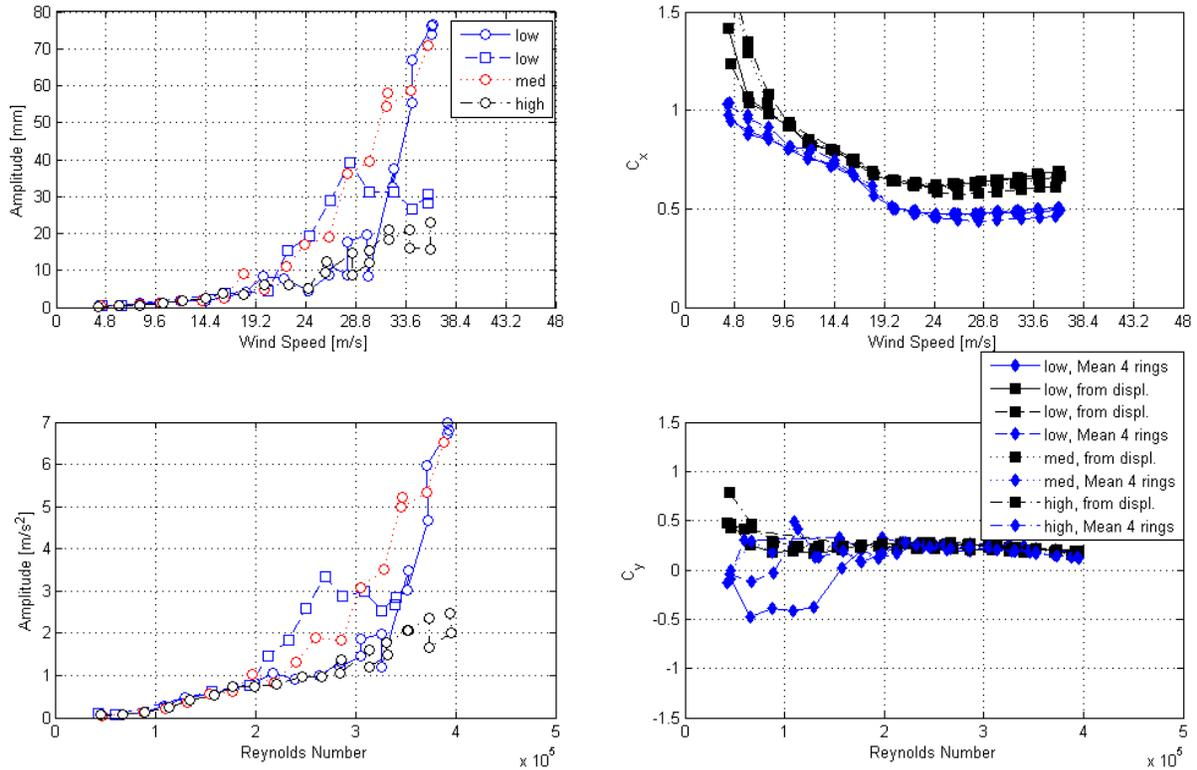
**Figure 38. Graph. Response of the cable model as a function of wind speed or Reynolds number for three damping levels as measured by lasers, accelerometers, and surface pressures for different levels of damping.**
