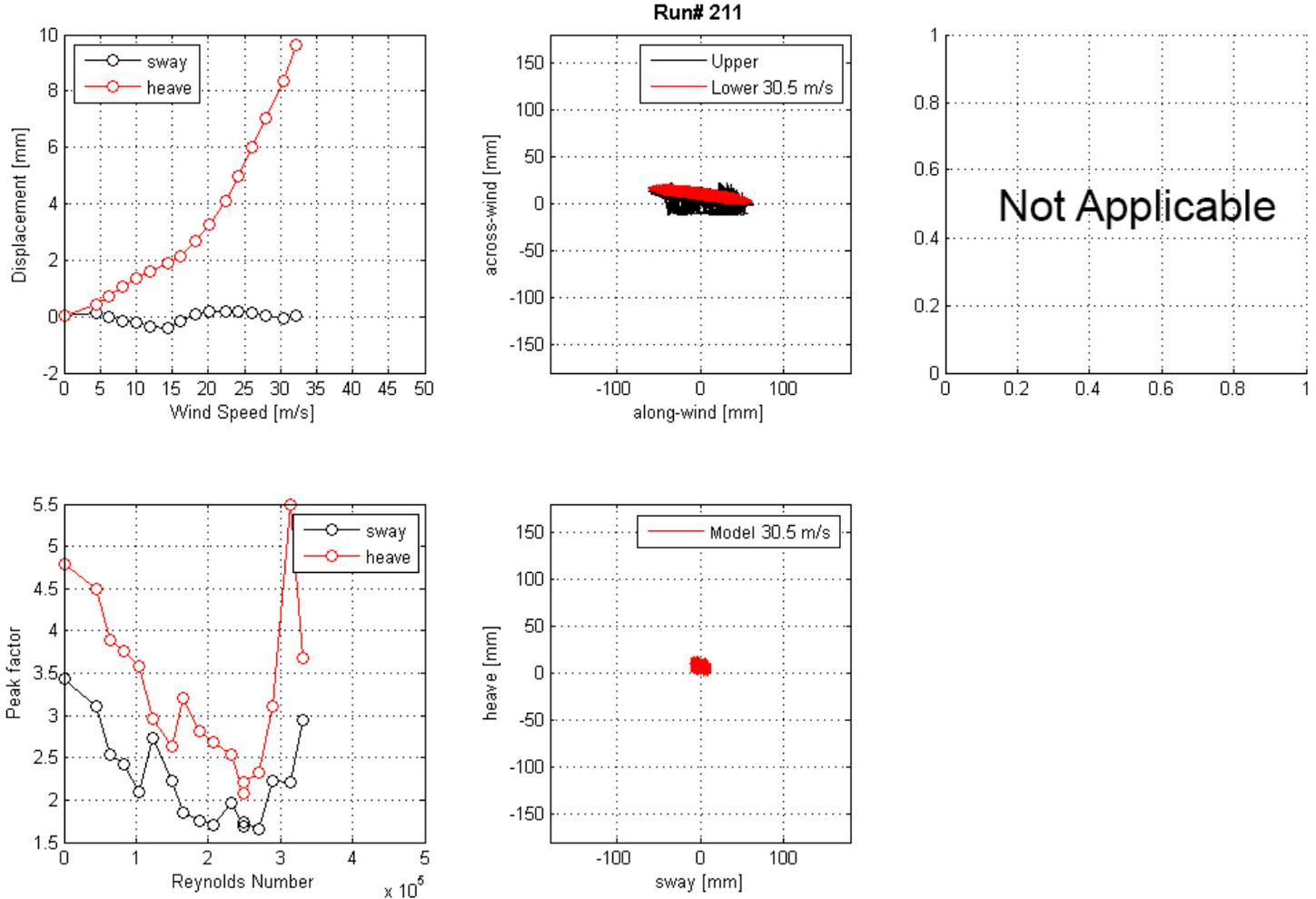
**Figure 151. Graph. Mean displacement and peak factor from the laser, motion path at one wind speed, and intensity of turbulence measured at the entrance of the test section for run 211.**
