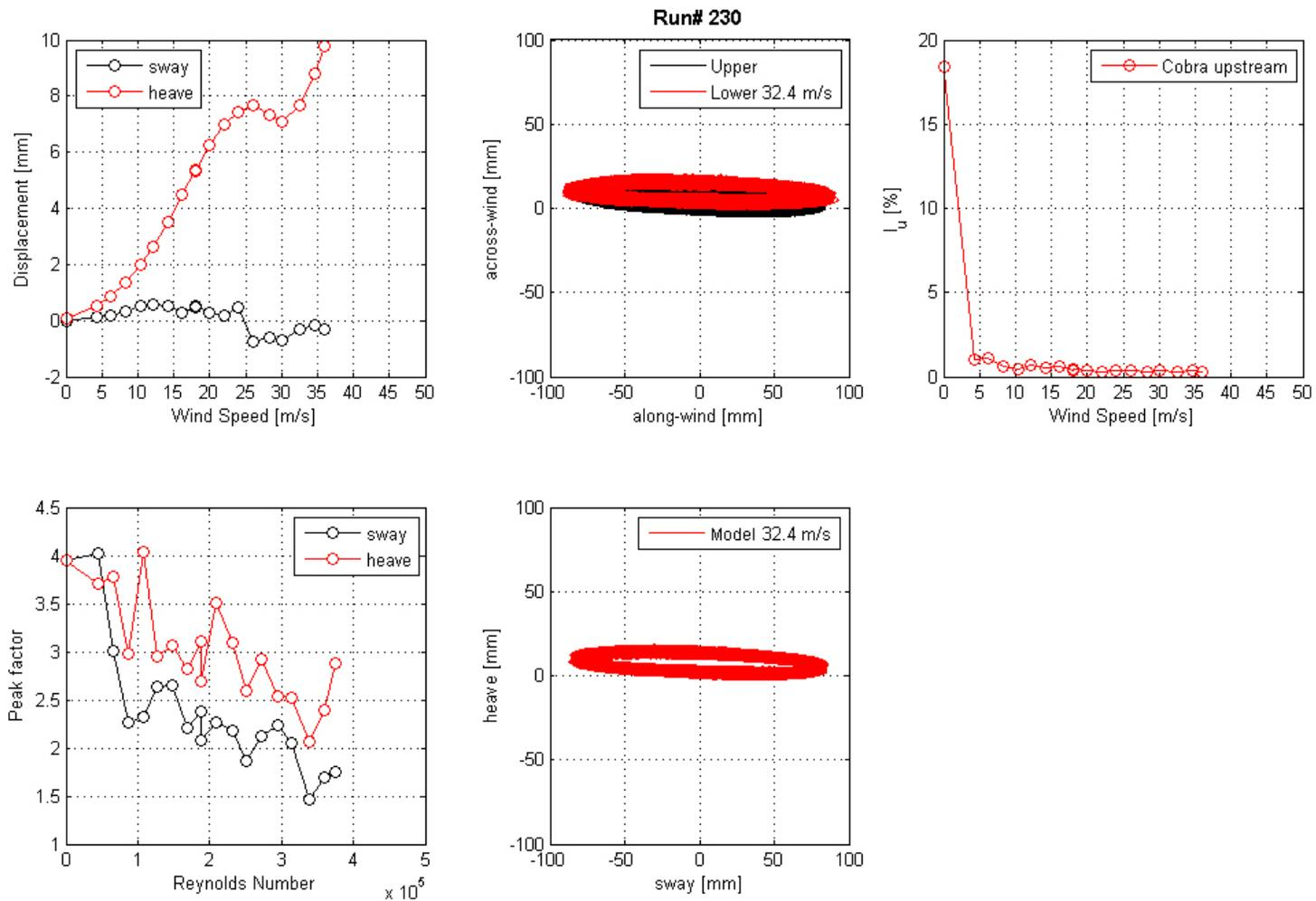
**Figure 165. Graph. Mean displacement and peak factor from the laser, motion path at one wind speed, and intensity of turbulence measured at the entrance of the test section for run 230.**
