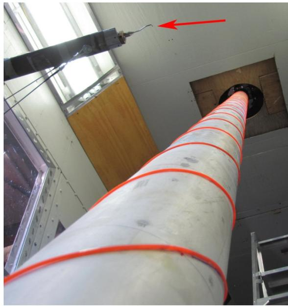
**Figure 49. Photo. TFI Cobra Probe placed in the wake of the cable model directly behind ring 3 of pressure taps.**
