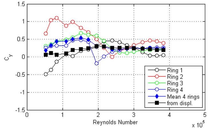
Figure 84. Graph. Response of the cable as a function of wind speed or Reynolds number as measured by the lasers, accelerometers, and surface pressures for run 67.
