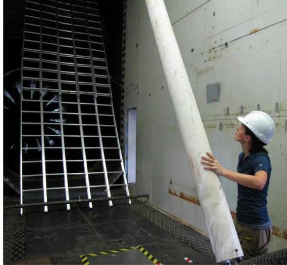
**Figure 17. Photo. Grid of ladders used to generate the turbulent flow field for position 2.**
