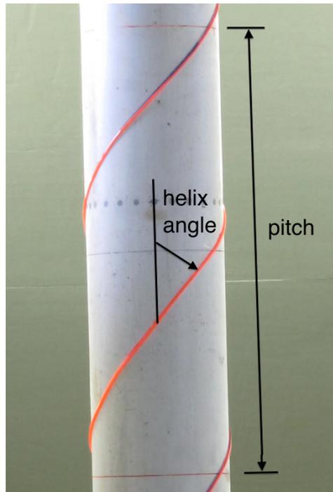
**Figure 3. Photo. Pitch and helix angle.**
