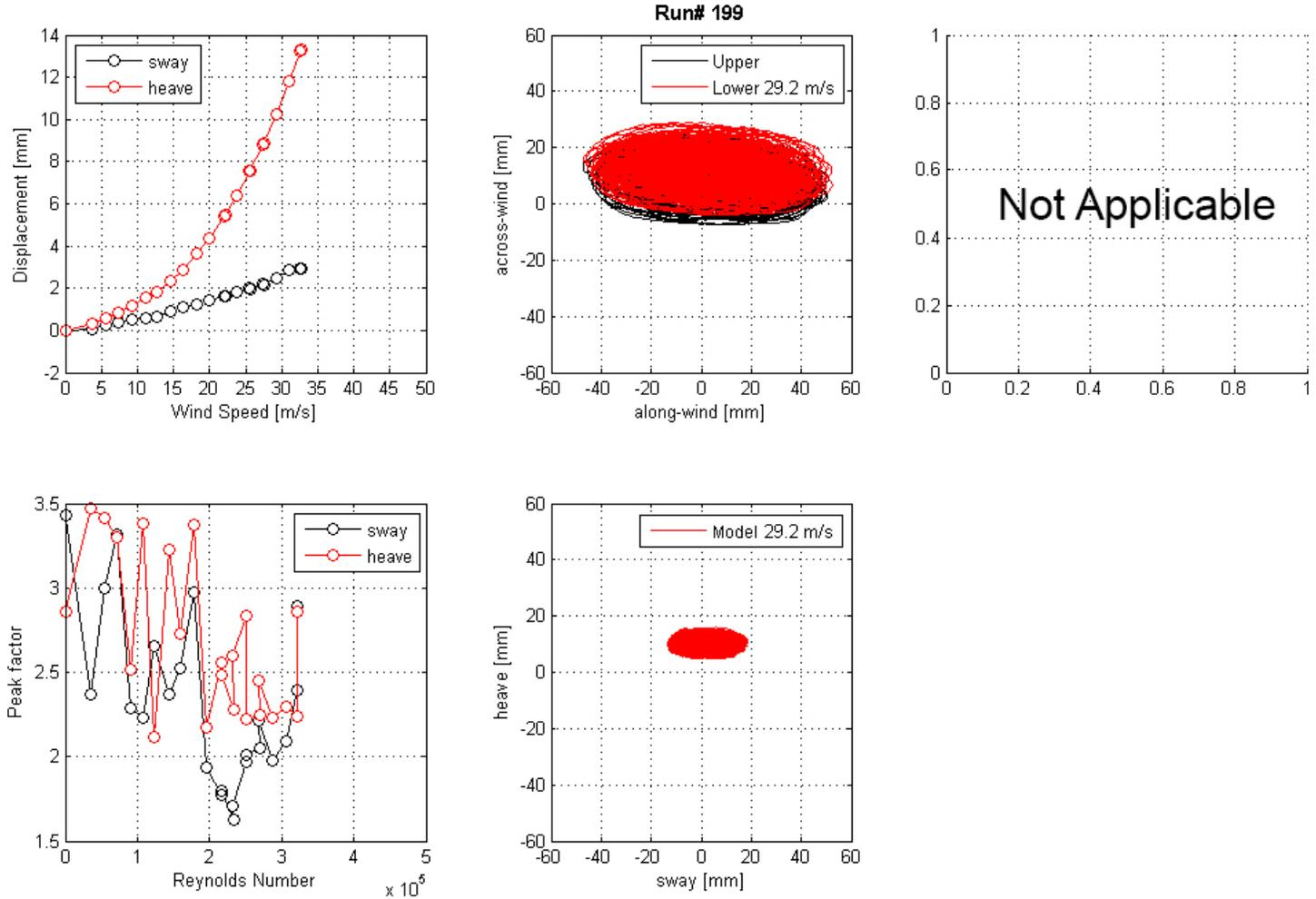
**Figure 143. Graph. Mean displacement and peak factor from the laser, motion path at one wind speed, and intensity of turbulence measured at the entrance of the test section for run 199.**
