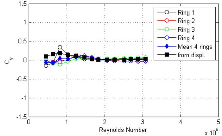
Figure 158. Graph. Response of the cable as a function of wind speed or Reynolds number as measured by the lasers, accelerometers, and surface pressures for run 222.
