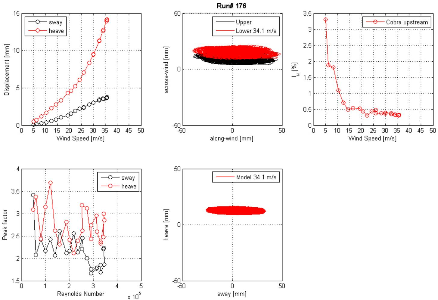
**Figure 137. Graph. Mean displacement and peak factor from the laser, motion path at one wind speed, and intensity of turbulence measured at the entrance of the test section for run 176.**
