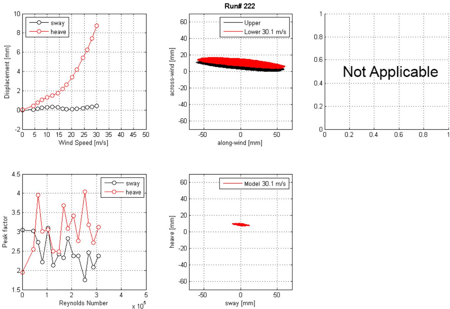
**Figure 159. Graph. Mean displacement and peak factor from the laser, motion path at one wind speed, and intensity of turbulence measured at the entrance of the test section for run 222.**
