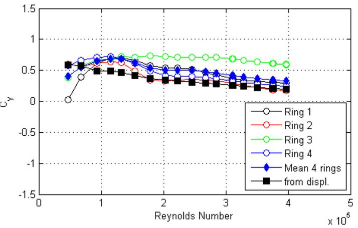
**Figure 128. Graph. Response of the cable as a function of wind speed or Reynolds number as measured by the lasers, accelerometers, and surface pressures for run 155.**
