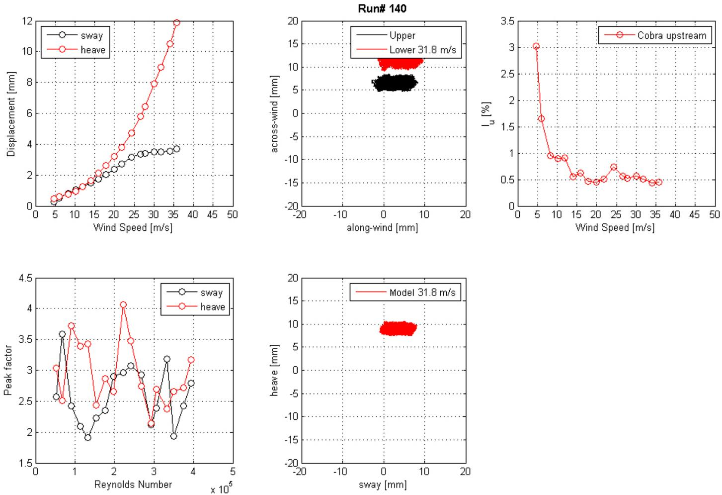
**Figure 119. Graph. Mean displacement and peak factor from the laser, motion path at one wind speed, and intensity of turbulence measured at the entrance of the test section for run 140.**
