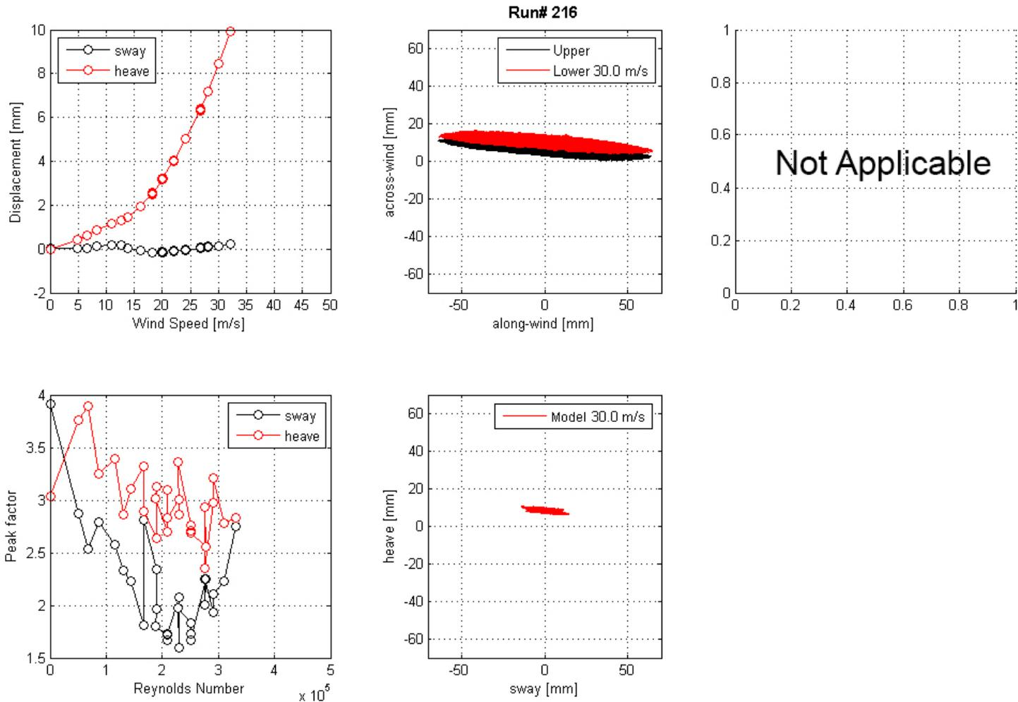
**Figure 155. Graph. Mean displacement and peak factor from the laser, motion path at one wind speed, and intensity of turbulence measured at the entrance of the test section for run 216.**
