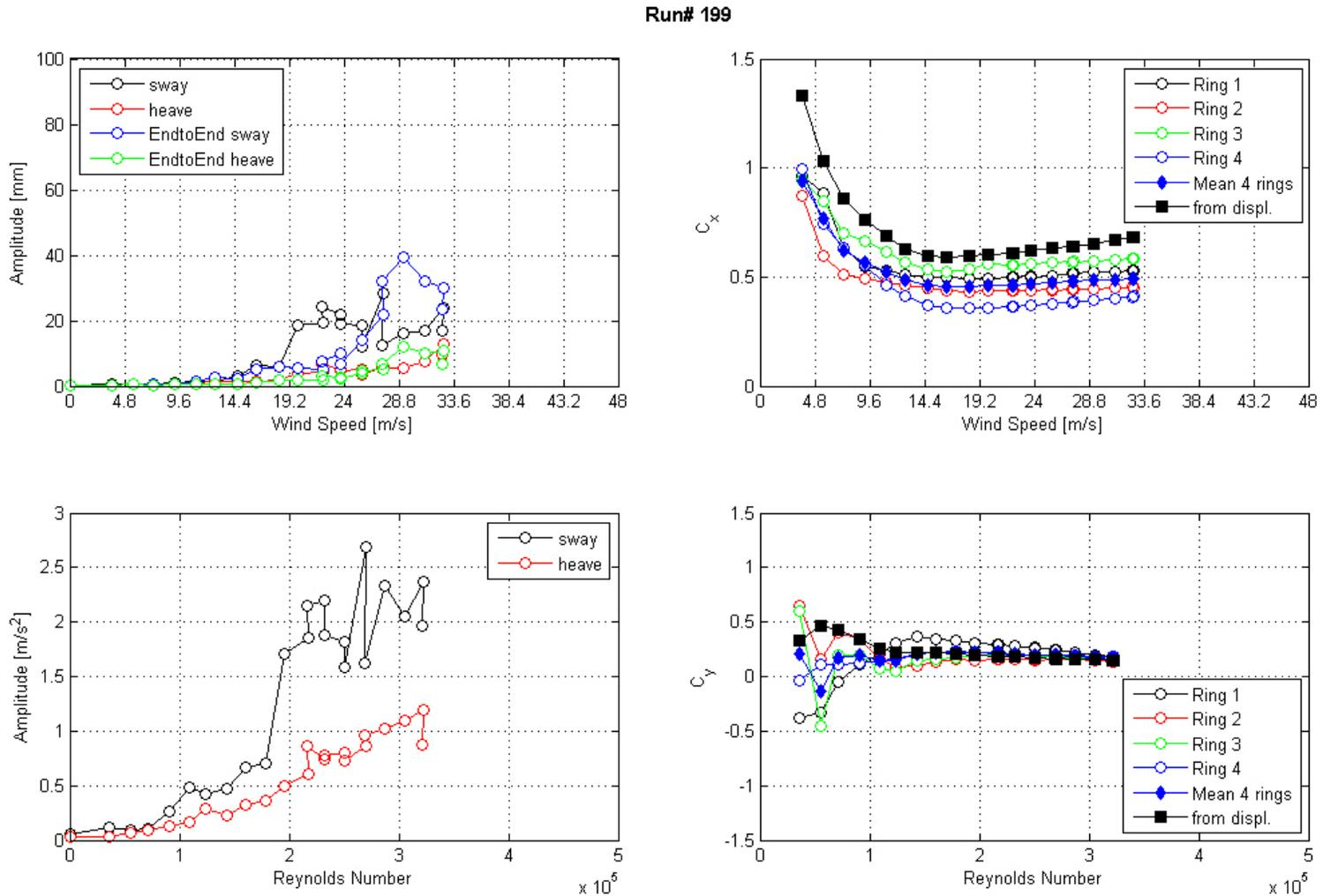
**Figure 142. Graph. Response of the cable as a function of wind speed or Reynolds number as measured by the lasers, accelerometers, and surface pressures for run 199.**
