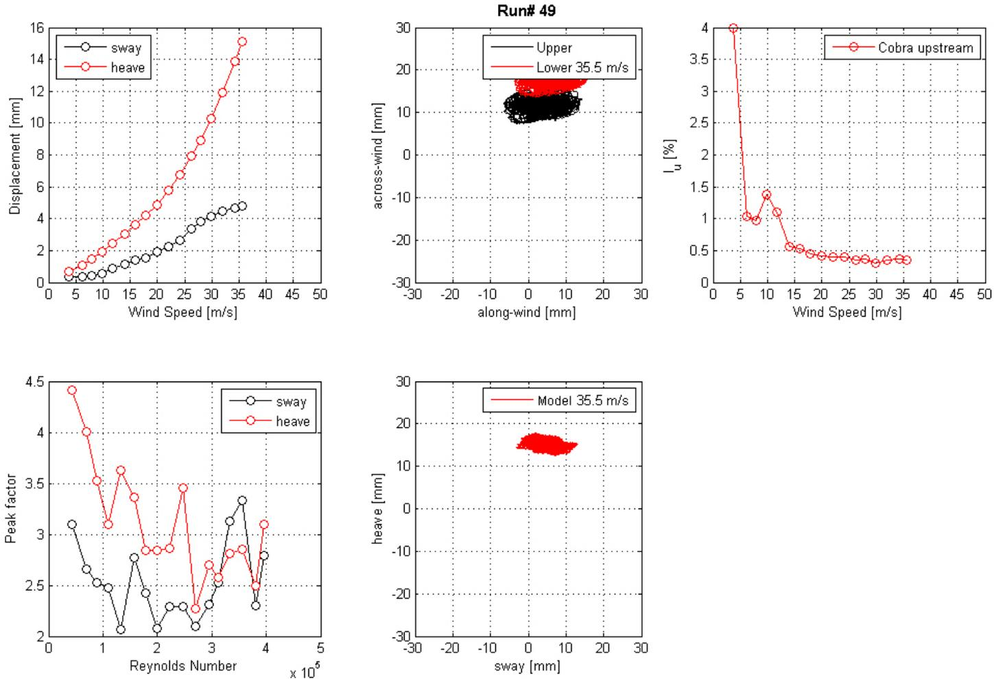
**Figure 73. Graph. Mean displacement and peak factor from the laser, motion path at one wind speed, and intensity of turbulence measured at the entrance of the test section for run 49.**
