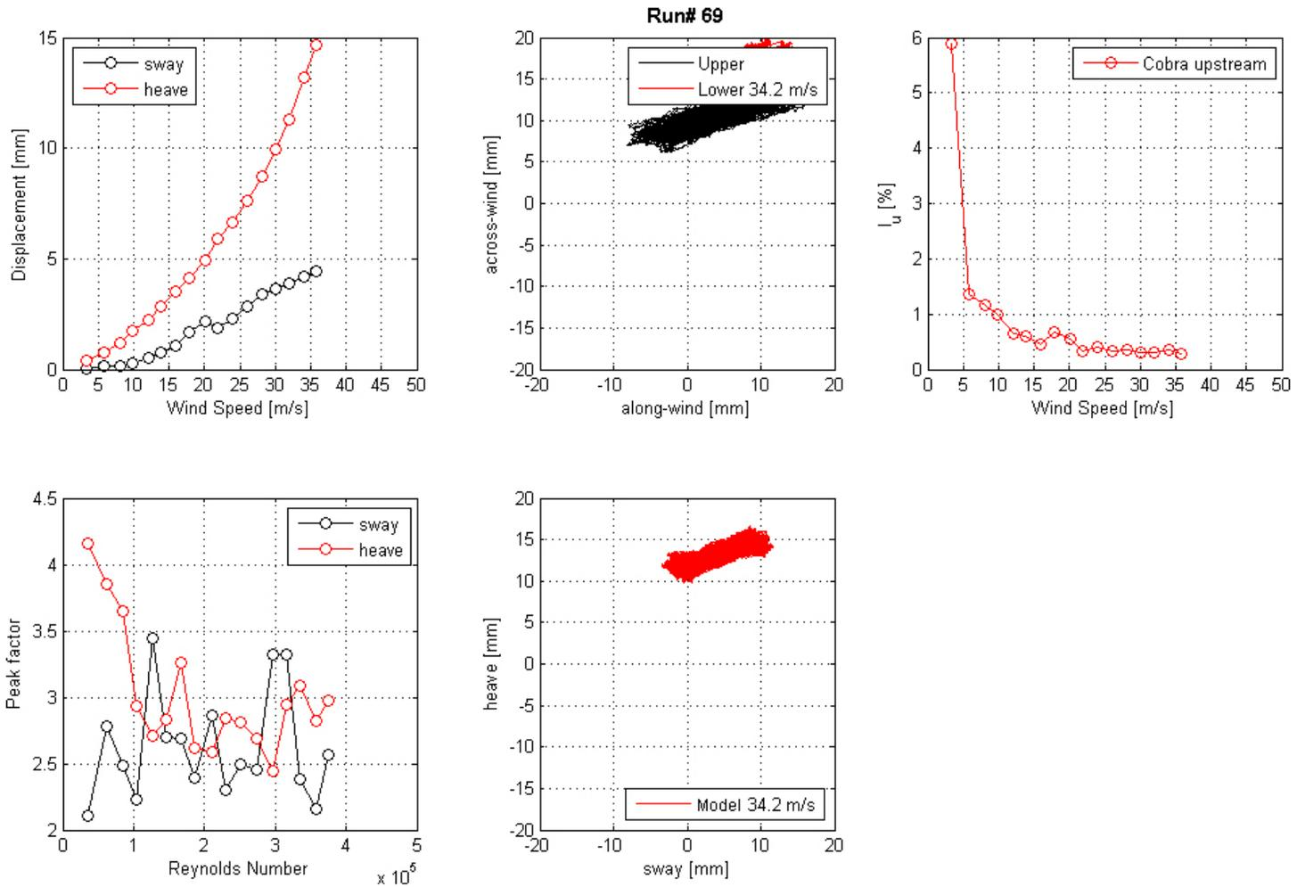
**Figure 87. Graph. Mean displacement and peak factor from the laser, motion path at one wind speed, and intensity of turbulence measured at the entrance of the test section for run 69.**
