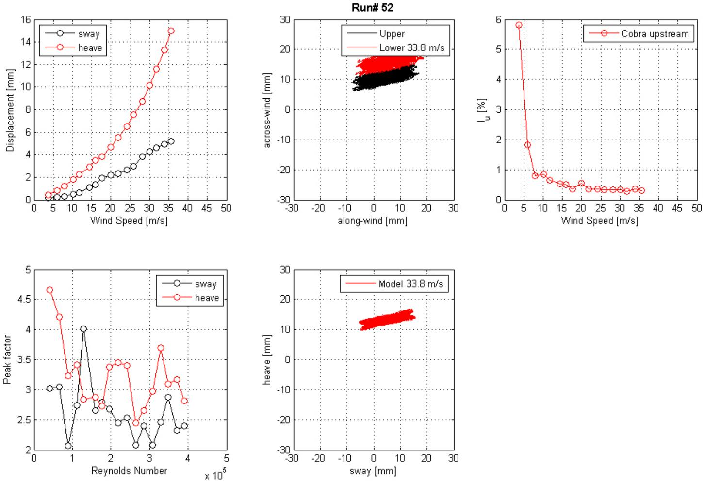
**Figure 75. Graph. Mean displacement and peak factor from the laser, motion path at one wind speed, and intensity of turbulence measured at the entrance of the test section for run 52.**
