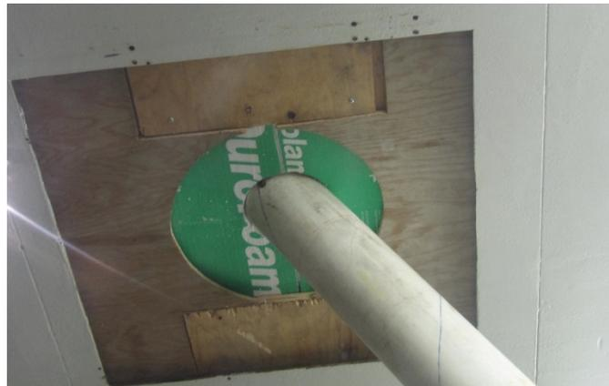
**Figure 13. Photo. Underside of the sealed interface between the cable model and the roof of the wind tunnel.**
