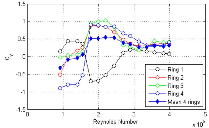
Figure 66. Graph. Intensity of turbulence measured at the entrance of the test section and  $C_x$  and  $C_y$  calculated from surface pressure measurements as a function of Reynolds number and wind speed for run 39.
