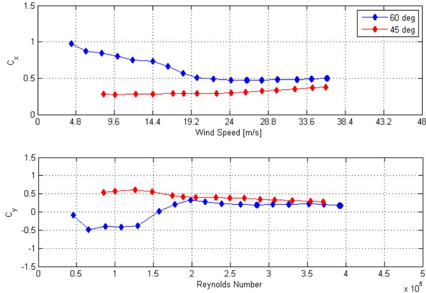
**Figure 32. Graph. Mean force coefficients calculated from the integration of surface pressure measurements for the cable inclined at 60 and 45 degrees and rotated at -90 degrees along its main axis in smooth flow and with a helical fillet.**
