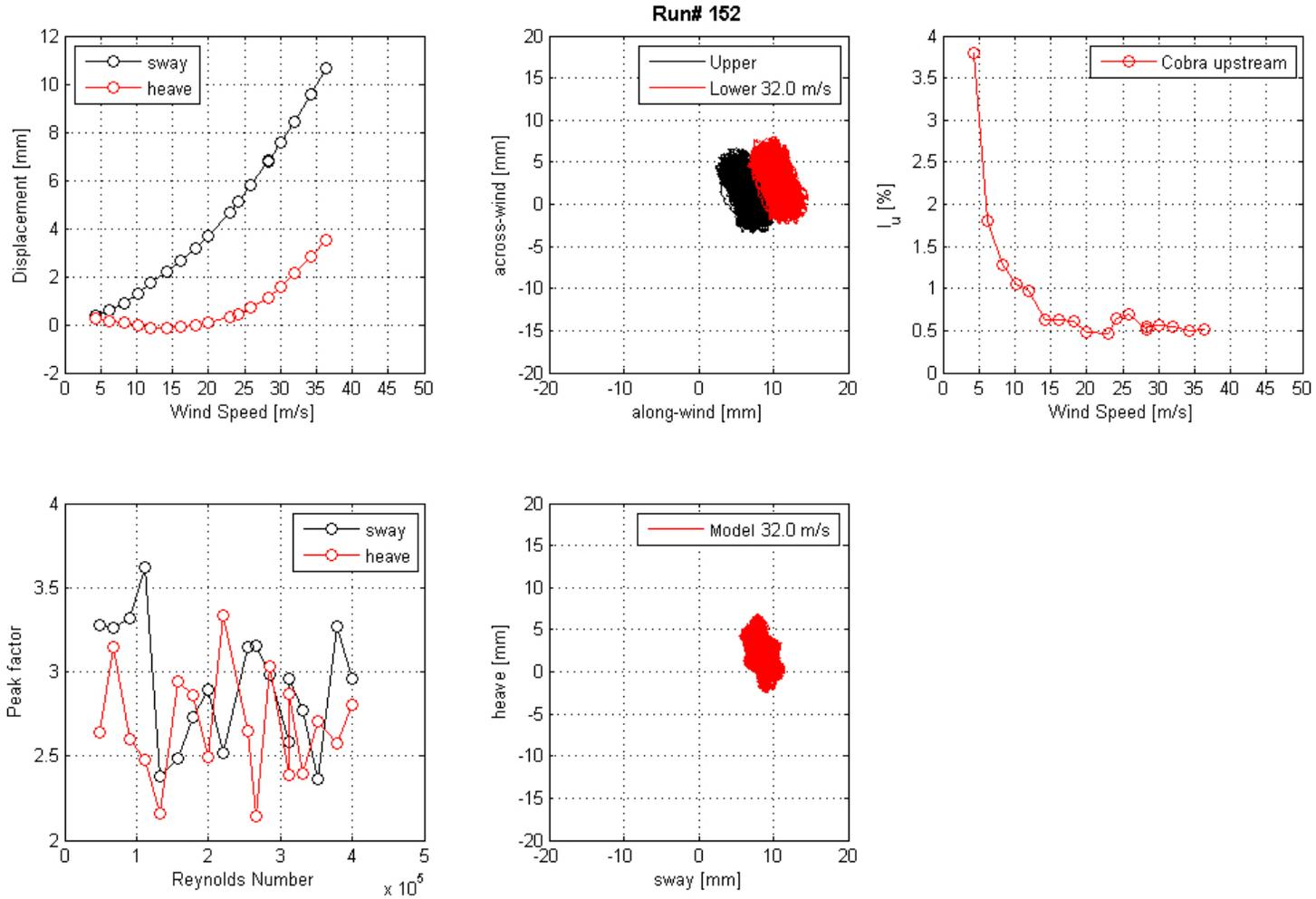
**Figure 127. Graph. Mean displacement and peak factor from the laser, motion path at one wind speed, and intensity of turbulence measured at the entrance of the test section for run 152.**
