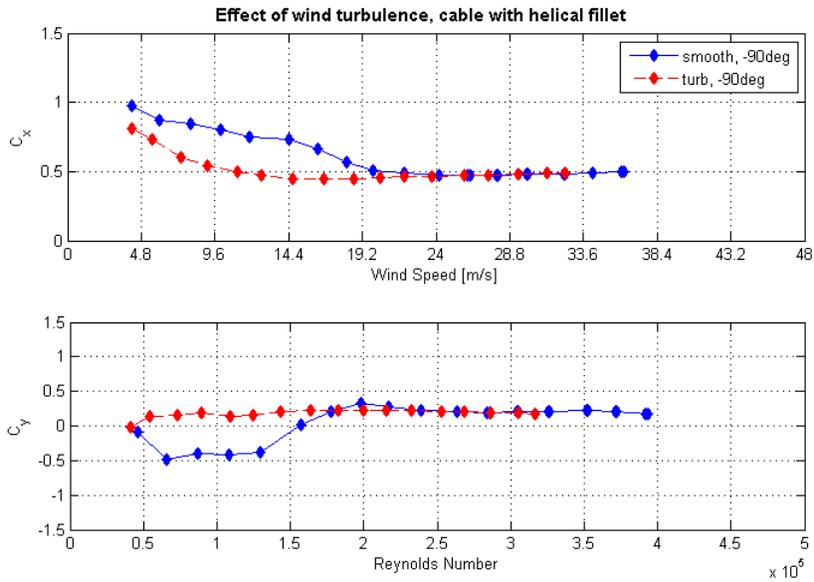
**Figure 41. Graph. Mean force coefficients at cable rotation of -90 degrees and inclined at 60 degrees with a helical fillet in smooth and turbulent flow.**
