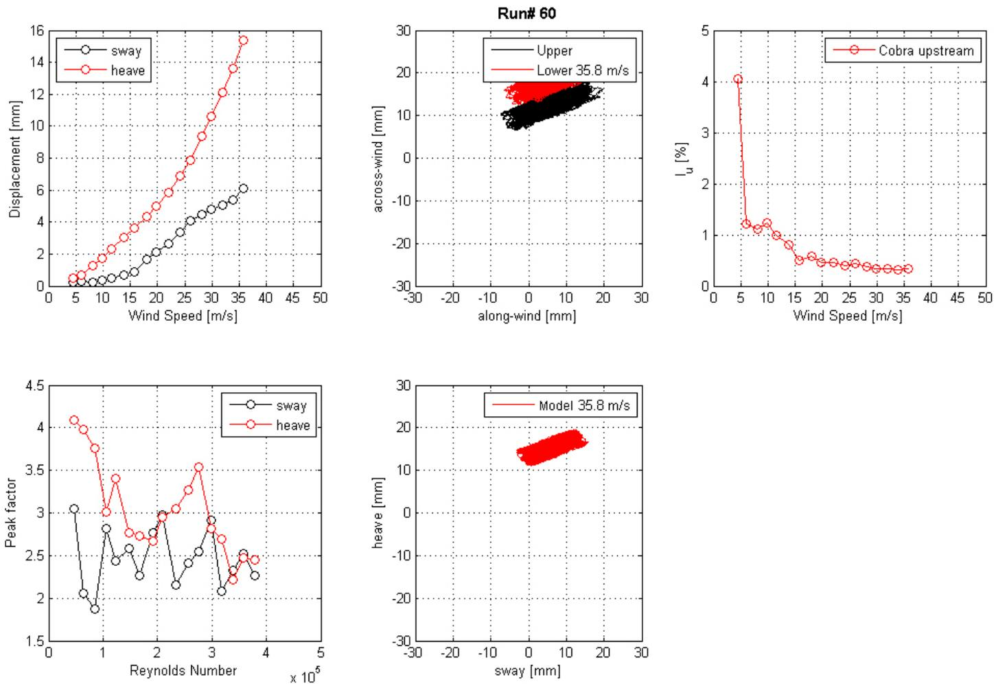
**Figure 79. Graph. Mean displacement and peak factor from the laser, motion path at one wind speed, and intensity of turbulence measured at the entrance of the test section for run 60.**
