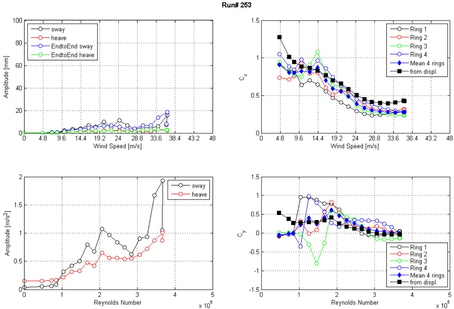
**Figure 176. Graph. Response of the cable as a function of wind speed or Reynolds number as measured by the lasers, accelerometers, and surface pressures for run 253.**
