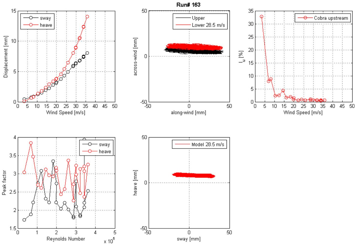
**Figure 133. Graph. Mean displacement and peak factor from the laser, motion path at one wind speed, and intensity of turbulence measured at the entrance of the test section for run 163.**
