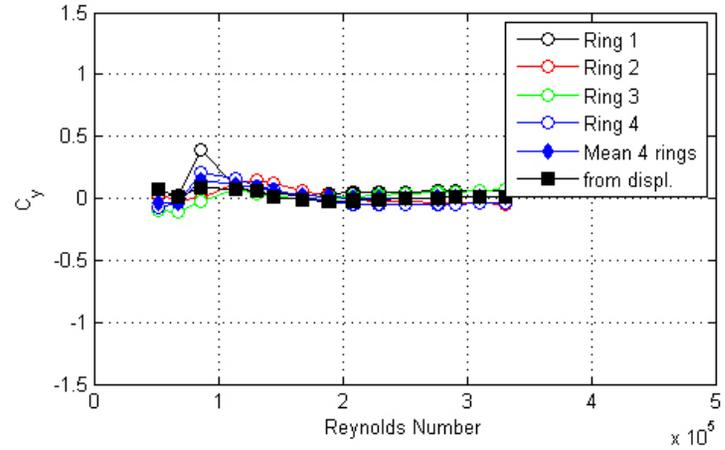
Figure 154. Graph. Response of the cable as a function of wind speed or Reynolds number as measured by the lasers, accelerometers, and surface pressures for run 216.
