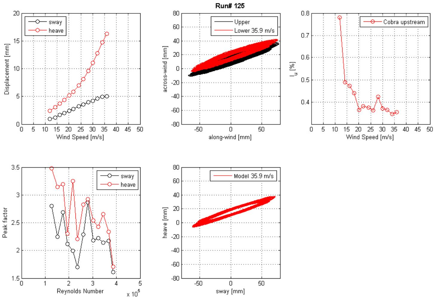
**Figure 111. Graph. Mean displacement and peak factor from the laser, motion path at one wind speed, and intensity of turbulence measured at the entrance of the test section for run 125.**
