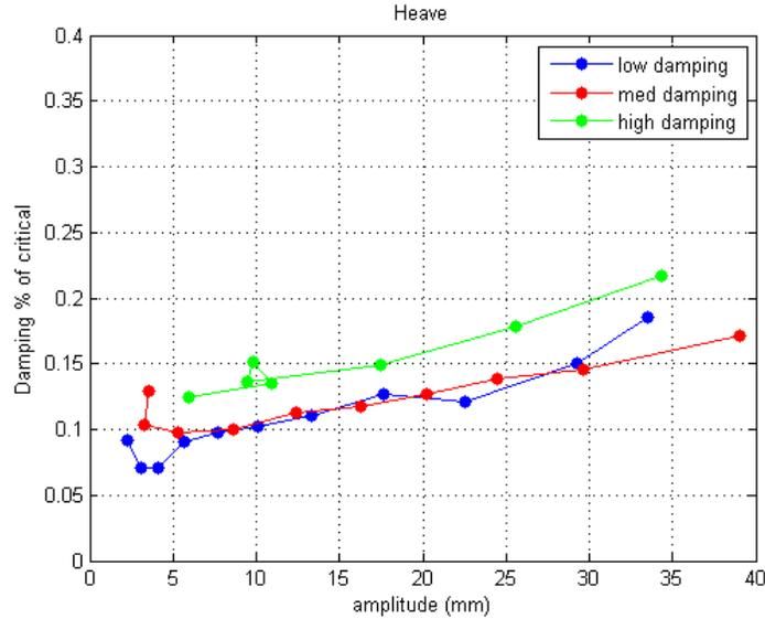
**Figure 37. Graph. Structural damping level as a function of amplitude of motion of the cable for the heave mode.**
