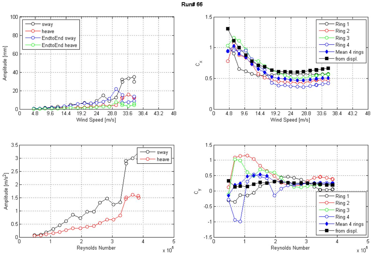
**Figure 82. Graph. Response of the cable as a function of wind speed or Reynolds number as measured by the lasers, accelerometers, and surface pressures for run 66.**
