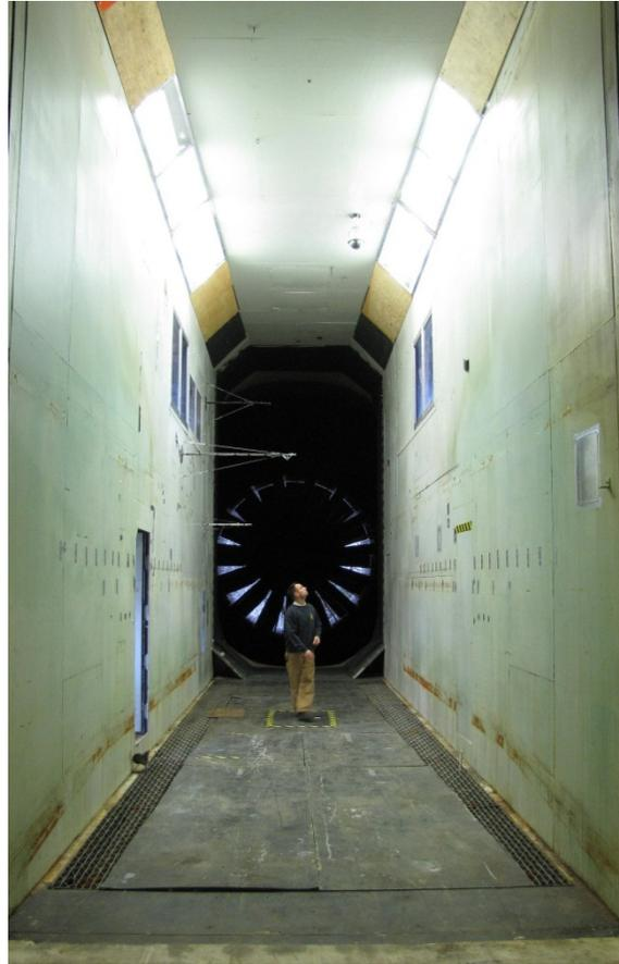
**Figure 14. Photo. Downstream view of the test section during dynamic pressure calibration prior to the installation of the cable model.**
