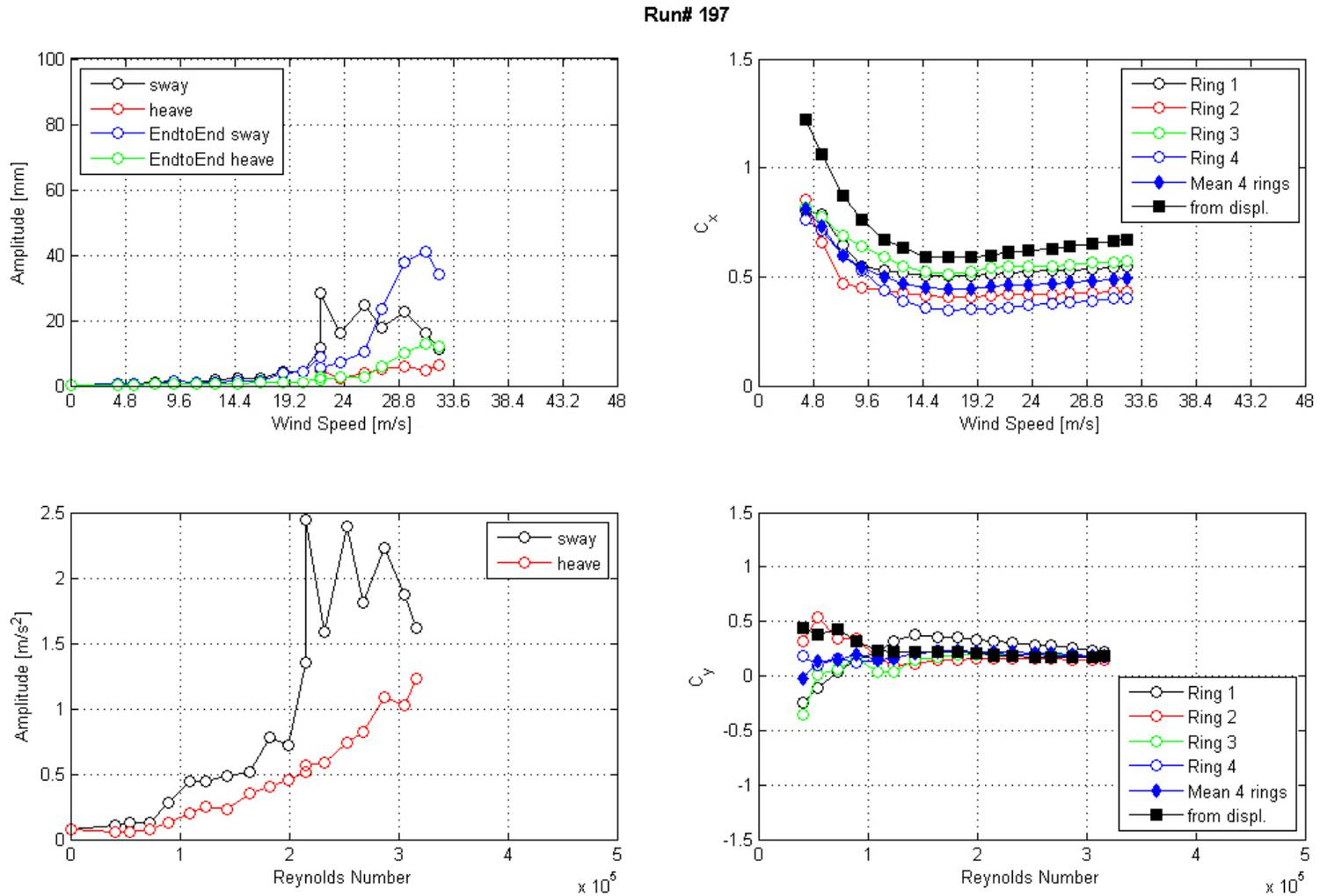
**Figure 140. Graph. Response of the cable as a function of wind speed or Reynolds number as measured by the lasers, accelerometers, and surface pressures for run 197.**
