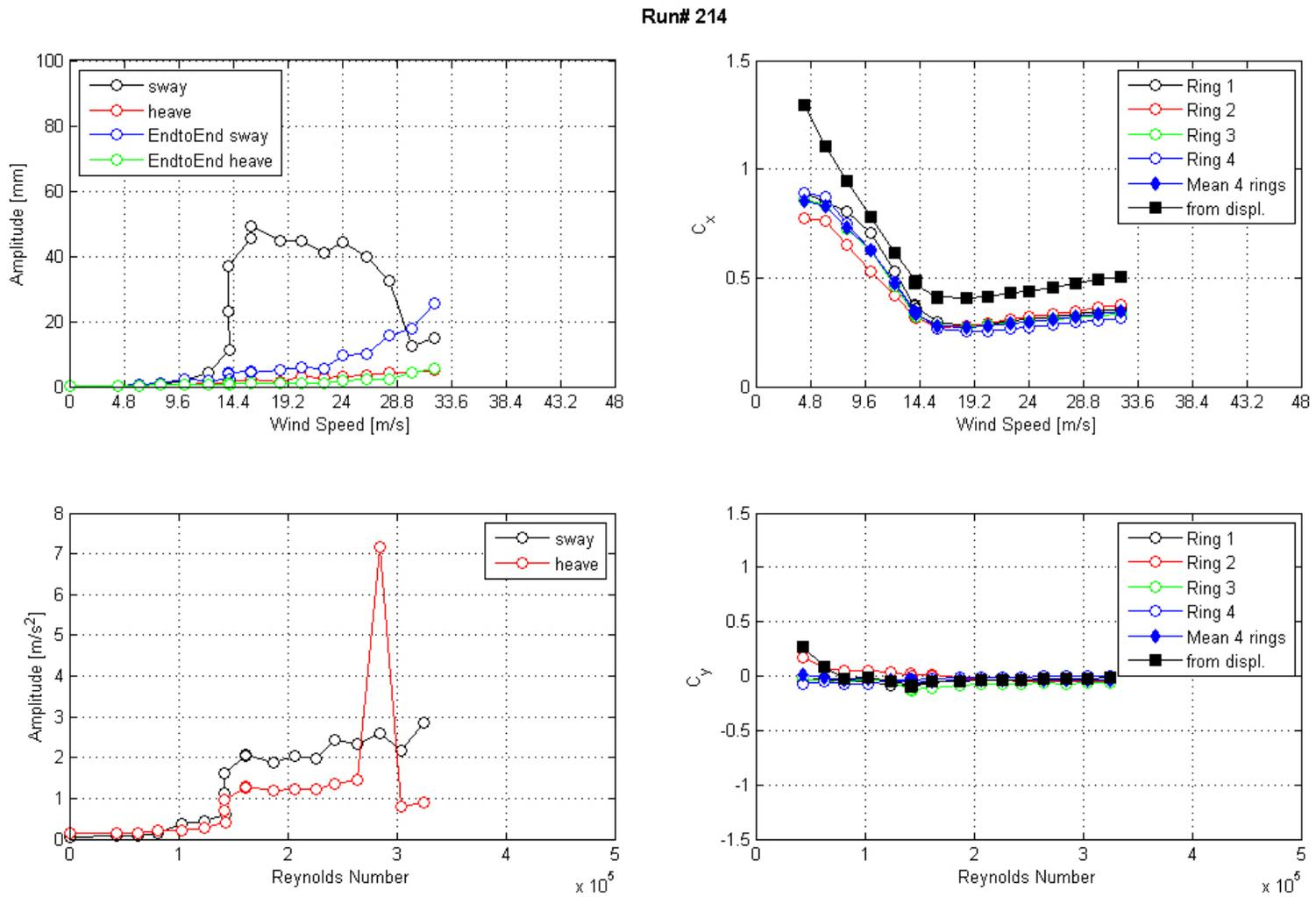
**Figure 152. Graph. Response of the cable as a function of wind speed or Reynolds number as measured by the lasers, accelerometers, and surface pressures for run 214.**
