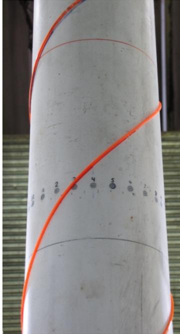
**Figure 5. Photo. Close-up view of double helical right-handed fillet.**
