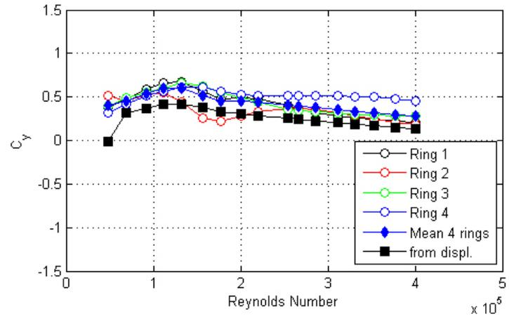
Figure 126. Graph. Response of the cable as a function of wind speed or Reynolds number as measured by the lasers, accelerometers, and surface pressures for run 152.
