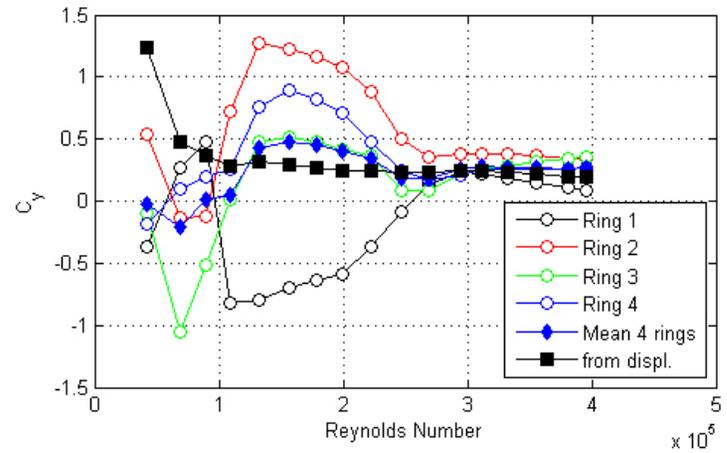
Figure 72. Graph. Response of the cable as a function of wind speed or Reynolds number as measured by the lasers, accelerometers, and surface pressures for run 49.
