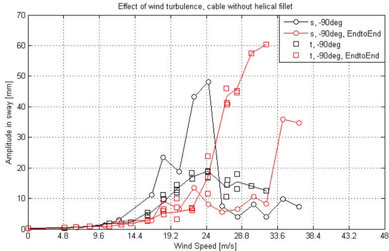
**Figure 42. Graph. Amplitude of motion in sway and end-to-end sway at cable rotation of -90 degrees and inclined at 60 degrees without a helical fillet in smooth and turbulent flow.**
