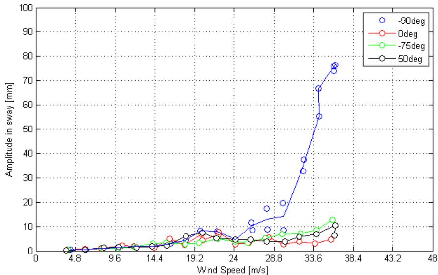
**Figure 29. Graph. Amplitude of motion in sway for four different rotations of the cable along its main axis for the cable inclined at 60 degrees with helical fillet and in smooth flow.**
