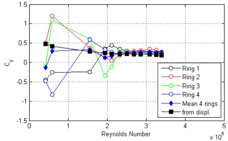
Figure 138. Graph. Response of the cable as a function of wind speed or Reynolds number as measured by the lasers, accelerometers, and surface pressures for run 178.
