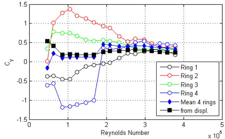
Figure 78. Graph. Response of the cable as a function of wind speed or Reynolds number as measured by the lasers, accelerometers, and surface pressures for run 60.
