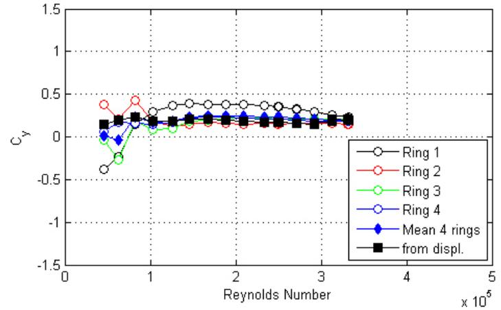
Figure 144. Graph. Response of the cable as a function of wind speed or Reynolds number as measured by the lasers, accelerometers, and surface pressures for run 203.
