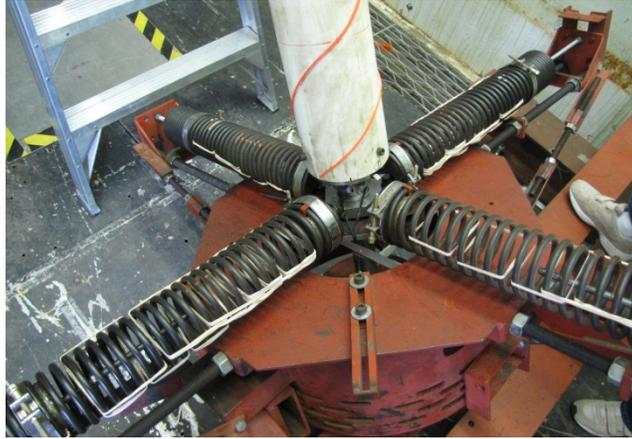
**Figure 33. Photo. Elastic bands used to increase the structural damping of the suspension system.**
