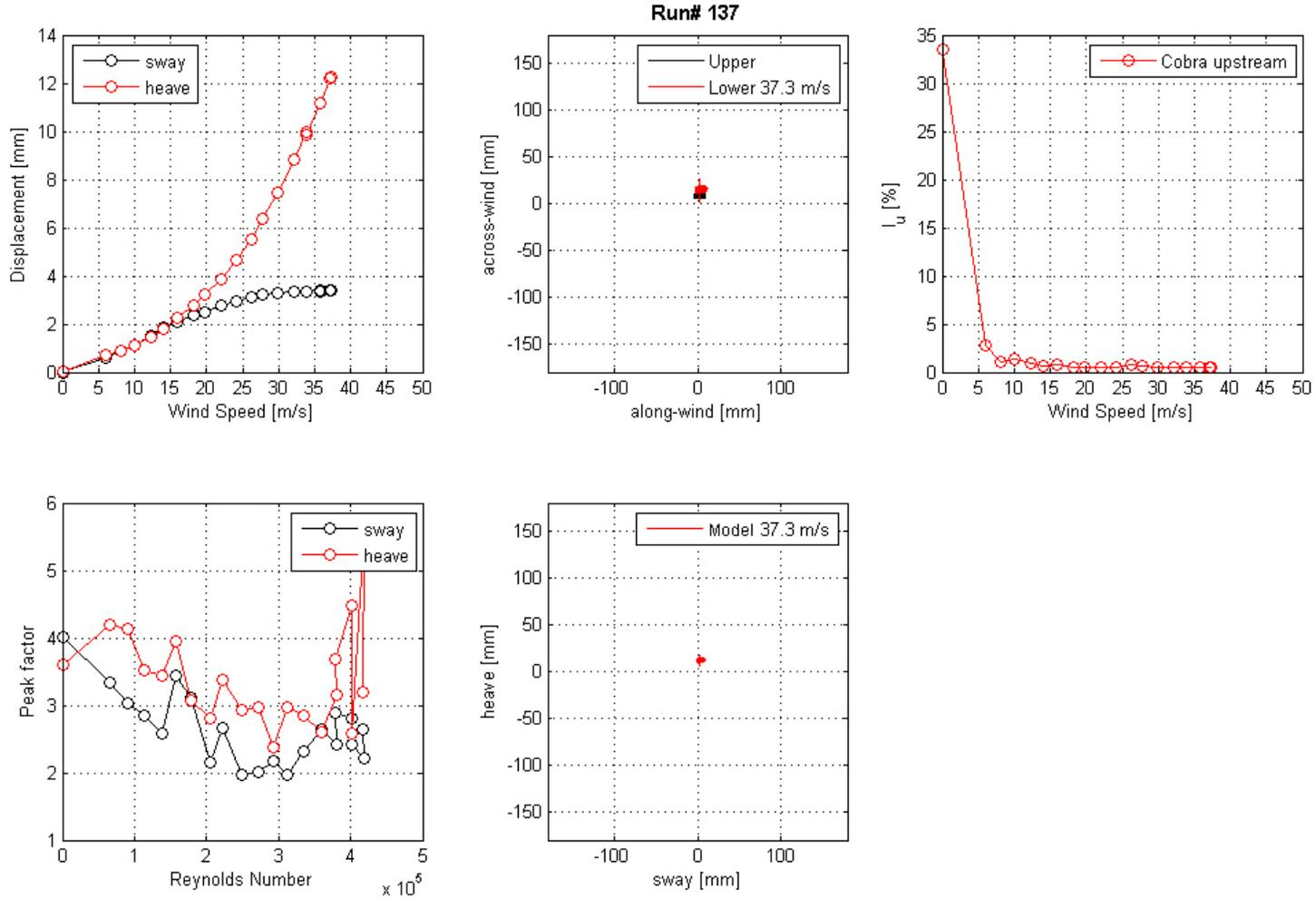
**Figure 117. Graph. Mean displacement and peak factor from the laser, motion path at one wind speed, and intensity of turbulence measured at the entrance of the test section for run 137.**
