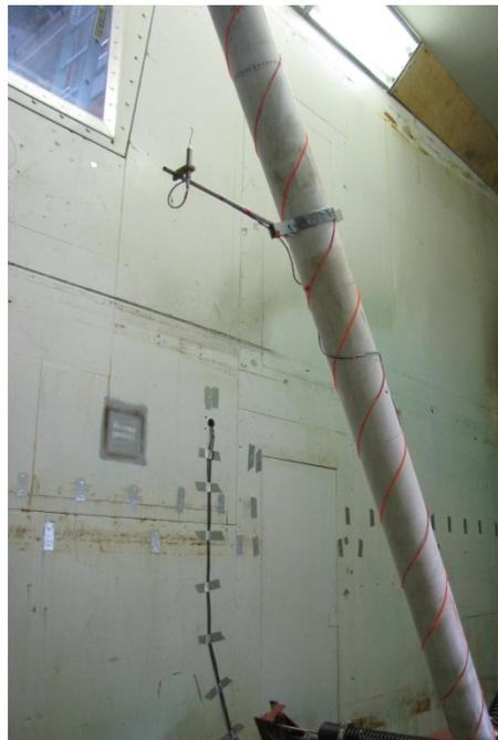
**Figure 18. Photo. TFI Cobra Probe attached to the cable model to measure the turbulence level behind the grid of ladders.**
