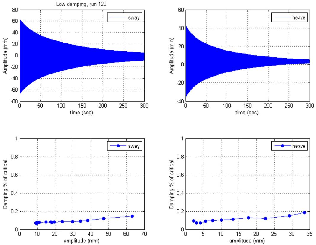
**Figure 184. Graph. Damping traces and level for the sway and heave modes for the low damping level case.**
