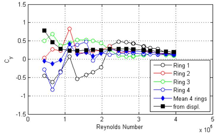
Figure 104. Graph. Response of the cable as a function of wind speed or Reynolds number as measured by the lasers, accelerometers, and surface pressures for run 118.
