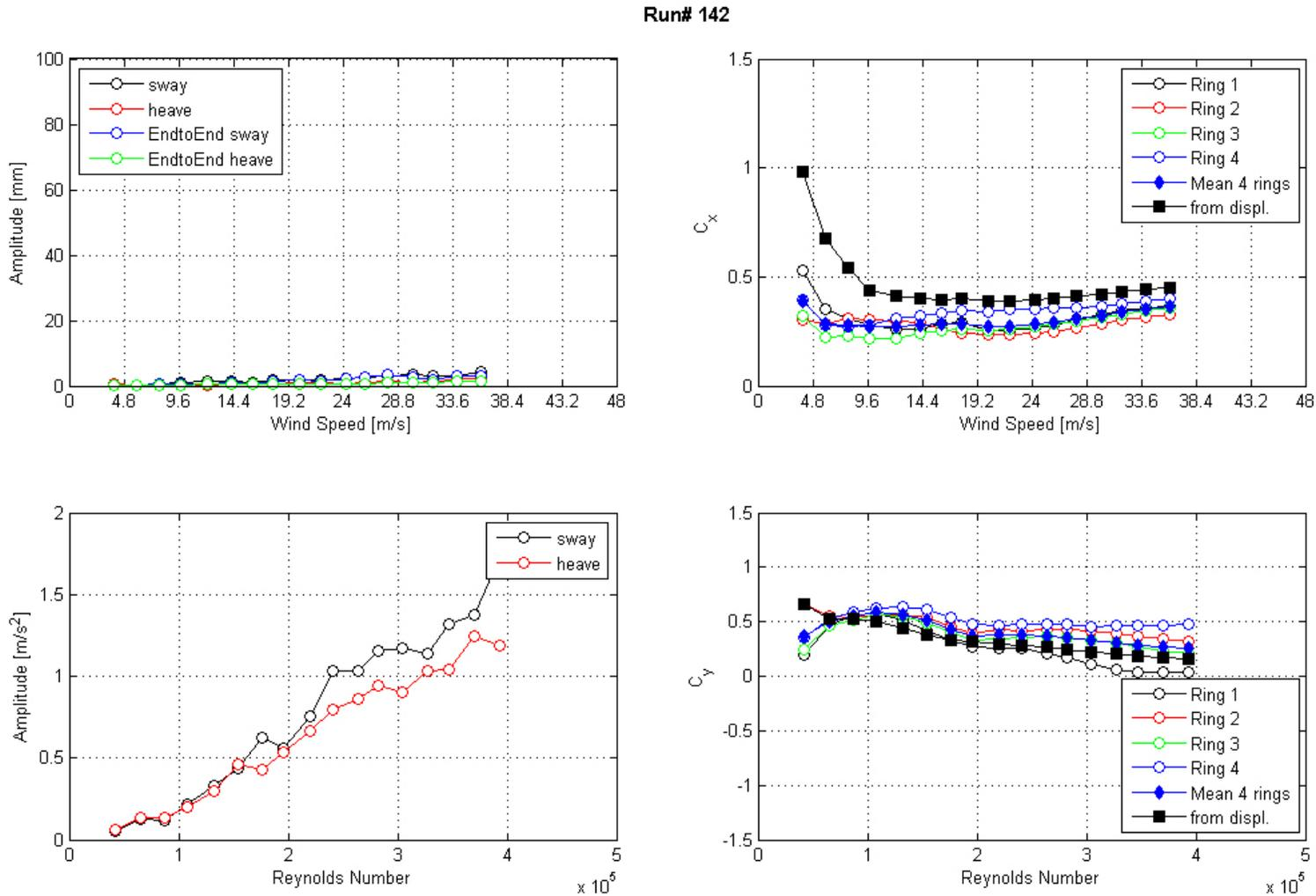
**Figure 120. Graph. Response of the cable as a function of wind speed or Reynolds number as measured by the lasers, accelerometers, and surface pressures for run 142.**
