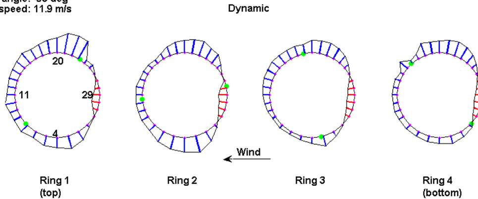
**Figure 47. Illustration. Distribution of surface pressure coefficient for the four rings with the cable in motion (run 122).**
