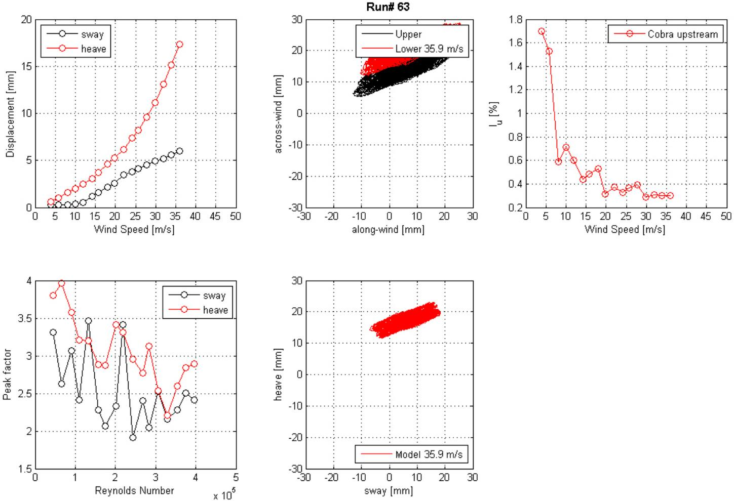
**Figure 81. Graph. Mean displacement and peak factor from the laser, motion path at one wind speed, and intensity of turbulence measured at the entrance of the test section for run 63.**
