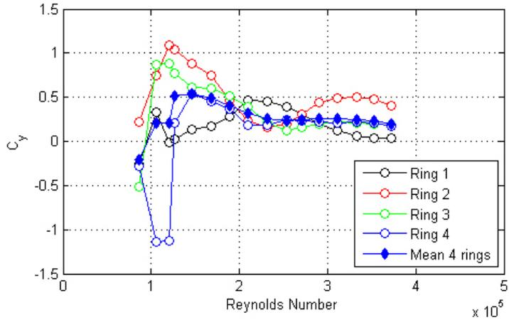
Figure 94. Graph. Intensity of turbulence measured at the entrance of the test section and  $C_x$  and  $C_y$  calculated from surface pressure measurements as a function of Reynolds number and wind speed for run 81.
