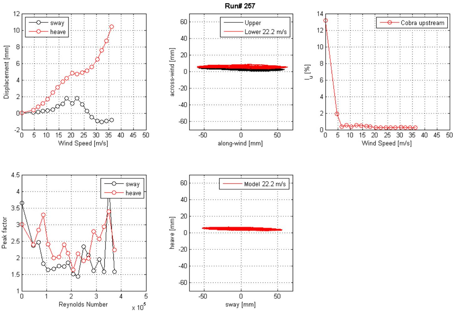
**Figure 181. Graph. Mean displacement and peak factor from the laser, motion path at one wind speed, and intensity of turbulence measured at the entrance of the test section for run 257.**
