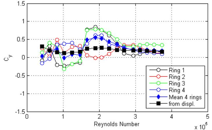
Figure 88. Graph. Response of the cable as a function of wind speed or Reynolds number as measured by the lasers, accelerometers, and surface pressures for run 71.
