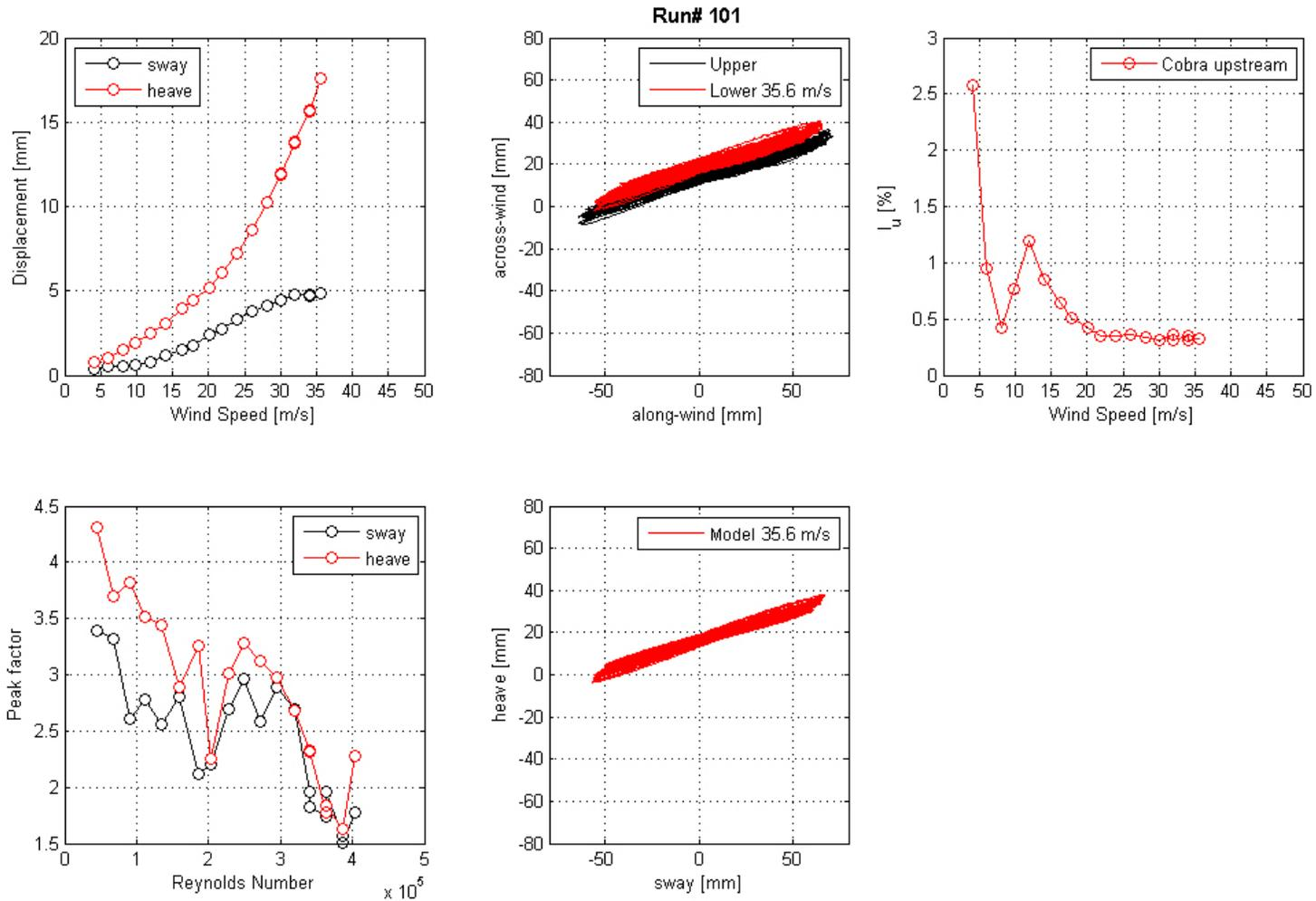
**Figure 101. Graph. Mean displacement and peak factor from the laser, motion path at one wind speed, and intensity of turbulence measured at the entrance of the test section for run 101.**
