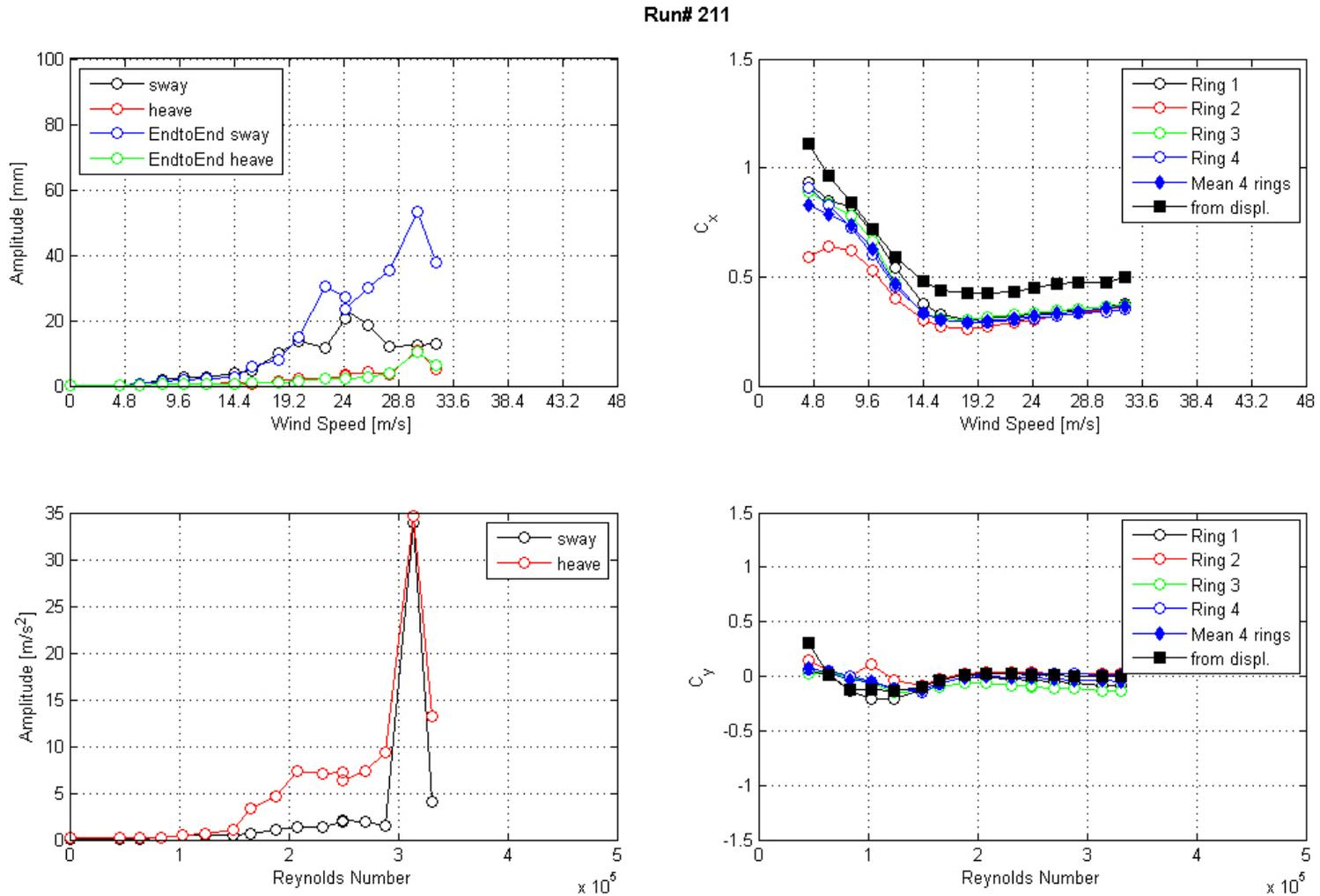
**Figure 150. Graph. Response of the cable as a function of wind speed or Reynolds number as measured by the lasers, accelerometers, and surface pressures for run 211.**
