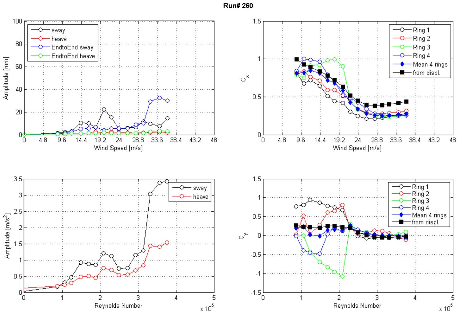
**Figure 182. Graph. Response of the cable as a function of wind speed or Reynolds number as measured by the lasers, accelerometers, and surface pressures for run 260.**
