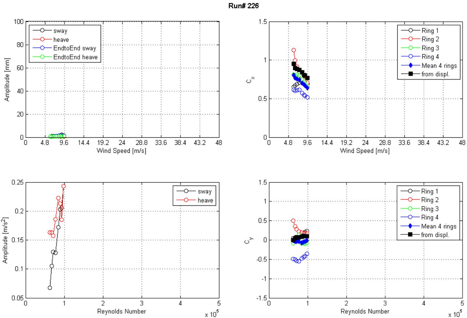
**Figure 162. Graph. Response of the cable as a function of wind speed or Reynolds number as measured by the lasers, accelerometers, and surface pressures for run 226.**
