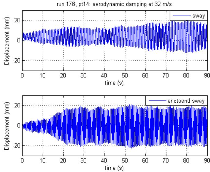
**Figure 26. Graph. Growth of the cable model vibration as a function of time inclined at 60 degrees and rotated at -90 degrees.**
