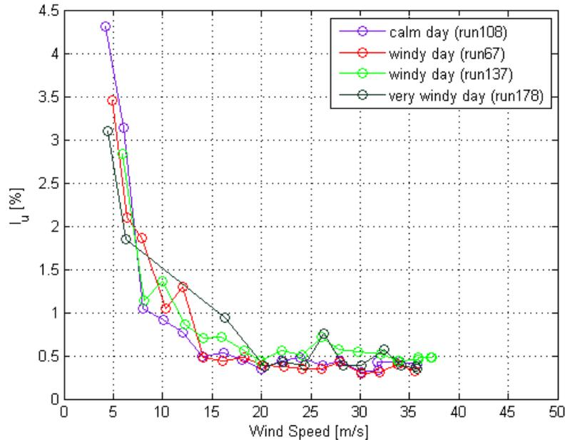
**Figure 15. Graph. Variations of  $I_u$  with wind speed measured at the entrance of the test section for different external conditions for the smooth flow case.**
