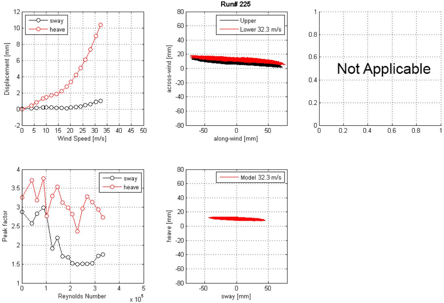
**Figure 161. Graph. Mean displacement and peak factor from the laser, motion path at one wind speed, and intensity of turbulence measured at the entrance of the test section for run 225.**
