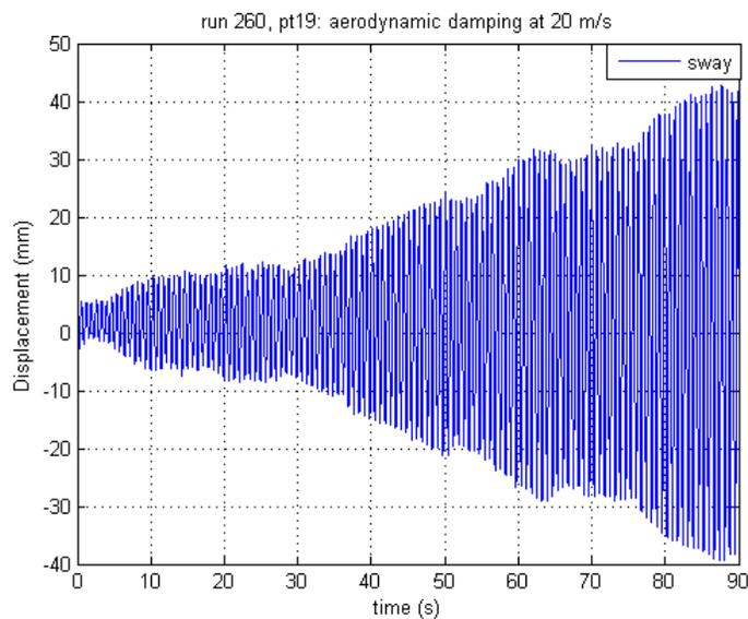
**Figure 25. Graph. Growth of the cable model vibration as a function of time inclined at 60 degrees and rotated at -88 degrees.**
