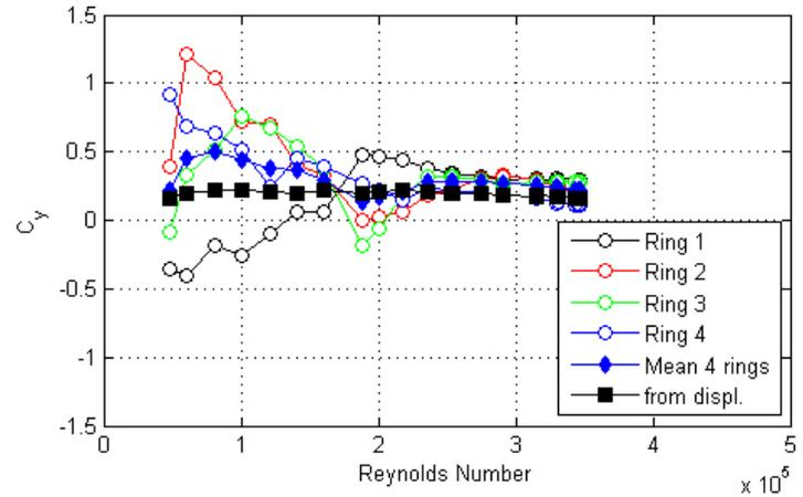
Figure 136. Graph. Response of the cable as a function of wind speed or Reynolds number as measured by the lasers, accelerometers, and surface pressures for run 176.
