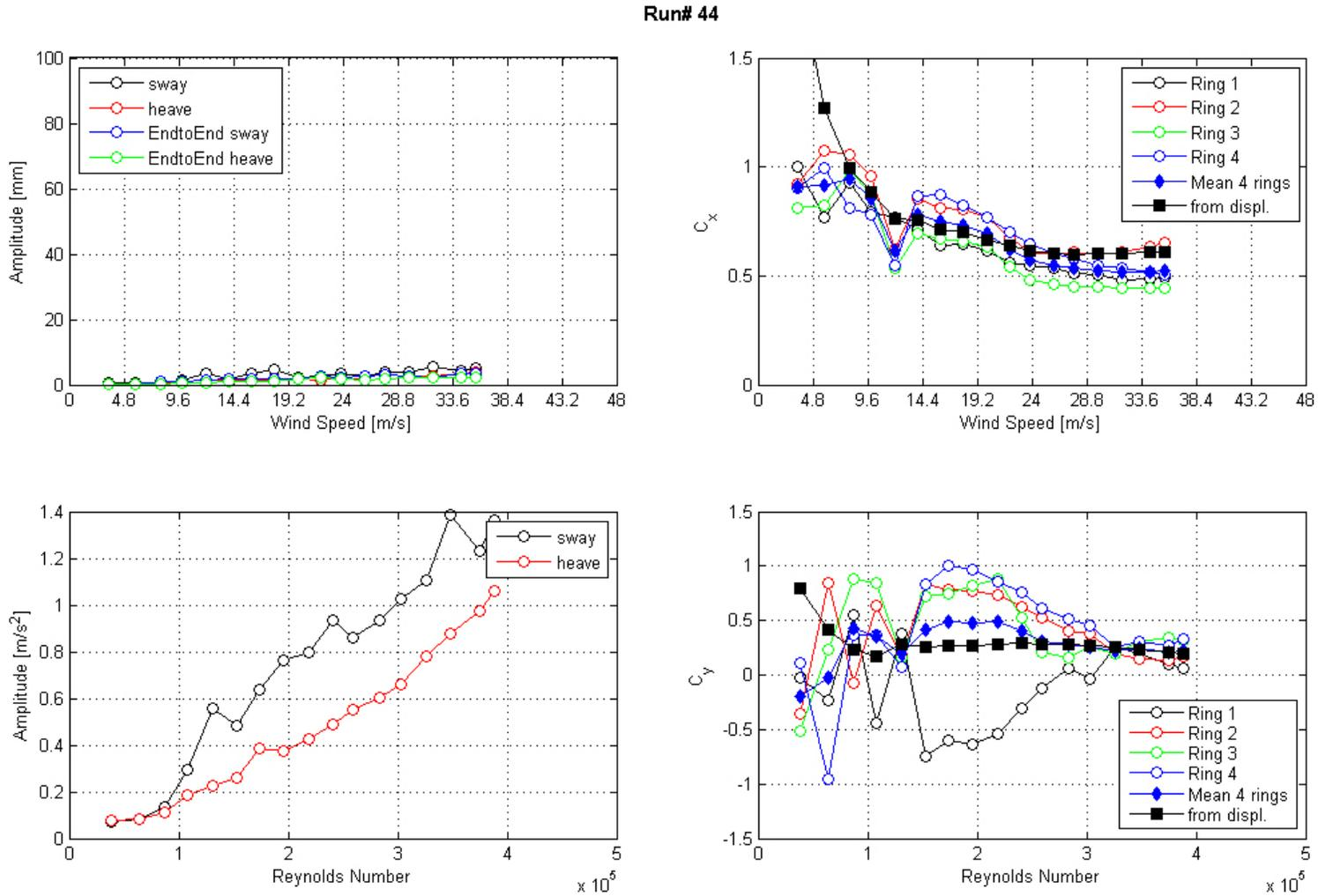
Figure 68. Graph. Response of the cable as a function of wind speed or Reynolds number as measured by the lasers, accelerometers, and surface pressures for run 44.
