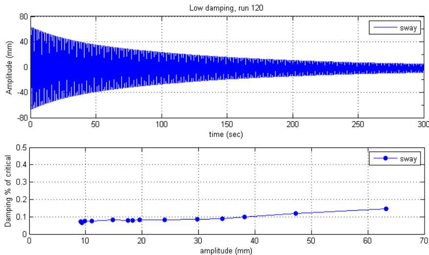
**Figure 27. Graph. Example of decay trace for the sway mode of vibration and corresponding variation of damping with amplitude of vibrations.**
