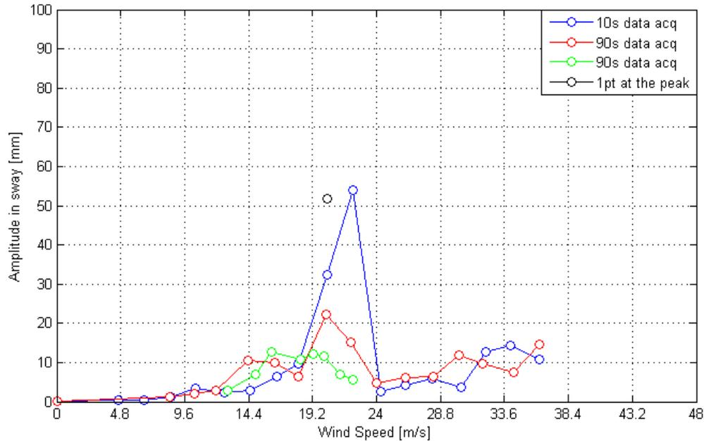
**Figure 58. Graph. Amplitude of motion in sway for four consecutive runs for the cable inclined at 60 degrees and rotated at -88 degrees without the helical fillet and in smooth flow.**
