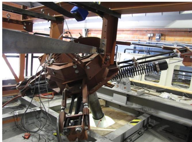
**Figure 8. Photo. Upper rig with spring rotation at 45 degrees.**
