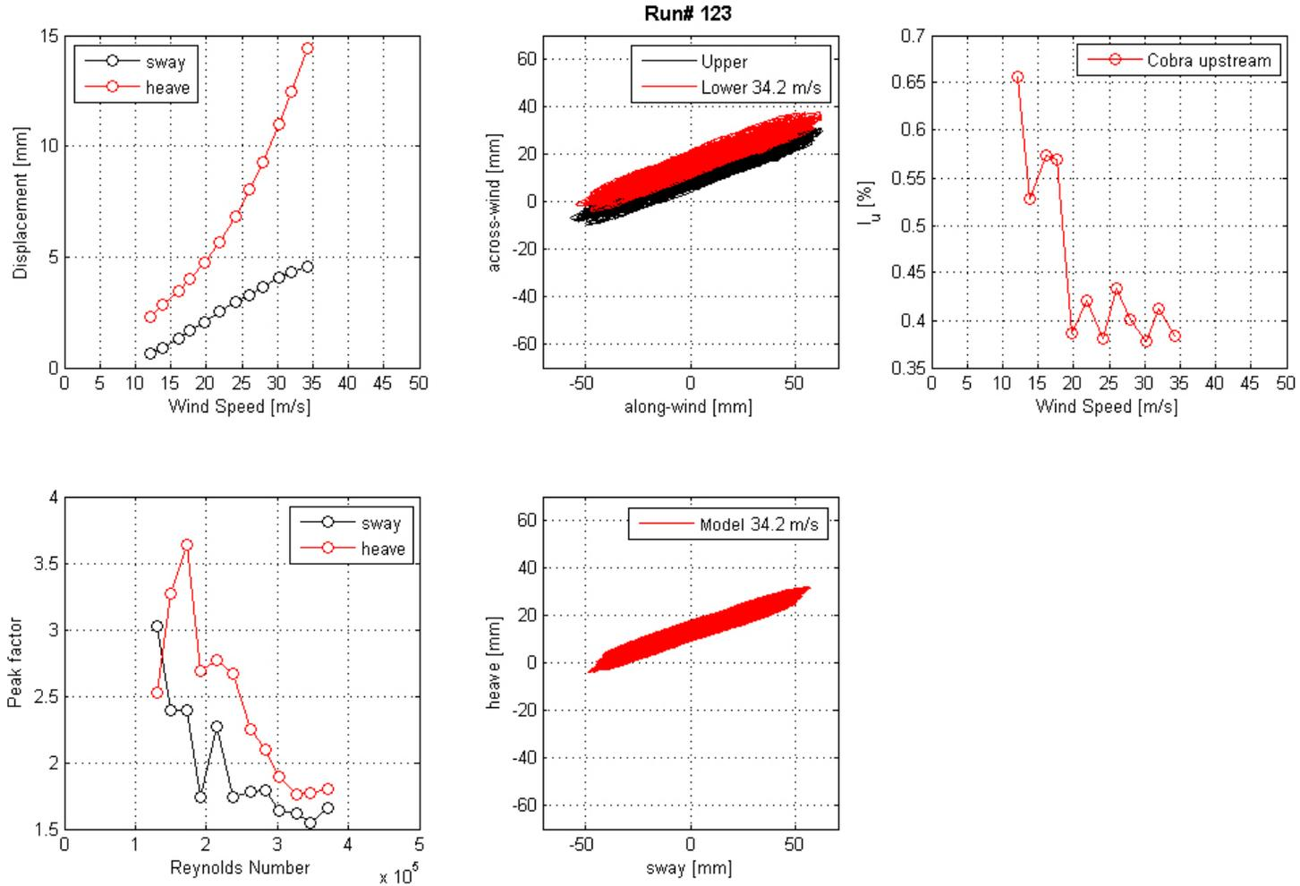
**Figure 109. Graph. Mean displacement and peak factor from the laser, motion path at one wind speed, and intensity of turbulence measured at the entrance of the test section for run 123.**
