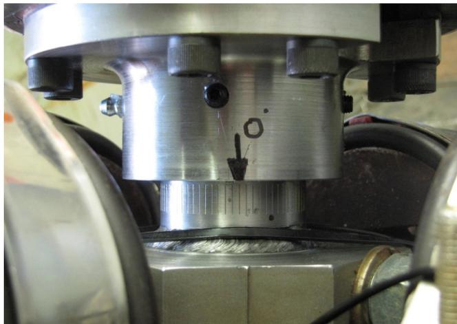
**Figure 11. Photo. Turntable that allowed rotation of the cable model on its axis.**
