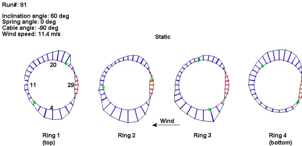
**Figure 46. Illustration. Distribution of surface pressure coefficient for the four rings with the cable in a static position (run 81).**
