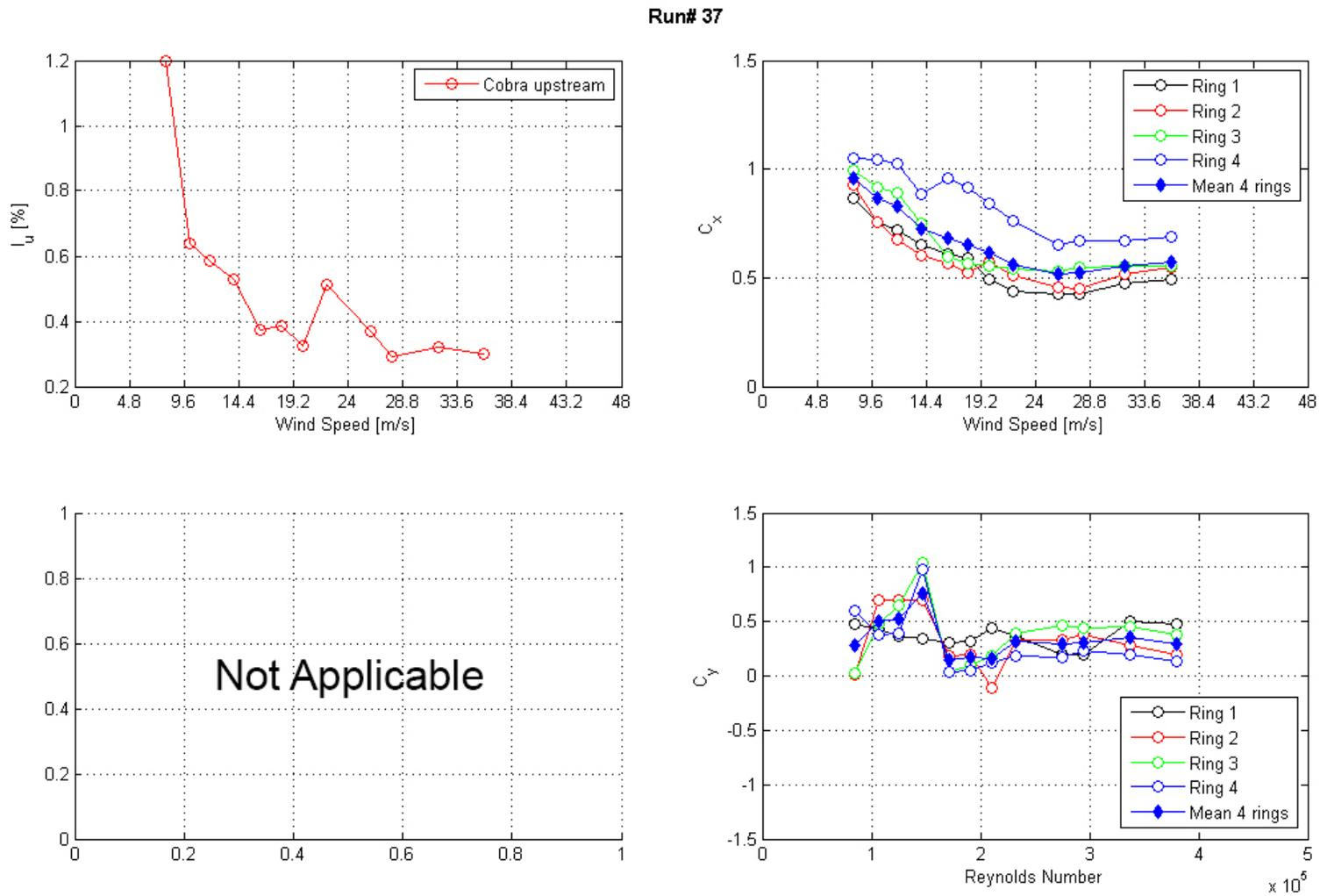
**Figure 65. Graph. Intensity of turbulence measured at the entrance of the test section and  $C_x$  and  $C_y$  calculated from surface pressure measurements as a function of Reynolds number and wind speed for run 37.**
