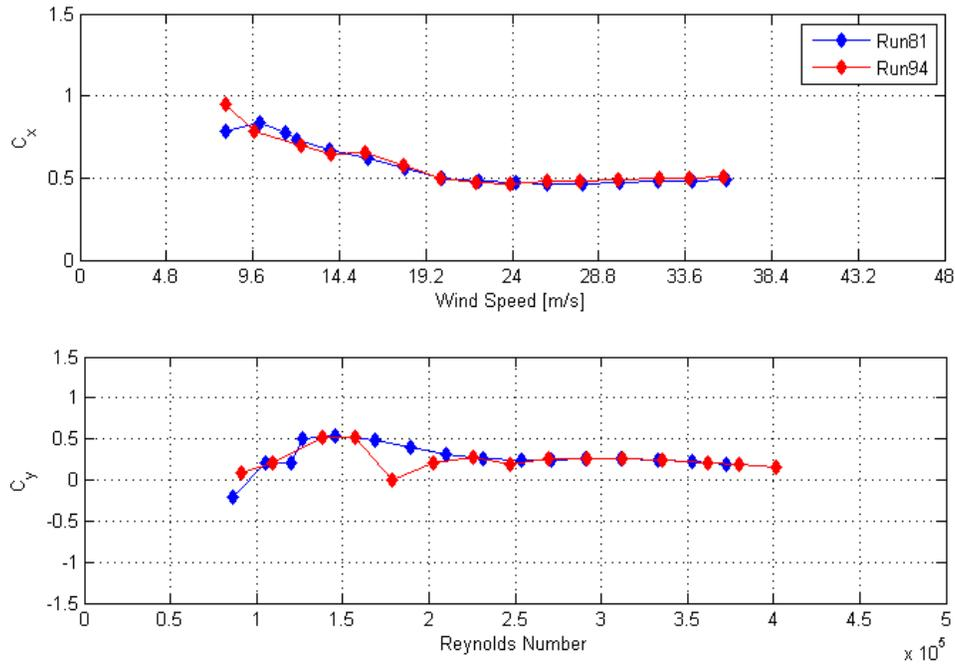
**Figure 56. Graph. Mean  $C_x$  and  $C_y$  calculated from the integration of surface pressure measurements for two runs with cable inclined at 60 degrees and rotated at -90 degrees in smooth flow and with helical fillet.**
