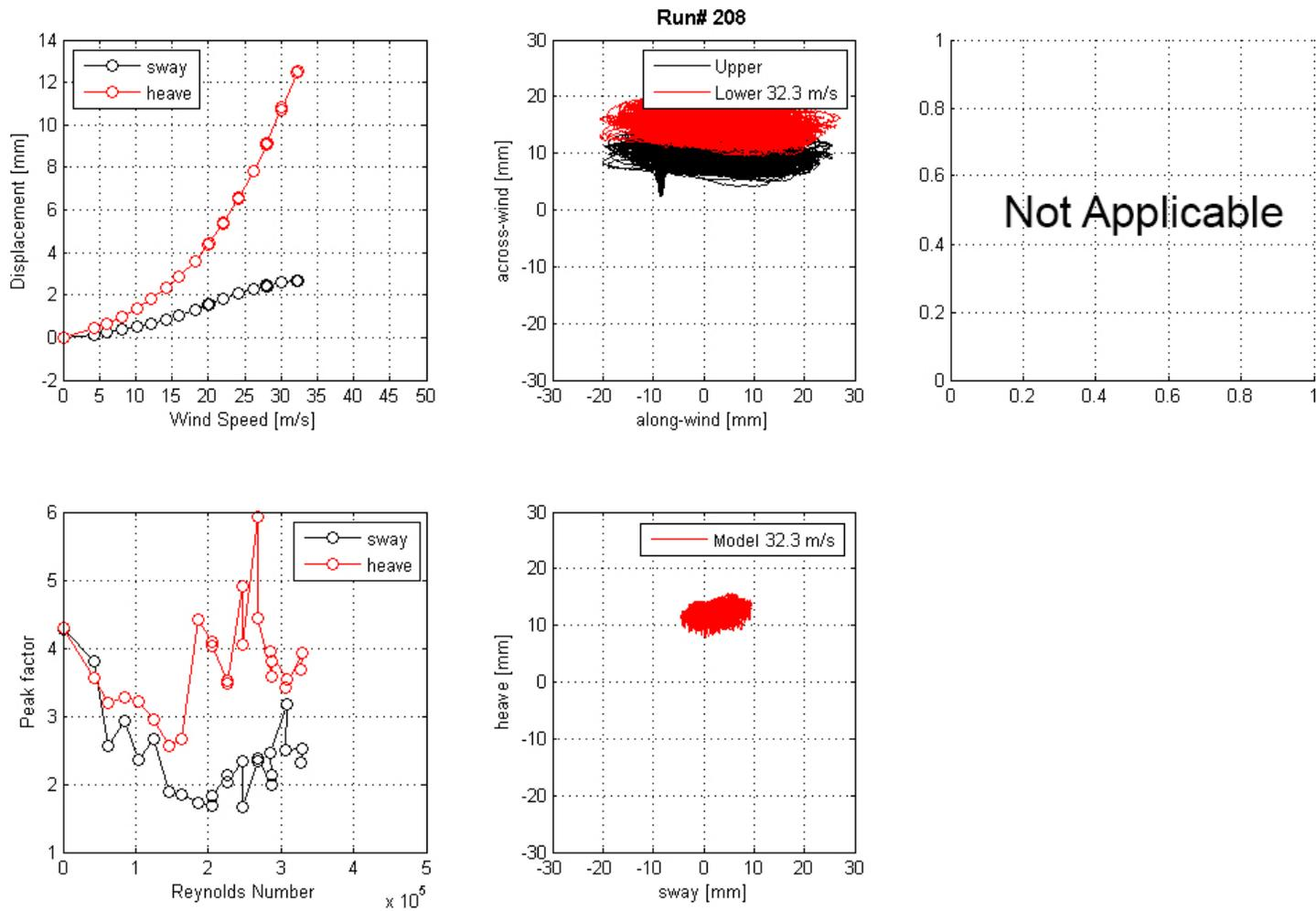
**Figure 149. Graph. Mean displacement and peak factor from the laser, motion path at one wind speed, and intensity of turbulence measured at the entrance of the test section for run 208.**
