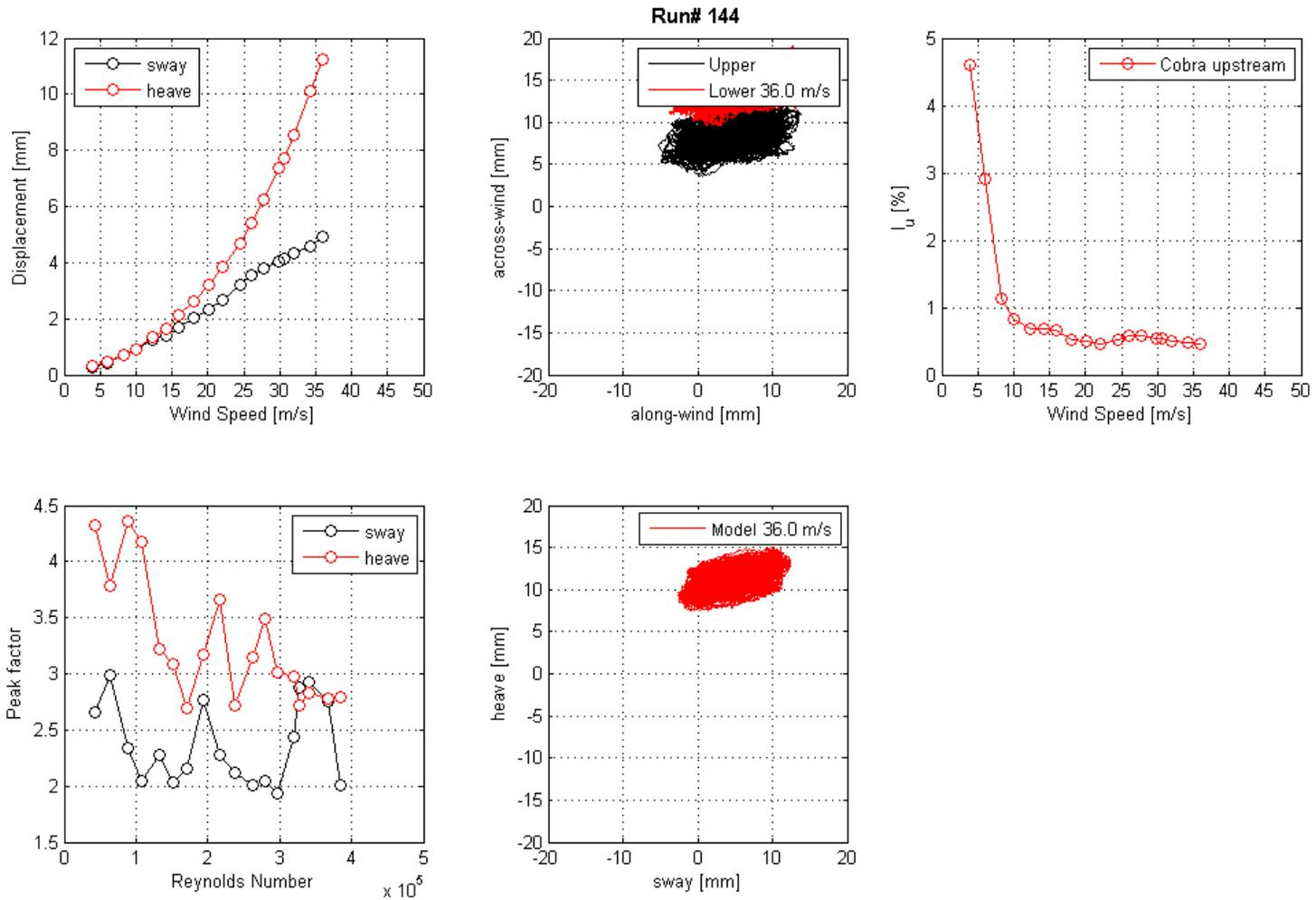
**Figure 123. Graph. Mean displacement and peak factor from the laser, motion path at one wind speed, and intensity of turbulence measured at the entrance of the test section for run 144.**
