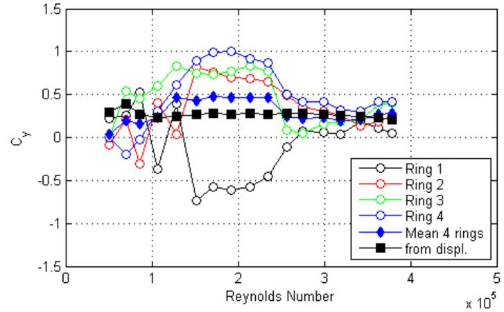
Figure 70. Graph. Response of the cable as a function of wind speed or Reynolds number as measured by the lasers, accelerometers, and surface pressures for run 46.
