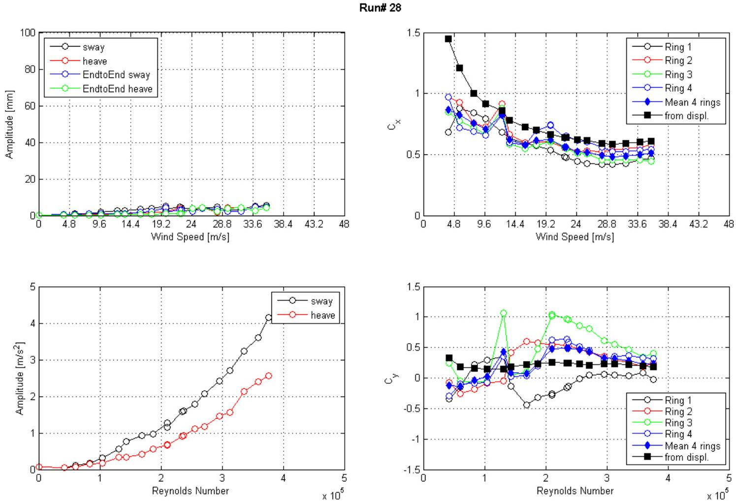
Figure 61. Graph. Response of the cable as a function of wind speed or Reynolds number as measured by the lasers, accelerometers, and surface pressures for run 28.
