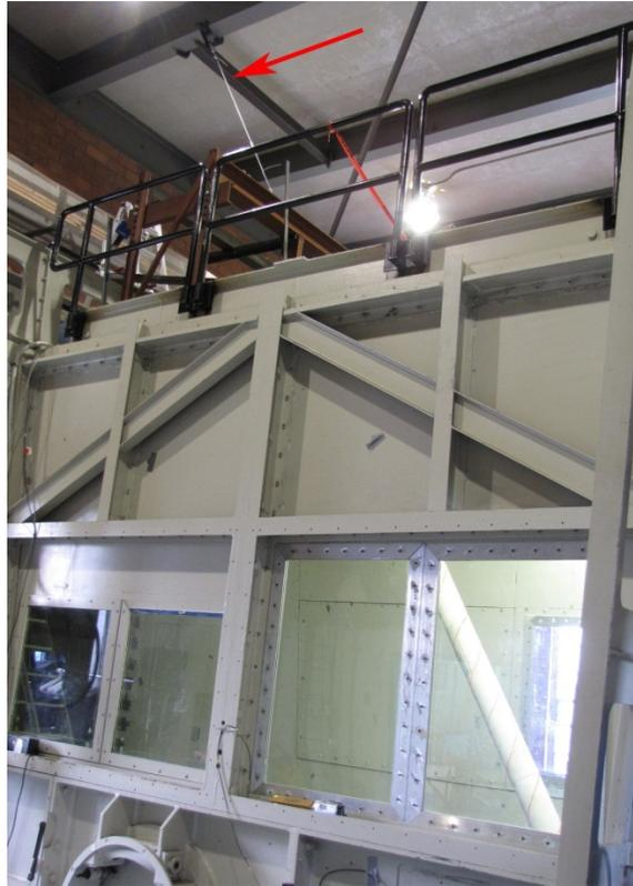
**Figure 9. Photo. Cable model at an inclination of 60 degrees from outside the test section of the 3-by-6-m Propulsion and Icing Wind Tunnel.**
