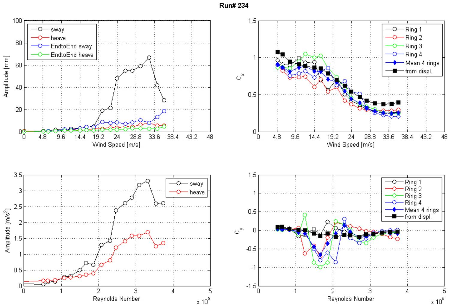
**Figure 166. Graph. Response of the cable as a function of wind speed or Reynolds number as measured by the lasers, accelerometers, and surface pressures for run 234.**
