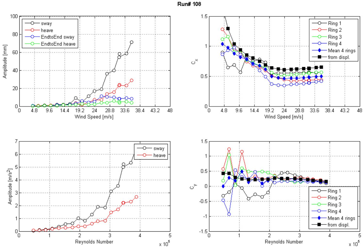
**Figure 102. Graph. Response of the cable as a function of wind speed or Reynolds number as measured by the lasers, accelerometers, and surface pressures for run 108.**
