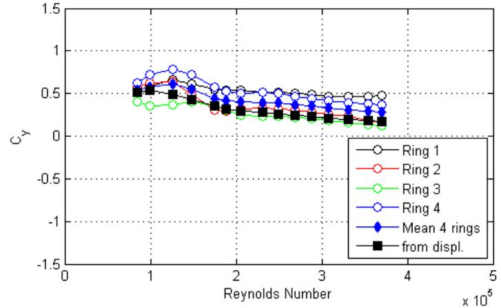
Figure 114. Graph. Response of the cable as a function of wind speed or Reynolds number as measured by the lasers, accelerometers, and surface pressures for run 136.
