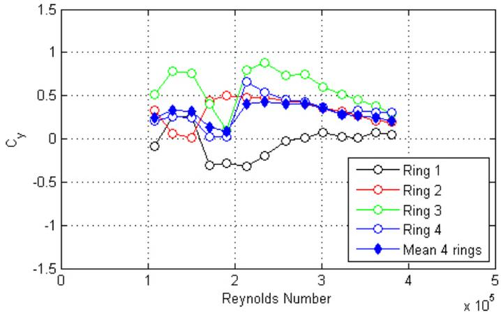
Figure 63. Graph. Intensity of turbulence measured at the entrance of the test section and  $C_x$  and  $C_y$  calculated from surface pressure measurements as a function of Reynolds number and wind speed for run 32.
