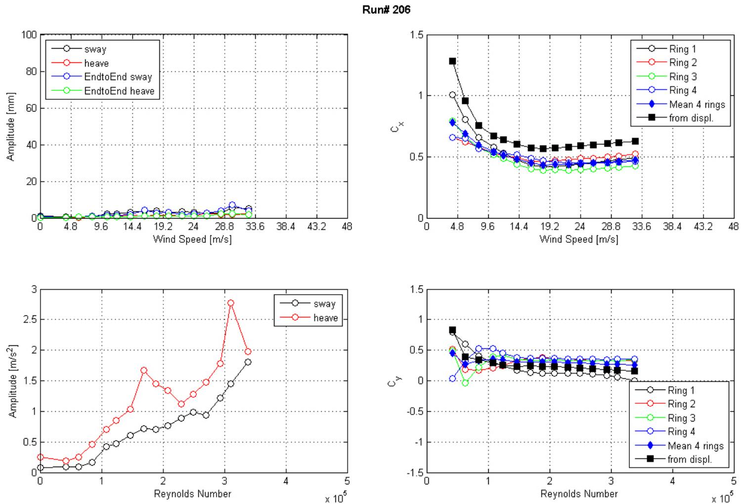
**Figure 146. Graph. Response of the cable as a function of wind speed or Reynolds number as measured by the lasers, accelerometers, and surface pressures for run 206.**
