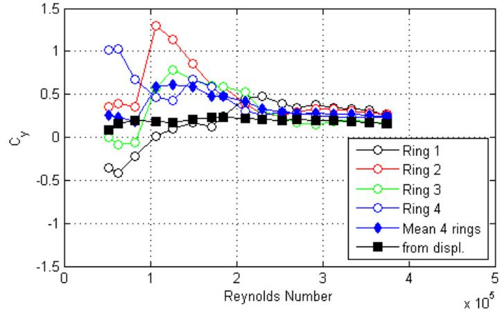
Figure 112. Graph. Response of the cable as a function of wind speed or Reynolds number as measured by the lasers, accelerometers, and surface pressures for run 131.
