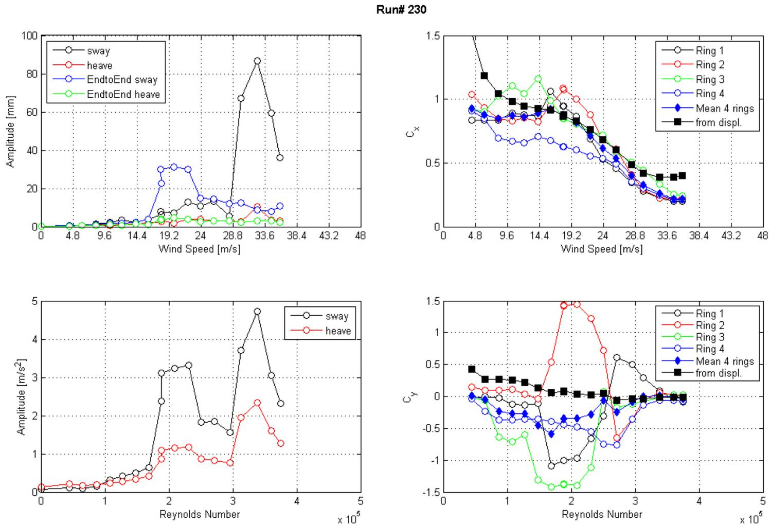
**Figure 164. Graph. Response of the cable as a function of wind speed or Reynolds number as measured by the lasers, accelerometers, and surface pressures for run 230.**
