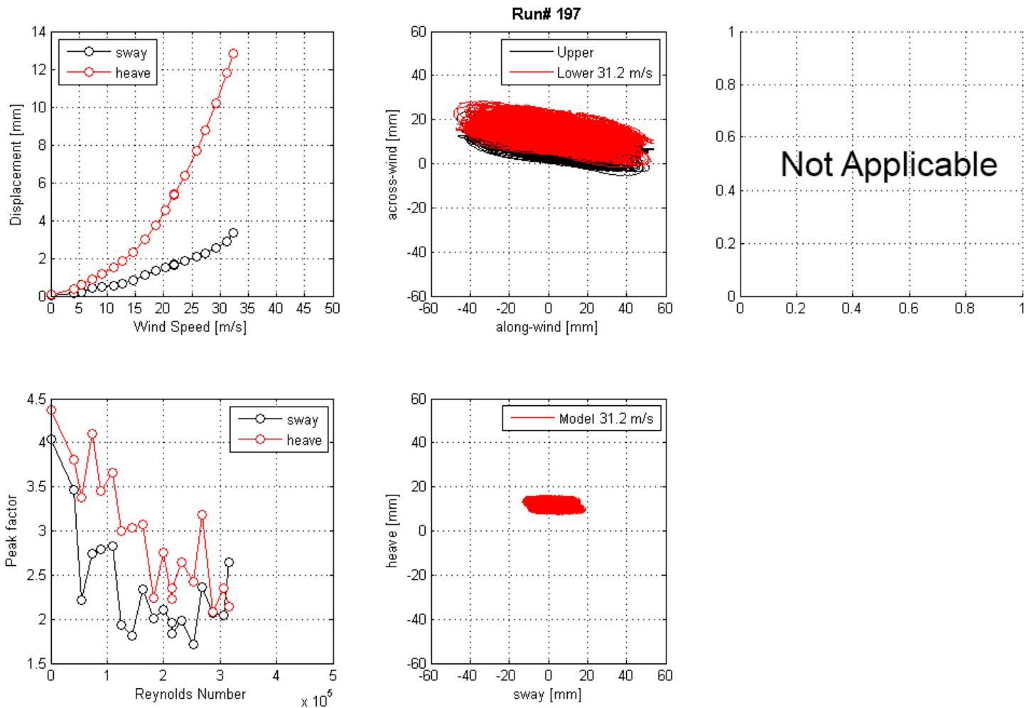
**Figure 141. Graph. Mean displacement and peak factor from the laser, motion path at one wind speed, and intensity of turbulence measured at the entrance of the test section for run 197.**
