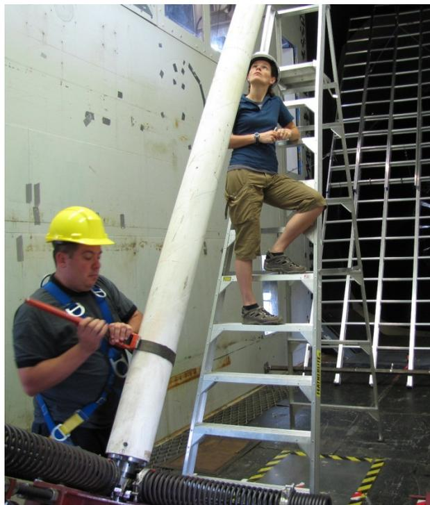
**Figure 28. Photo. Procedures followed to set the azimuth angle of the cable model.**
