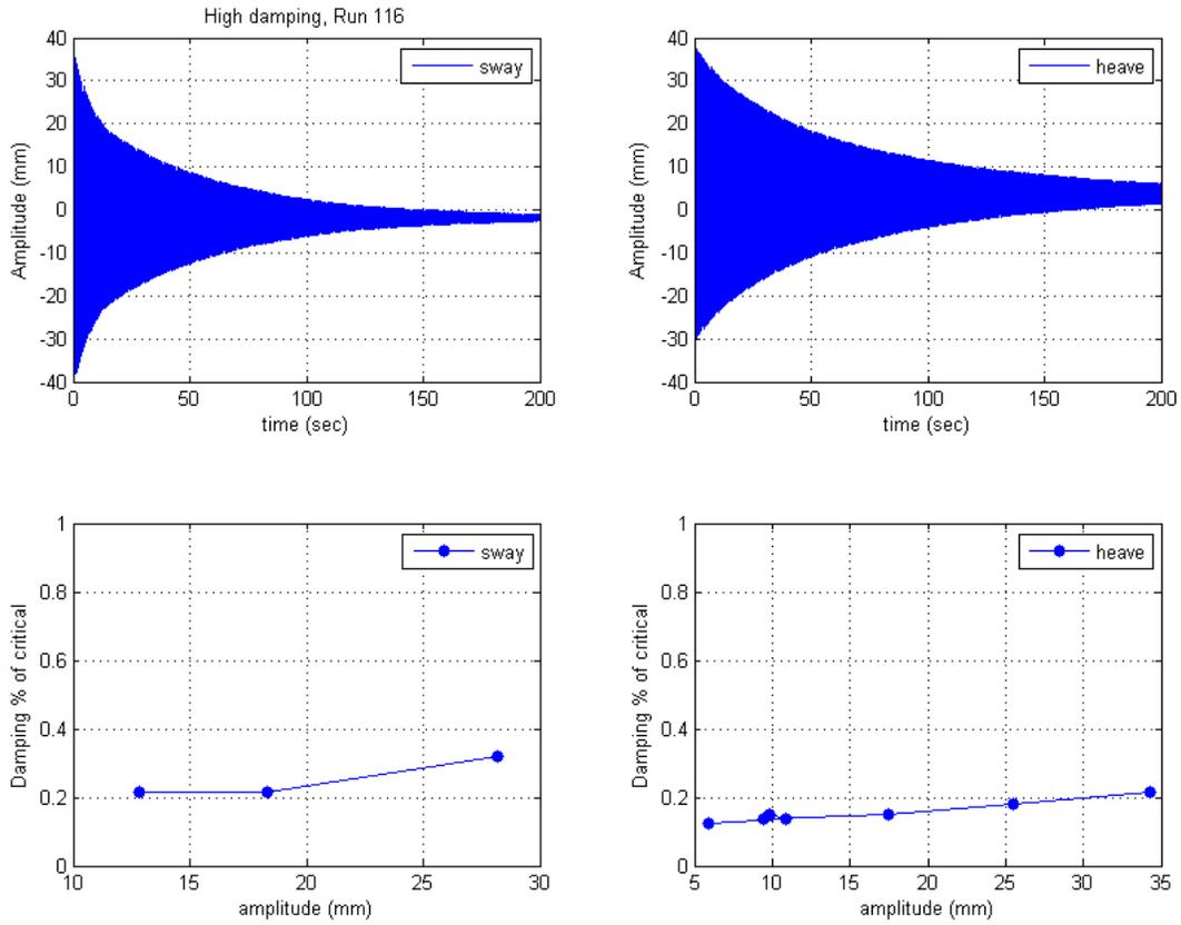
**Figure 186. Graph. Damping traces and level for the sway and heave modes for the high damping level case.**
