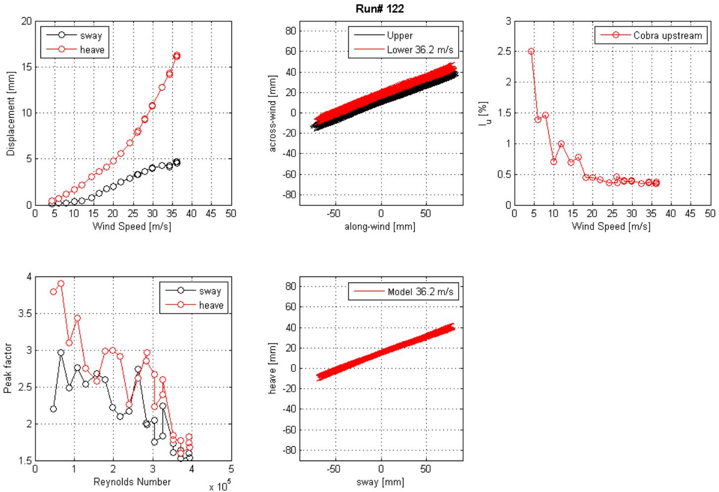
**Figure 107. Graph. Mean displacement and peak factor from the laser, motion path at one wind speed, and intensity of turbulence measured at the entrance of the test section for run 122.**
