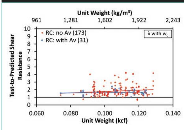
Figure 4. Test-to-predicted shear resistance compared with unit weight for GP-equation method.
