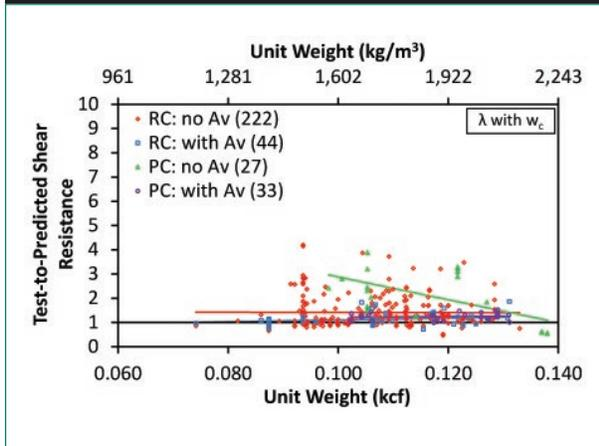
Figure 6. Test-to-predicted shear resistance compared with unit weight for Simplified Procedure for RC and PC Sections.
